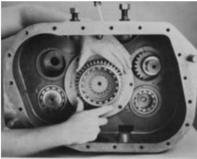
32. Center rear of mainshaft in case bore and install the auxiliary drive gear assembly on shaft, partially seating the bearing in bore. **DO NOT COMPLETE INSTALLATION AT THIS TIME.**
