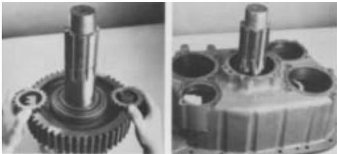
7. Place two mainshaft spacers or flat steel stock of equivalent thickness (.190") on rear face of deep reduction gear, 180° from each other (left). Install the auxiliary housing over end of output shaft assembly, allowing the housing to rest on blocking (right).
