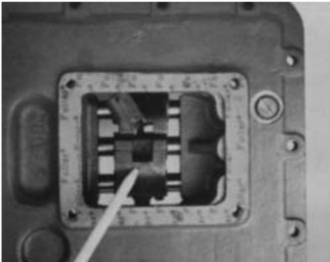
1. Check the shift bar housing assembly to make sure shift block and yoke notches are aligned in the neutral position.
