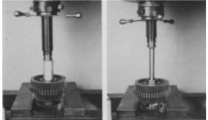
3. Using the rear face of 4th speed gear as a base, press the drive gear, PTO gear and 4th speed (or overdrive) gear from each countershaft (left). This will also remove the front bearing inner race from countershaft of models so equipped (right).
