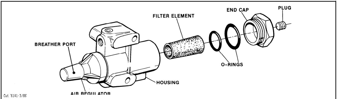
The air filter contains a replaceable filter element which can be removed by turning out the end cap. This element should be cleaned at each oil change, or more often under high humidity conditions. Replace if necessary.
