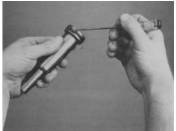
2. If previously removed, install the O-ring in groove of yoke bar piston.
