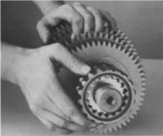
28. Remove the mainshaft assembly from vise. Align the missing internal spline of 4th-5th speed sliding clutch with key in mainshaft and install on front of shaft, engaging the external splines of sliding clutch with clutching teeth of 4th speed (or Overdrive) gear.
