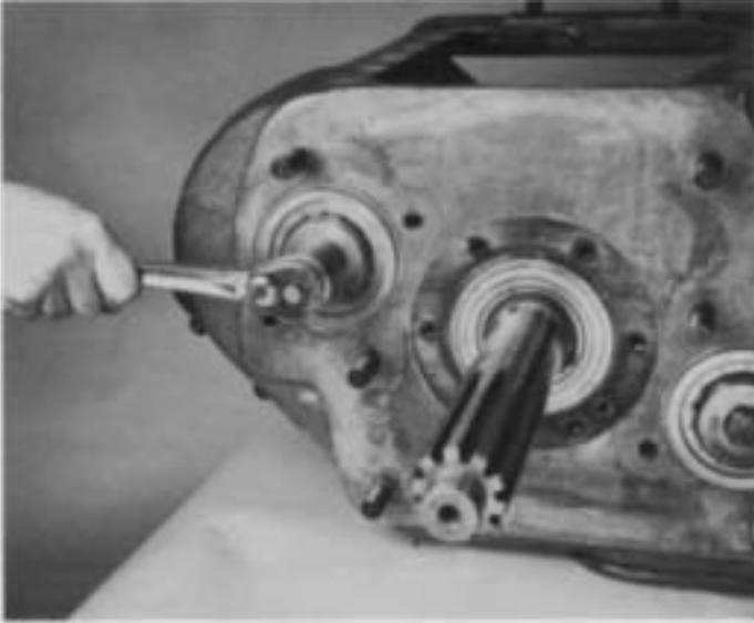
3. Turn out the capscrew and remove the front bearing retainer plate from each countershaft.
