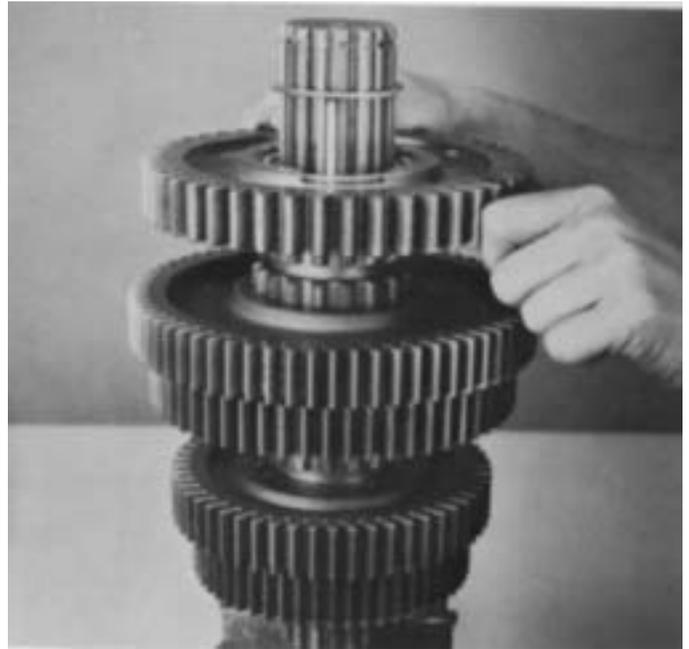
26. With the proper reverse gear limit washer installed on mainshaft, remove the auxiliary drive gear assembly and reverse gear.
