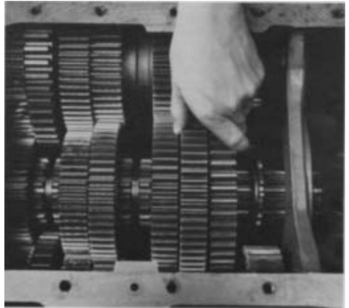
2. Move the reverse gear forward and against the 1st speed gear, engaging the splines of mainshaft sliding clutch.
