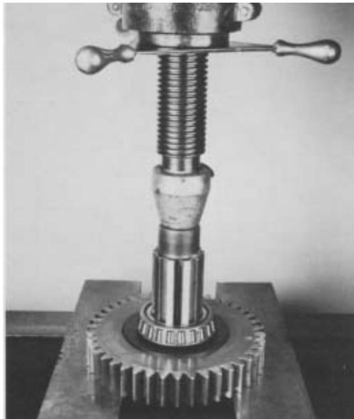
3. Using the front face of low range gear as a base, press the output shaft through the gear and bearing. Remove the bearing and washer from hub of low range gear.
