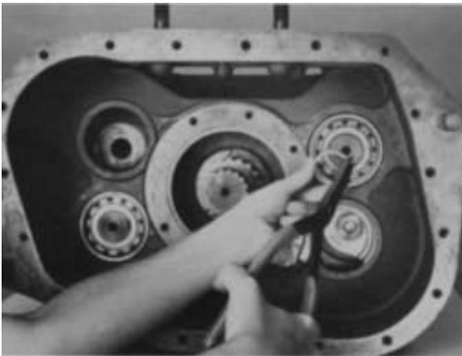
1. Remove the snap ring from groove at rear of each countershaft.
