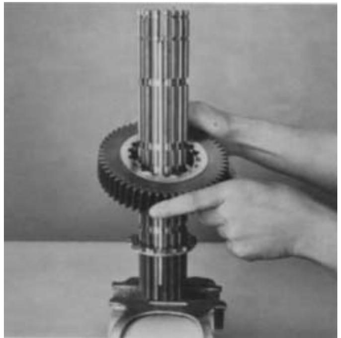
5. Install the 4th speed (or Overdrive) gear on mainshaft, clutching teeth down and engaged with external splines of spacer.
