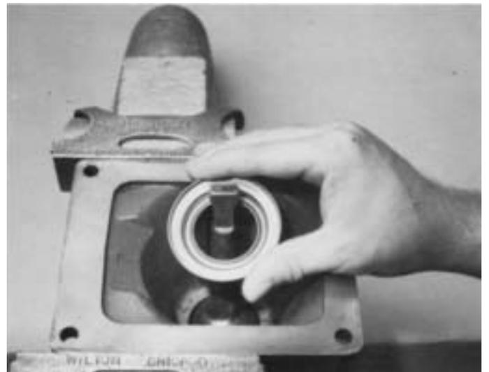
2. Position the gear shift lever in housing with spade pin in lever ball slot and install the tension spring washer over ball, dished-side up.
