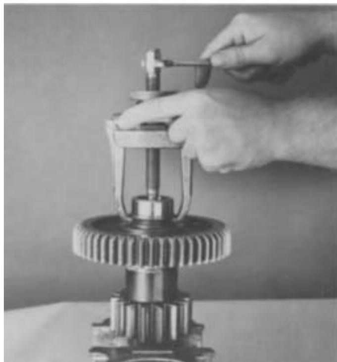
5. If necessary, secure the assembly in a vise and remove the bearing inner race from front of countershaft with jaw pullers.
