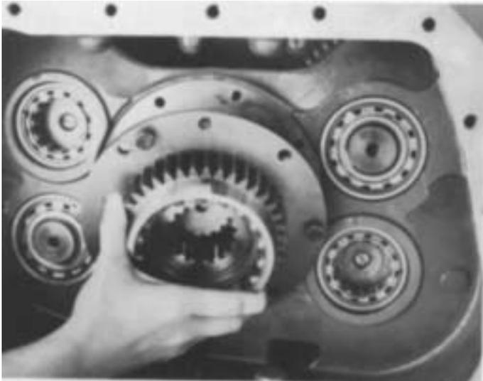
1. Remove the auxiliary drive gear assembly from mainshaft and rear bearing bore. Do not allow mainshaft to move to rear when removing auxiliary drive gear.
