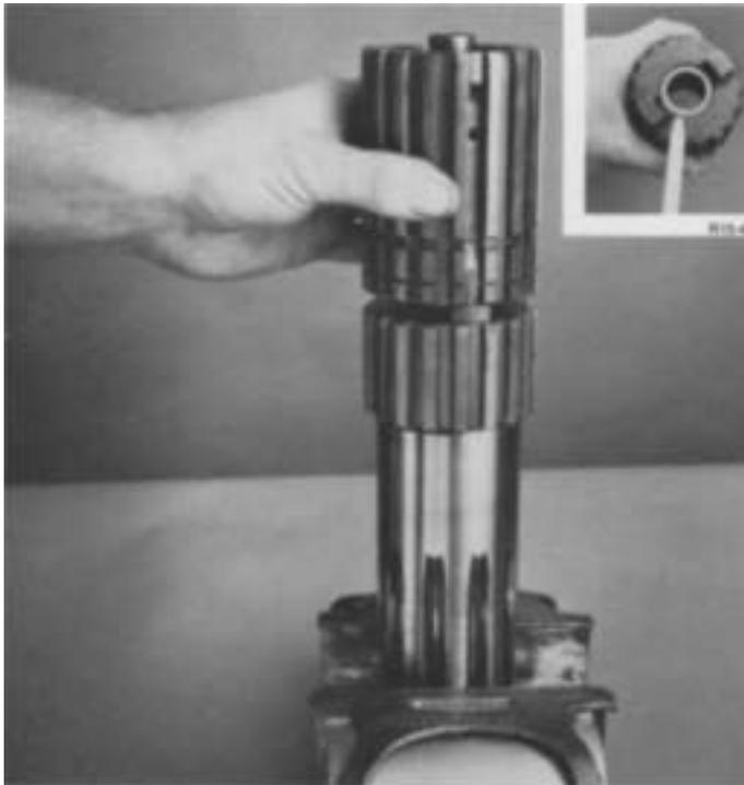
2. If necessary, press the bushing in rear bore of range mainshaft (inset) and install the mainshaft in position on quill.
