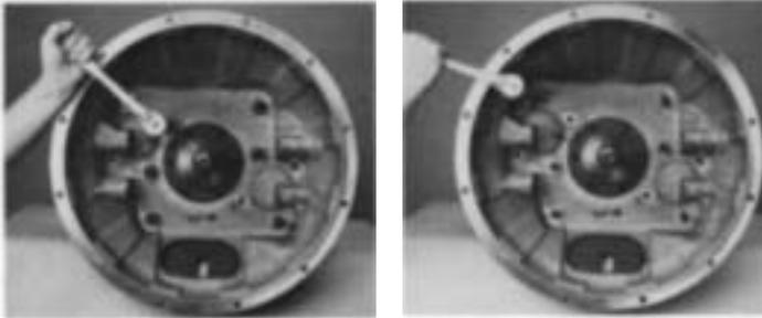
2. Turn out the four capscrews and remove the six nuts and lockwashers from studs securing the clutch housing to transmission case.
