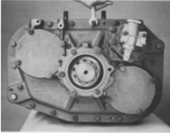
1. Turn out the retaining capscrews in auxiliary housing flange.
