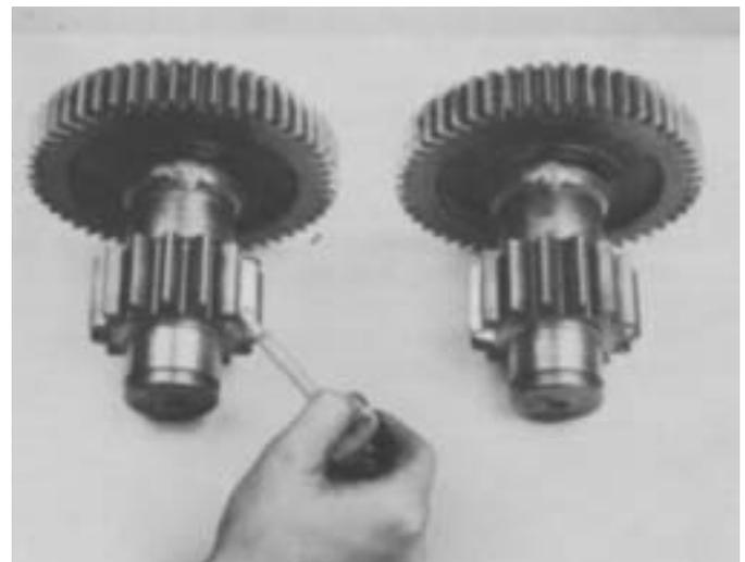
2. **IMPORTANT:** On the low range gear of each auxiliary countershaft assembly, use a highly visible color of toolmaker's dye to mark the tooth stamped with an "O" for timing purposes.
