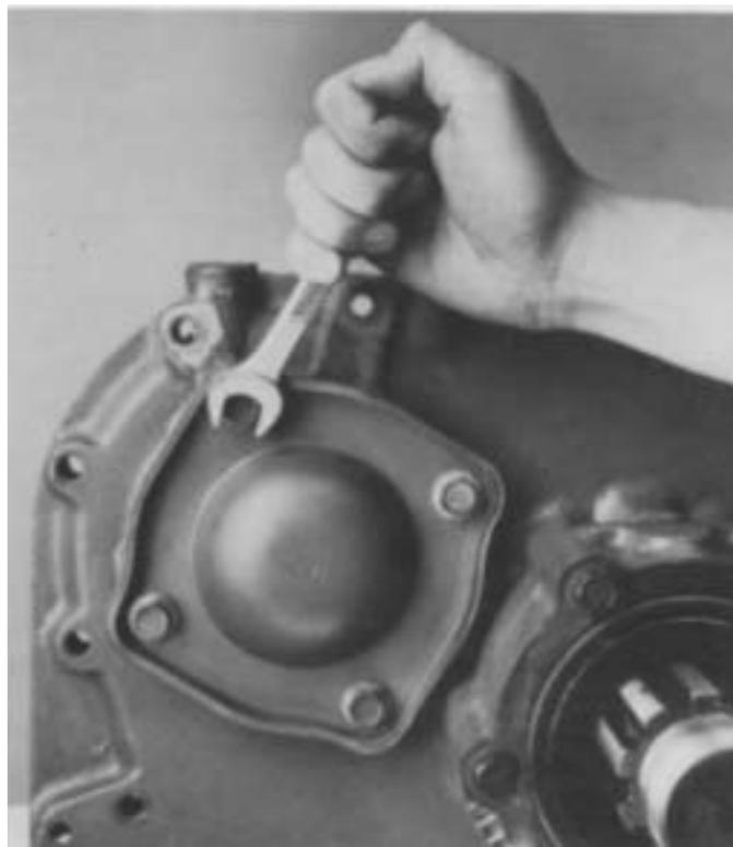
5. Position the corresponding new gasket on cover mounting surface and install both rear bearing covers. Tighten cap screws to secure covers to auxiliary plate.
