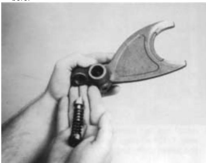
8. If necessary, remove the plug, spring, and reverse-stop plunger from the LO-Reverse speed shift yoke bore.
