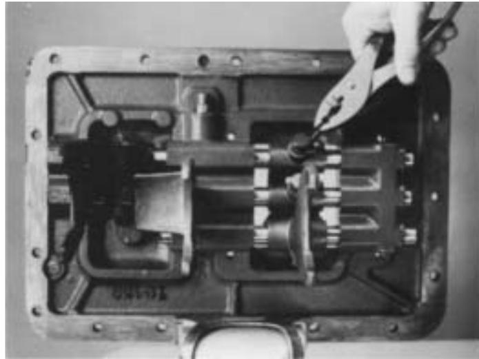
9. While holding notched-end of the bar, install the 3rd-4th speed shift bar in the housing boss upper bore, position the shift block on the bar between the front and center bosses, long hub to the housing rear. Install the block and yoke lockscrews, tighten, and lockwire securely.
