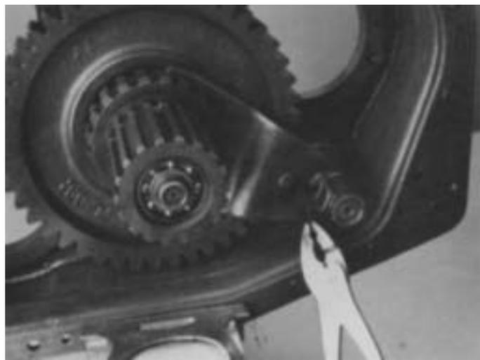
4. Install the yoke lockscrew, tighten and wire securely.
