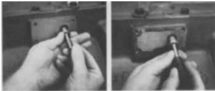
2. Install the spring on shank of actuating pin and insert in bore of transmission case.
