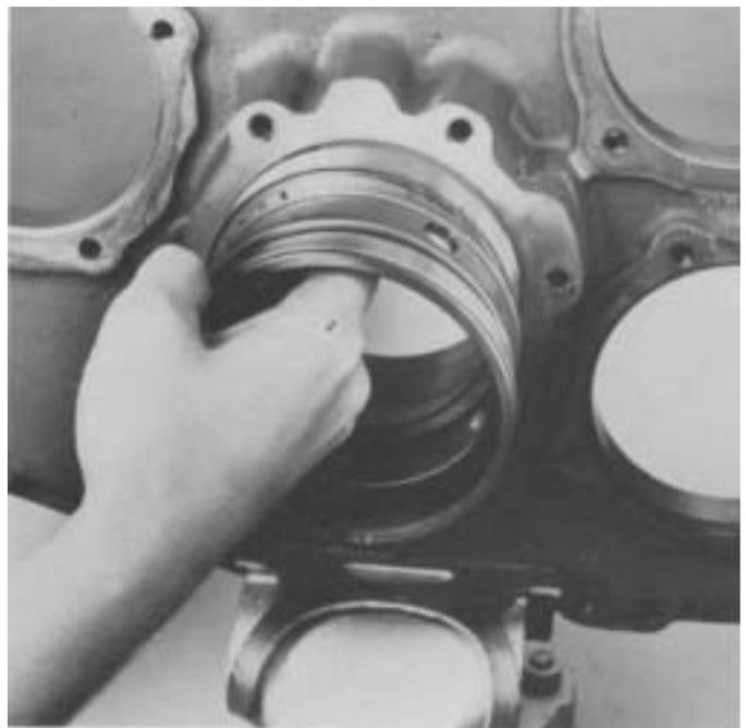
6. Remove the two bearing cups and outer spacer from bore in auxiliary housing.
