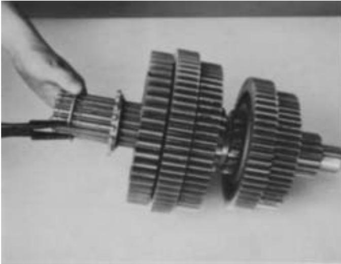
3. Remove the snap ring from groove at rear of mainshaft.
