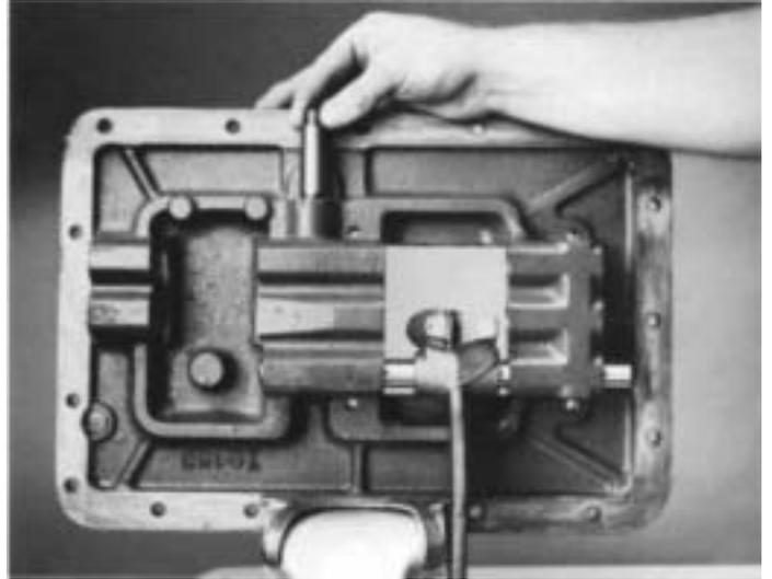
5. While holding the plunger shank, install the actuating plunger in the center boss bore.
