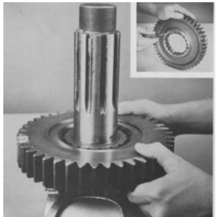
4. If previously removed, install the snap ring in deep reduction gear of models so equipped (inset). Install the gear on output shaft, clutching teeth down and engaged with splines of spacer.
