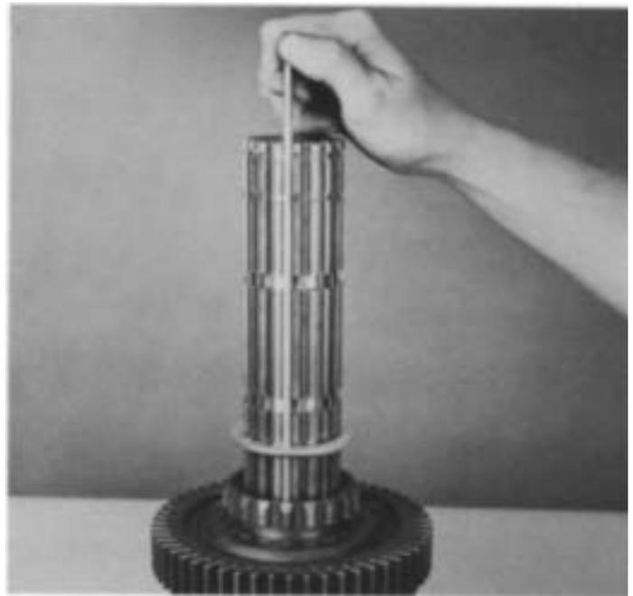
11. Remove the key from keyway and install the 2nd speed gear limit washer on mainshaft, flat side of washer up. Rotate washer in the 3rd groove of mainshaft to align the splines of washer with those of the mainshaft and reinsert key in keyway to lock washer in place.
