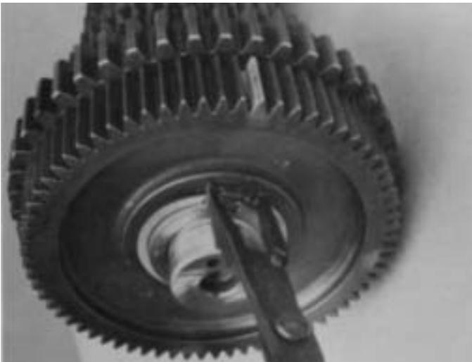
3. Remove the drive gear retaining snap ring from front of each countershaft.
