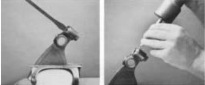
3. Install the plug and tighten to compress the spring (left). Back the plug out 1 - 1 1/2 turns and stake the plug through the small hole in the yoke (right.)
