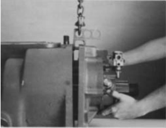
1. Attach a chain hoist to auxiliary. Move the assembly evenly into rear of front case, piloting it on the dowel pins. As assembly is moved forward, the countershaft drive gears will mesh with the auxiliary drive gear.
