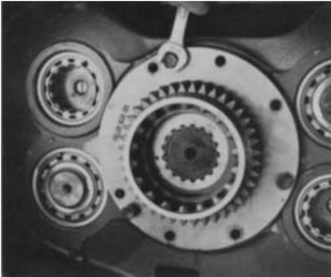
3. Insert three puller screws in the specially tapped holes of retainer ring. Tighten screws evenly to pull the auxiliary drive gear assembly from case bore.
