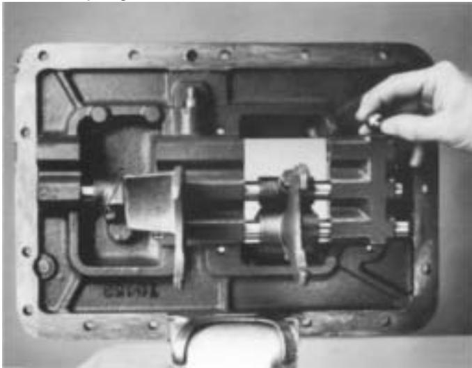
8. Install the other 3/4" interlock ball in the rear boss top bore. This ball rides between the 1st-2nd and the 3rd-4th speed shift bars.
