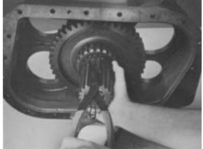
15. Install snap ring in groove of range mainshaft.
