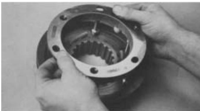
2. Place the larger low range synchronizer ring on bench and pull the high range synchronizer from blocker pins. However, before doing so, cover the assembly with a shop rag to prevent losing the three springs released from high range synchronizer at pin locations.
