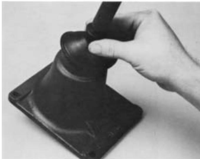
4. Remove the assembly from vise and install the rubber boot over gear shift lever and against housing.
