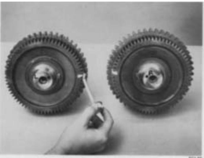
**IMPORTANT:** Mark the countershaft drive gear for timing purposes. On the drive gear of each countershaft assembly, mark the tooth aligned with keyway of gear and stamped with an "O" for easy identification. A highly visible color of toolmakers' dye is recommended for making timing marks.
