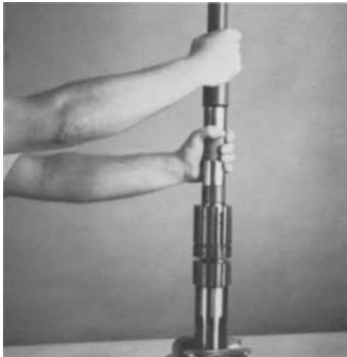
3. Install the bearings in front bore of range mainshaft. Use a small flanged-end driver to properly seat bearing in bore on mainshaft quill.
