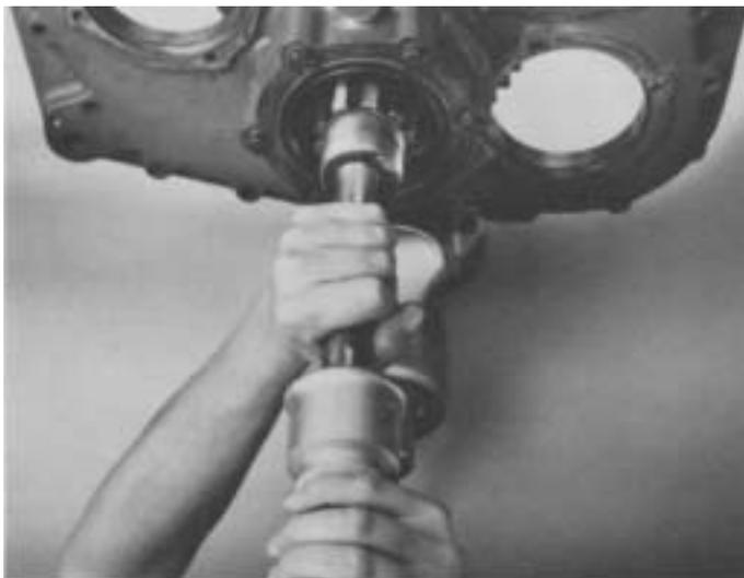
1. Use a soft bar and maul to drive the output shaft forward and through rear bearing assembly.
