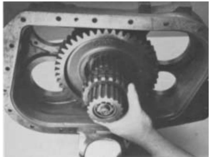
2. Remove deep reduction sliding clutch.
