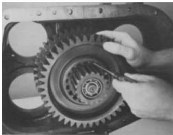
2. Turn the washer located in the hub of low range gear so that the splines of washer align with the splines of mainshaft.
