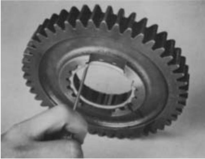
22. Install the snap ring in hub of reverse gear ONLY TO CHECK AXIAL CLEARANCE (END-PLAY) LIMITS.
