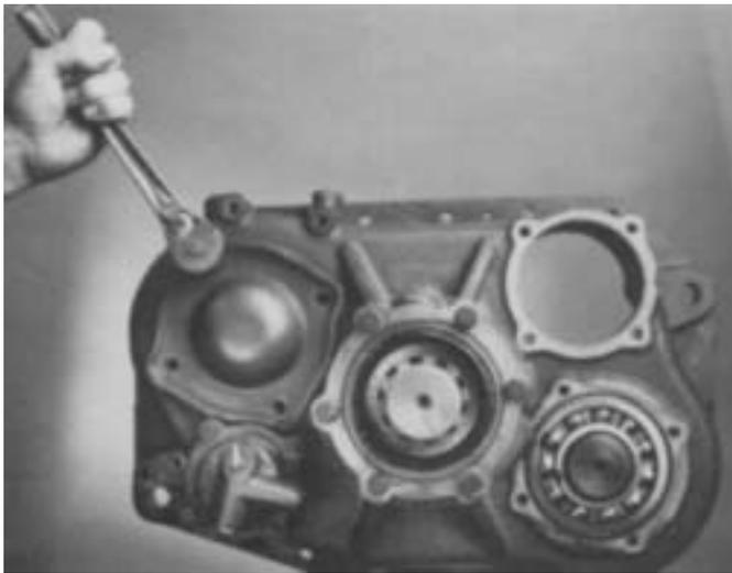
1. Turn out the capscrews and remove both countershaft rear bearing covers.
