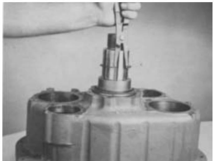
2. If not previously done so, remove the snap ring and speedometer drive gear or replacement spacer from output shaft of models so equipped.
