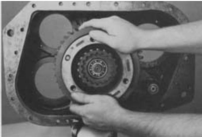
1. Pull the synchronizer assembly from the splines of range mainshaft.
