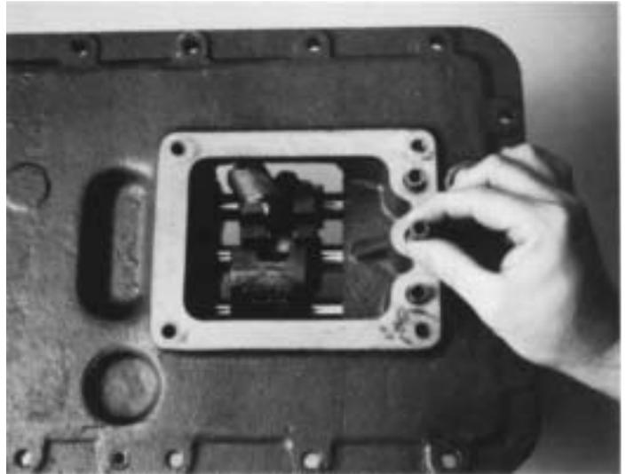
**12.** Install the three tension springs, one over each ball in the housing bores.
