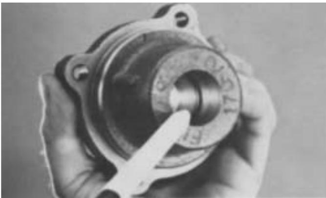
5. Remove the deep reduction cylinder housing and gasket from auxiliary housing. If necessary, remove the small O-ring from bore in cylinder housing.
