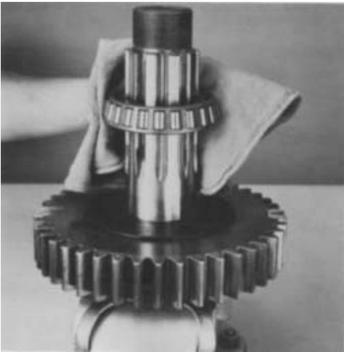
6. Heat the front bearing cone and install on shaft against washer, bearing taper up.
