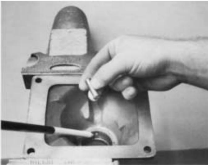
4. Remove the spade pin from bore in housing tower. If necessary, remove the O-ring from groove inside tower.
