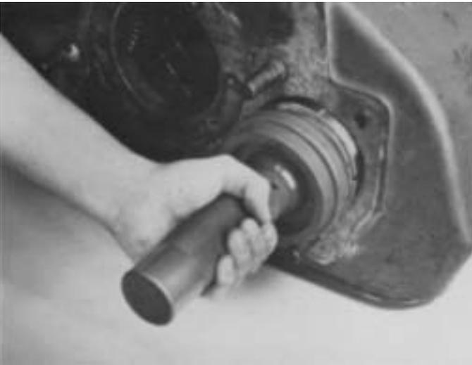
2. Use a flanged-end bearing driver to start the bearing in case bore.
