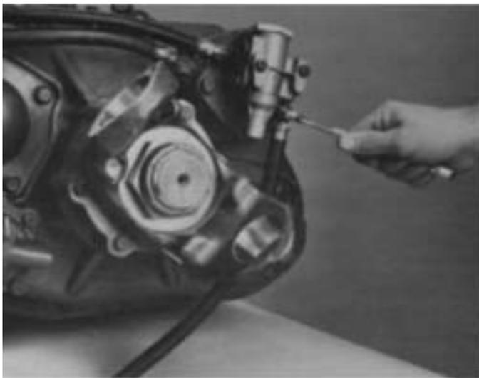
2. For 15-Speed Models ONLY, also disconnect the 1/4" I.D. air line between the air filter/regulator assembly and reduction cylinder.
