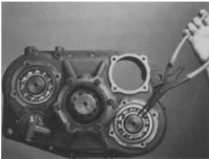
4. Install the snap ring in groove at rear of each countershaft.
