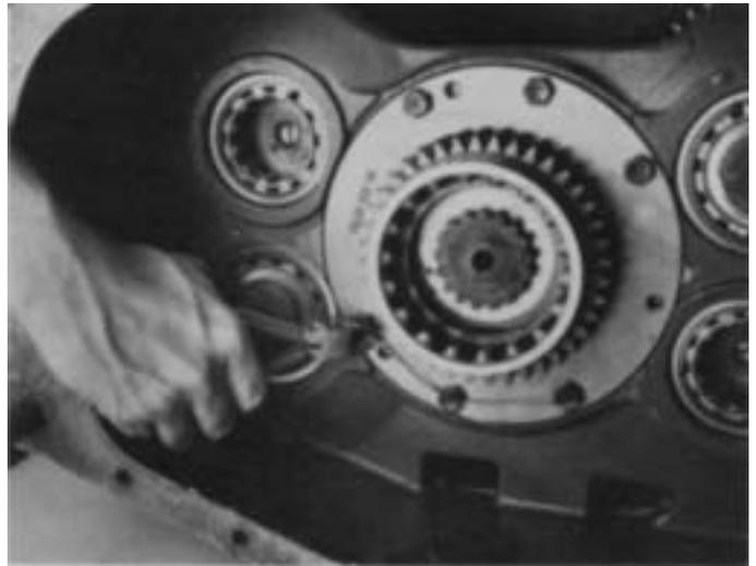
2. Cut lockwire and remove the cap screws from bearing retainer ring.
