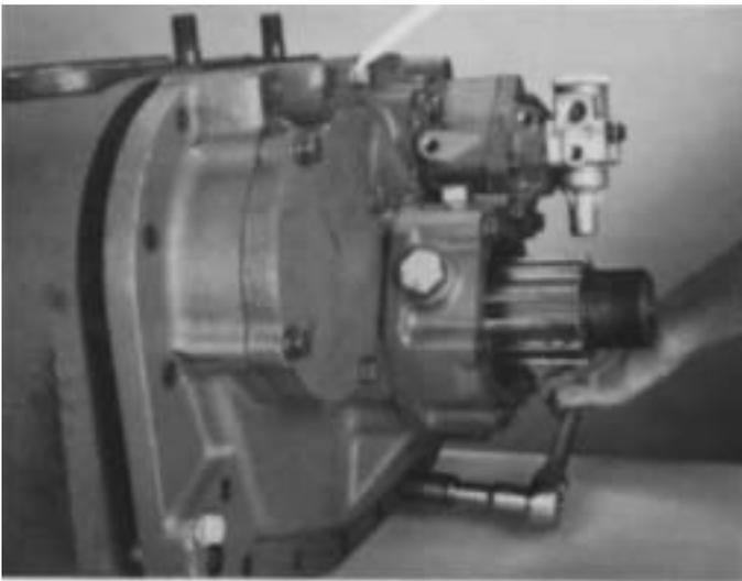
2. Insert three puller screws in the tapped holes of housing flange. Tighten evenly to move auxiliary section to the rear and just far enough from front section to break gasket seal.
