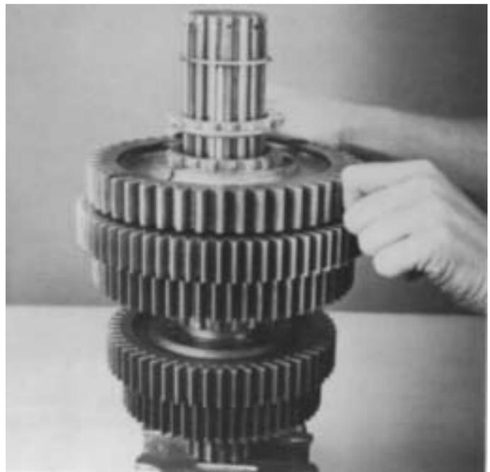
27. Remove the snap ring from hub of reverse gear and reinstall the gear on mainshaft. Engage the clutching teeth of gear with the splines of spacer and sliding clutch and move the reverse gear against the 1st speed gear.
