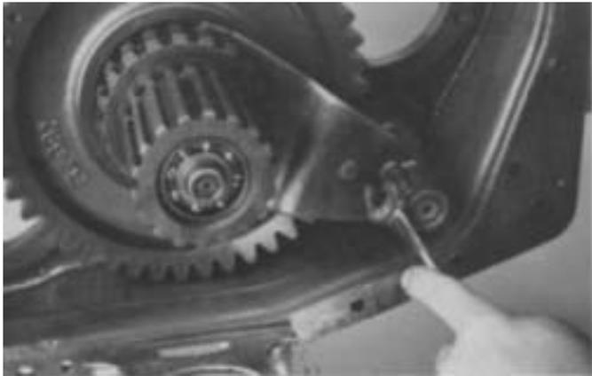
3. Cut lockwire and remove the lockscrew from shift yoke.
