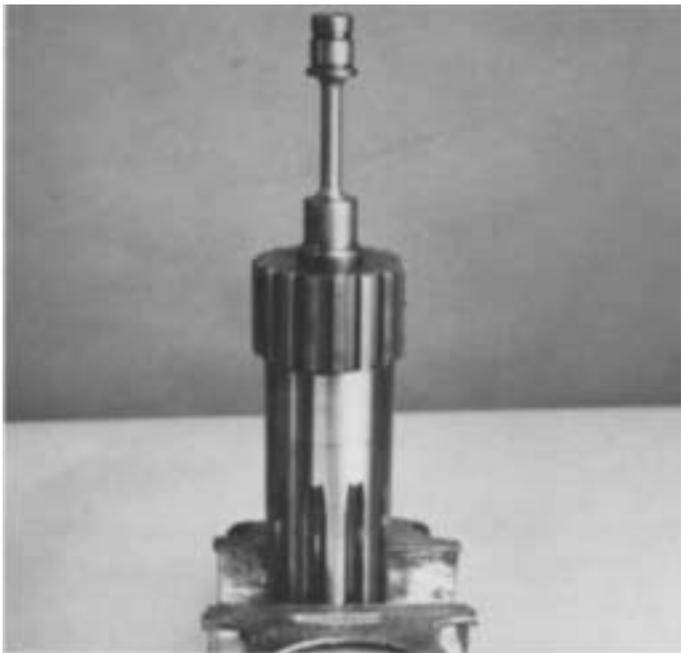
1. Secure the output shaft in a vise with mainshaft quill up.
