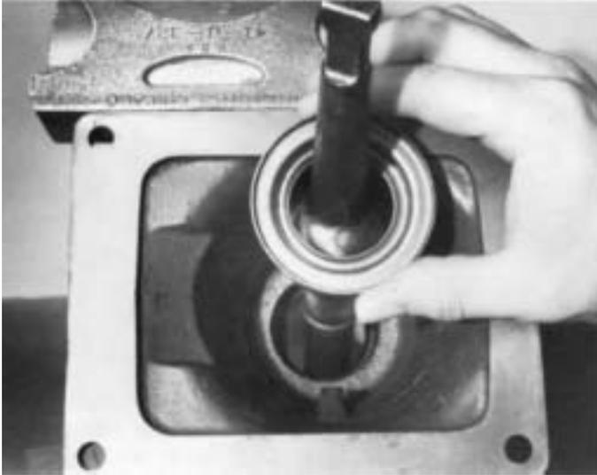
3. Remove the tension spring, washer and gear shift lever from housing.
