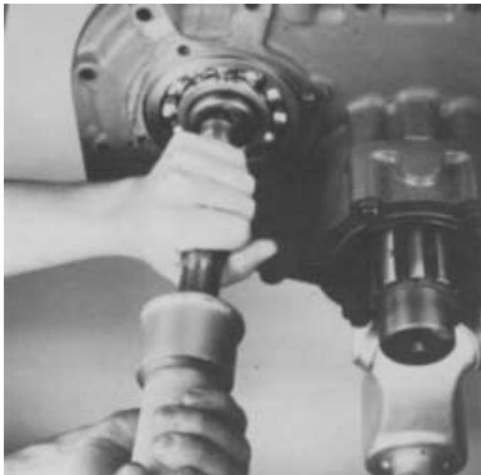
3. Use a soft bar and maul to drive the countershafts forward and from rear bearings.
