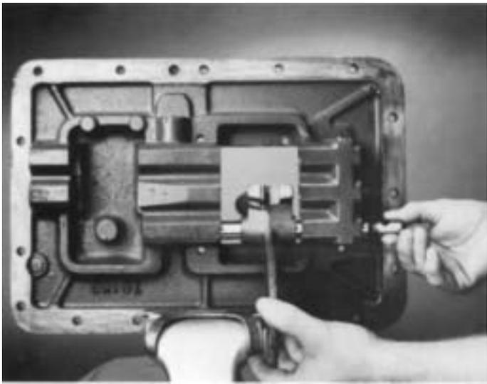
4. Secure the shift bar housing in a vise. Hold the notched-end of the short LO-Reverse speed shift bar, install the bar in the lower bore of the shift bar housing bosses. Install the yoke lock screw, tighten and wire securely.
