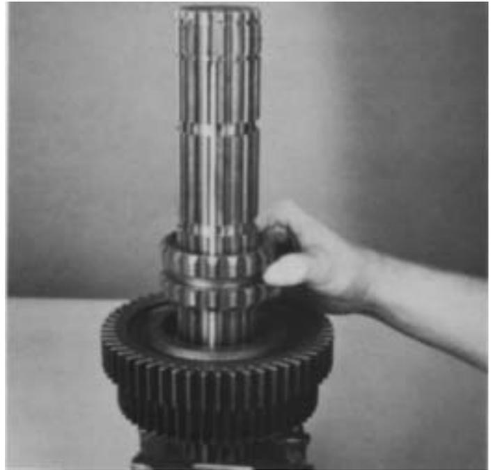
10. Install the 2nd-3rd speed sliding clutch, aligning the missing internal spline of sliding clutch with key in mainshaft.
