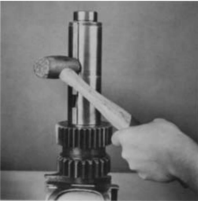
1. If previously removed, install the roll pin and key in keyway of countershaft.
