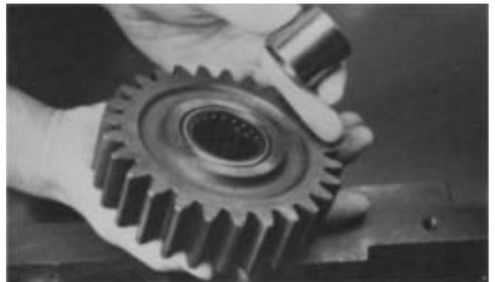
7. If necessary, remove the inner race from bearing and press needle bearing from idler gear.
