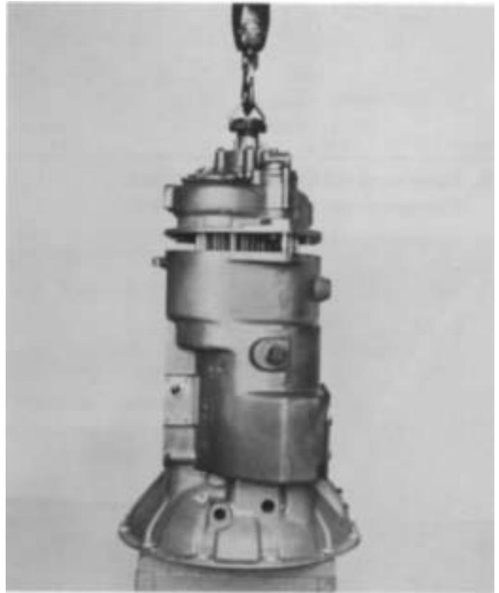
3. The auxiliary section can also be installed with transmission set in the vertical position. Block under the clutch housing to prevent damage to the input shaft, position the corresponding new gasket on plate/housing mounting surface and lower the assembly onto rear of front case. Install the retaining capscrews and tighten securely. See **TORQUE RECOMMENDATIONS**,
