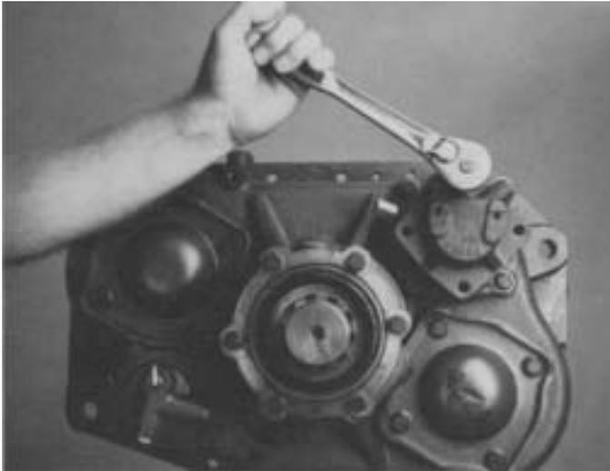
1. For ease of disassembly, mount the auxiliary section upright in a vise. Turn out the cap screws and remove the range cylinder cover and gasket.
