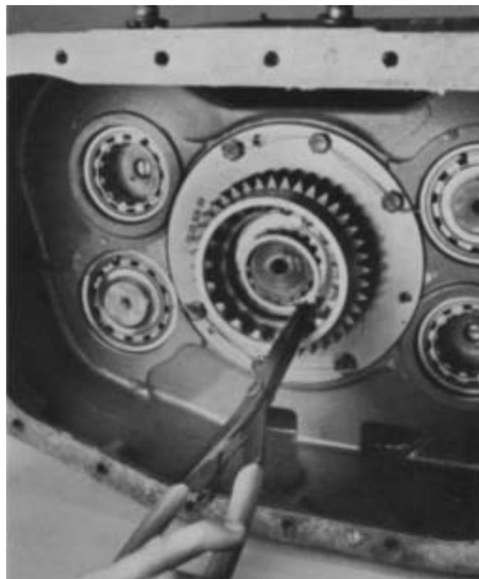
7. Install the snap ring in groove at end of mainshaft.
