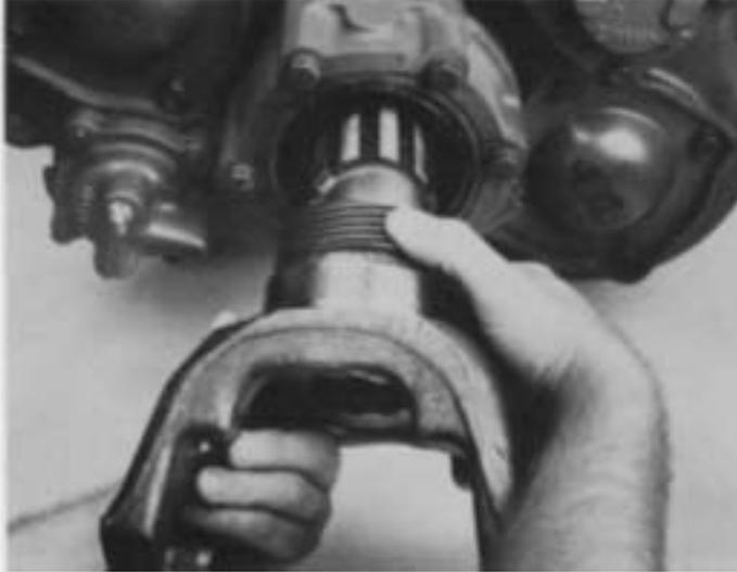
1. For models so equipped, install the speedometer drive gear or replacement spacer in position on hub of companion flange or yoke. Install the companion flange or yoke on splines of output shaft and move into rear bearing cover.
