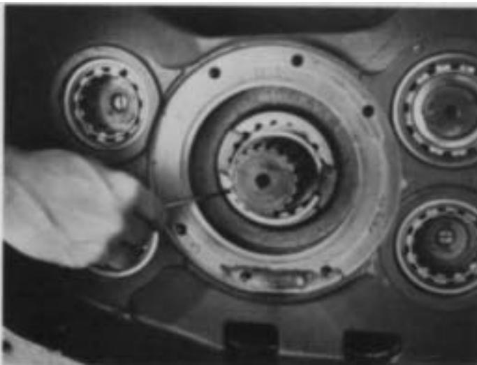
1. Move the mainshaft reverse gear as far to the rear as possible and remove the snap ring from I.D. of gear.
