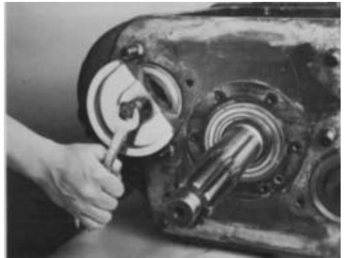
6. Use a bearing puller or pry bars to remove the countershaft front bearings.
