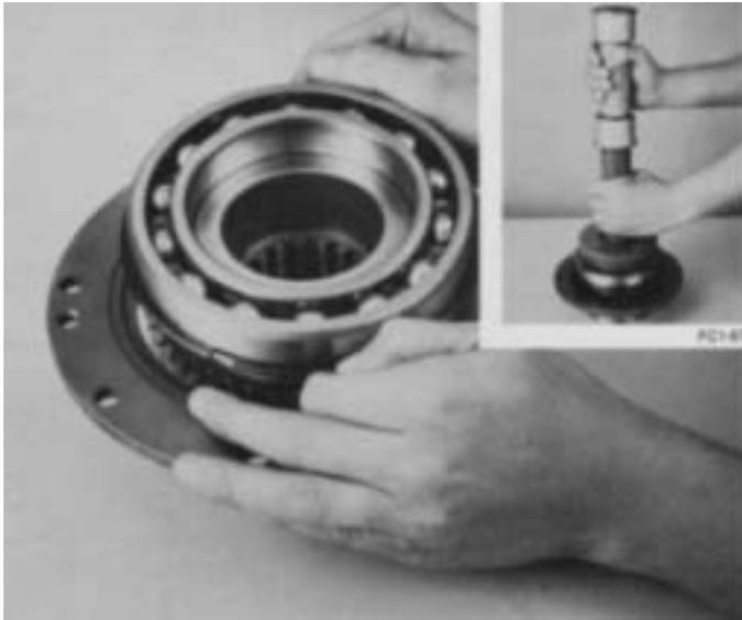
3. Start the auxiliary drive gear bearing on front hub, bearing snap ring facing groove in retainer ring. Using both the inner and outer race of bearing as a base, press the bearing on gear with snap ring in groove of retainer ring or use a bearing driver (inset).
