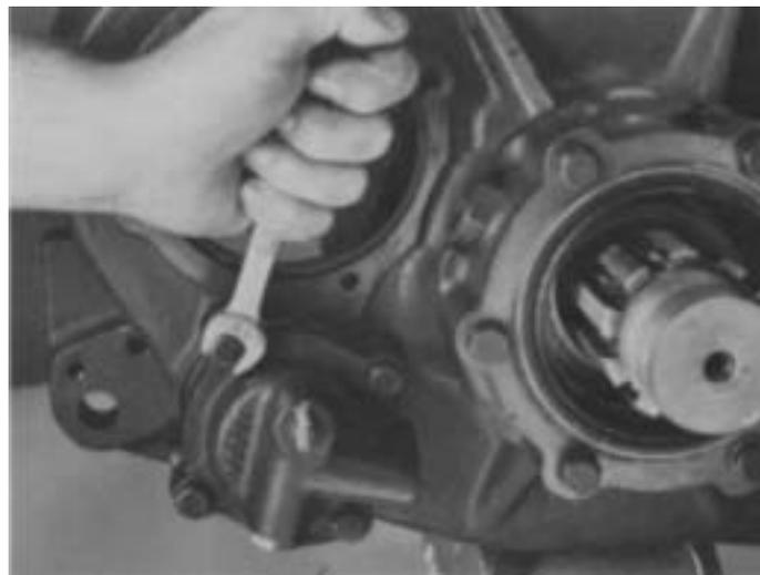
6. Position the corresponding new gasket on cover mounting surface and install the deep reduction cylinder cover, aligning the air channel with channel in cylinder housing. Tighten cap screws to secure cover to cylinder housing.
