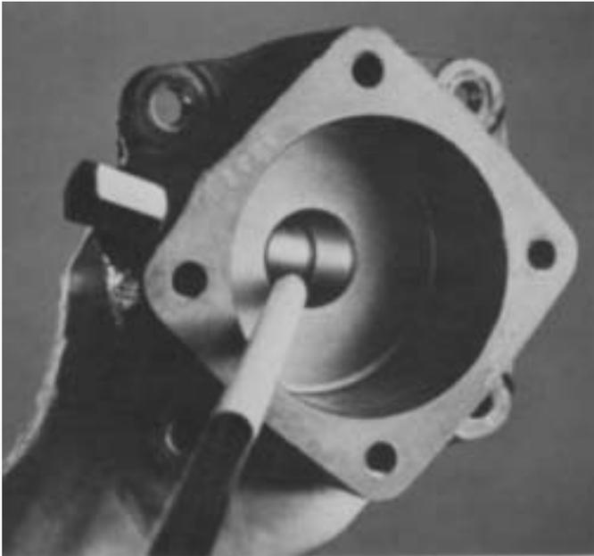
1. If previously removed, install the O-ring in bore of range cylinder housing.
