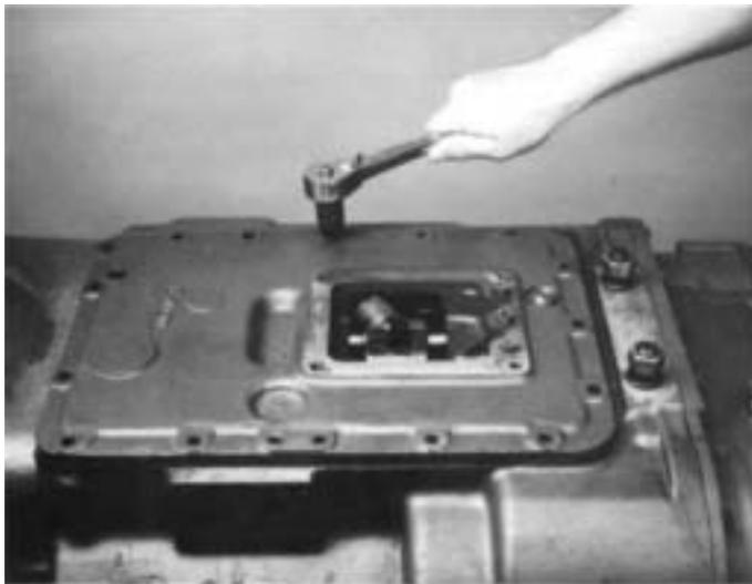
1. Turn out the retaining capscrews. Jar the top to break the gasket seal and lift the shift bar housing from the transmission case. Remove the gasket.
