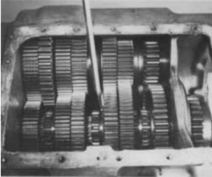
2. Engage two mainshaft sliding clutches into gear to prevent transmission from rotating.
