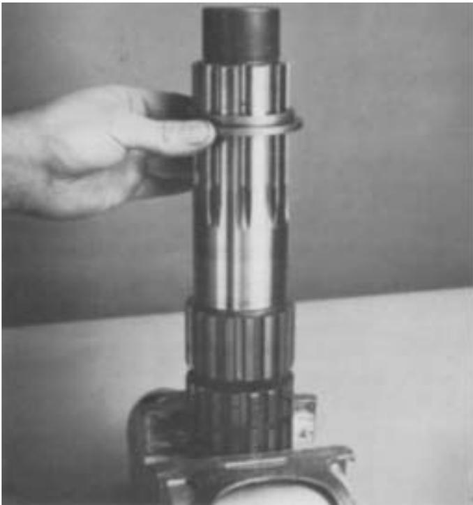
1. Remount the output shaft in vise with threaded-end up and secure on range mainshaft. For models so equipped, install the stepped washer on shaft, large diameter step down.
