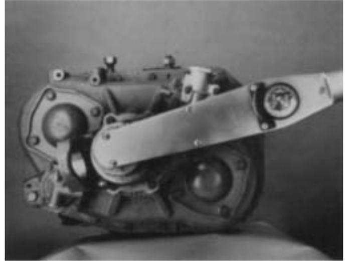
2. Lock the transmission by engaging two main-shaft gears with sliding clutches. Install the washer and/or nut on output shaft and tighten nut using 450-500 lbs/ft of torque.
