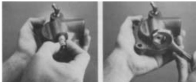
5. For models so equipped, install the insert valve in bottom exhaust port of cylinder cover as shown (left). Install the valve retaining nut in exhaust port of cover and tighten to recommended torque ratings (right).
