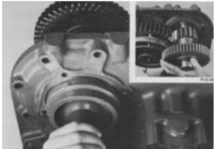
3. Place one countershaft into position in housing, meshing the marked tooth of countershaft gear with either set of two marked teeth of mainshaft deep reduction gear (inset). Center rear of countershaft in bearing bore, start rear bearing in bore and complete installation with a flanged-end driver and maul. Repeat the procedure with other auxiliary countershaft assembly, making sure the deep reduction gear set remains in time during bearing installation.
