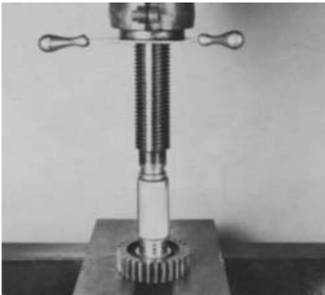
2. If previously removed, press the needle bearing into bore of reverse idler gear.
