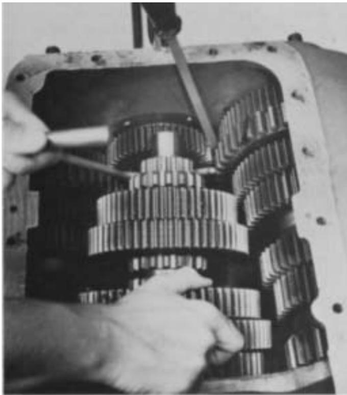
29. Block the right countershaft assembly against case wall and lower the mainshaft assembly into position with the reverse gear held against 1st speed gear and rear of shaft moved into case bore.
