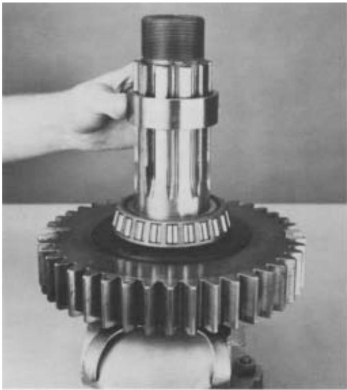
2. Remove the bearing inner spacer from output shaft.
