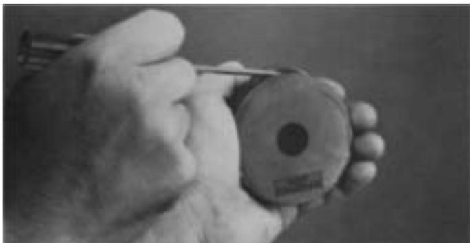
5. If previously removed, install the O-rings in the I.D. and O.D. of range piston.
