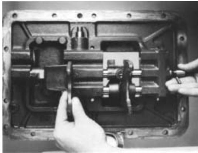
5. Move the 1st-2nd speed shift bar to the housing rear, removing the yoke and block from the bar. As the neutral notch in the bar clears the rear boss, remove the small interlock pin from the bore.
