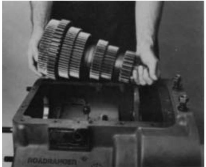
1. Place the left countershaft assembly into position in case, making sure that the "L"-marked assembly has the larger 47-tooth PTO gear.
