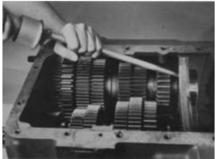
2. From inside the case, use a soft punch and maul to drive the countershaft rear bearings to the rear and from case bores.
