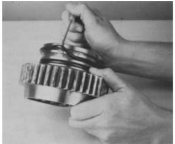
6. If necessary, remove the O-rings from hub O.D. of auxiliary drive gear.
