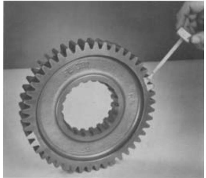
3. **IMPORTANT:** Mark any two adjacent teeth on deep reduction gear and repeat the procedure for the two adjacent teeth directly opposite the first set marked. A highly visible color of toolmakers' dye is recommended for making timing marks.
