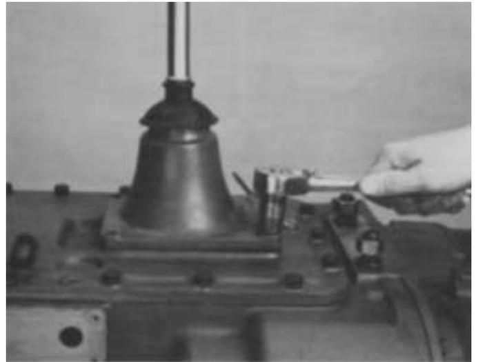
3. Install the retaining cap screws in housing flange and tighten to secure the assembly to shift bar housing.
