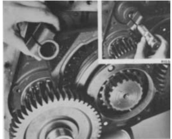
3. Place the range yoke into position with sliding clutch of synchronizer assembly, long hub of yoke to the front (RT-11610/12610 Series); long hub of yoke to the rear (RT-14610 Series). Insert threaded-end of yoke bar through yoke and into bore of range cylinder housing, aligning the notches in bar with yoke lock screw holes (inset).
