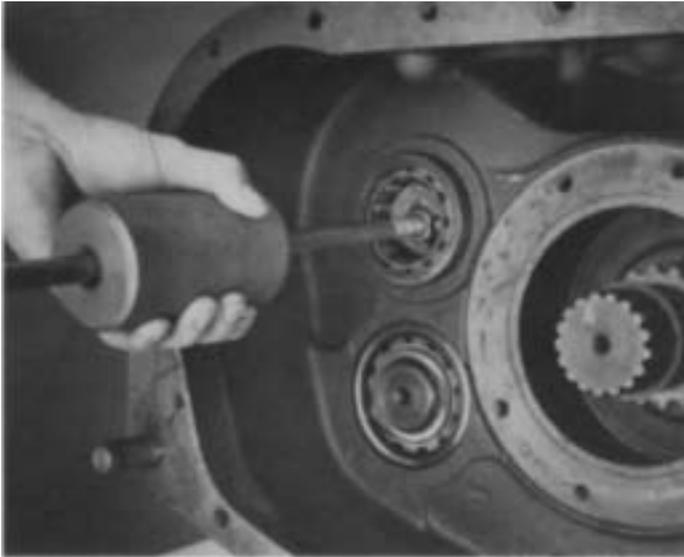
3. Using inside jaw pullers or impact puller, remove the auxiliary countershaft front bearing from left reverse idler gear bore. If necessary, repeat the procedure for removing the auxiliary countershaft front bearing from right reverse idler gear bore.
