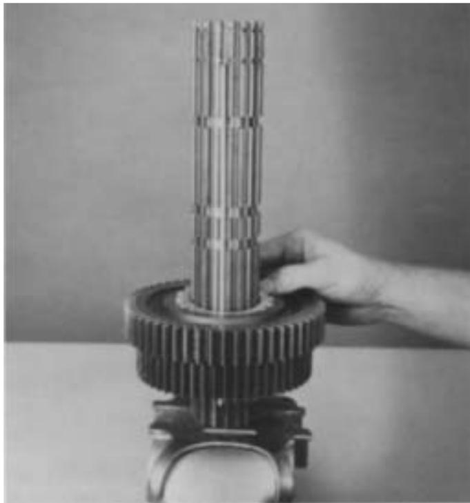
7. Install the spacer in 3rd speed gear, engaging the external splines of spacer with clutching teeth of gear.
