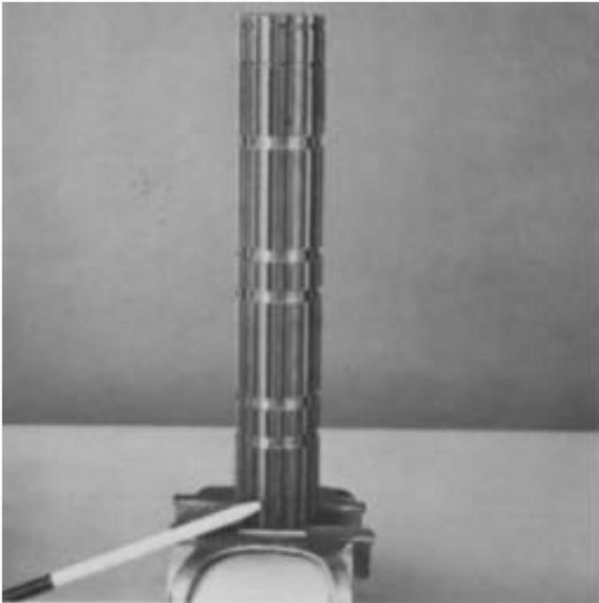
2. Secure the mainshaft in a vise equipped with brass jaws or wood blocks, pilot-end of shaft down. If previously removed, install the roll pin in keyway.
