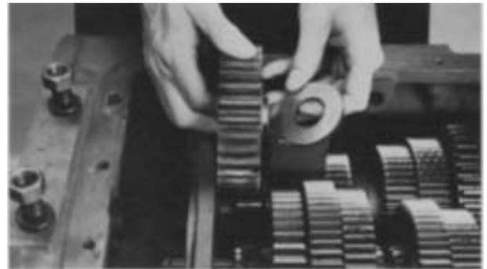
6. As the idler shaft and washer is moved to the rear, remove the thrust washer, and gear from case.
