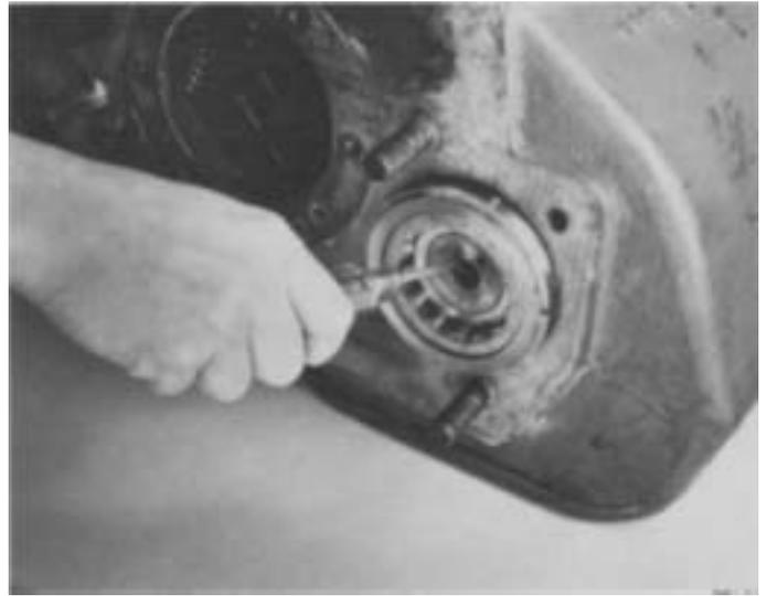
3. Center the front of left countershaft in bearing and move the assembly forward.
