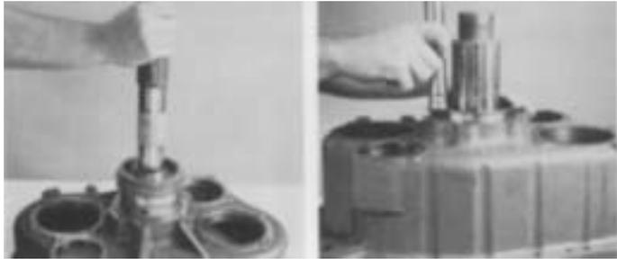
11. Stack the bearing outer spacer and rear bearing cup on top of the front bearing cup in proper sequence. Use a soft bar or a flanged driver to move all three parts evenly into housing bore until lip of rear bearing cup seats on housing.
