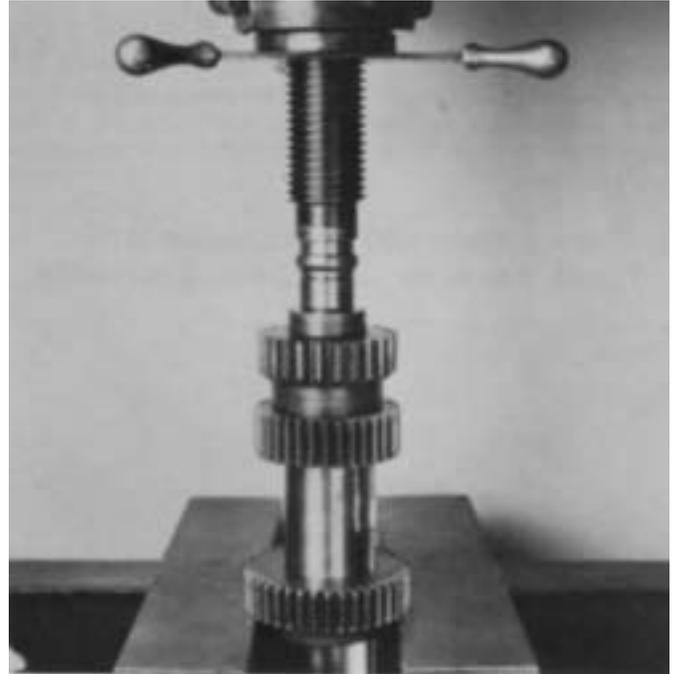
2. Align keyway of gear with key in countershaft and press the 2nd speed gear on shaft, long hub of gear to the front of countershaft.
