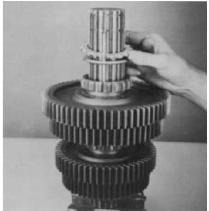
20. Install the spacer on shaft against washer.
