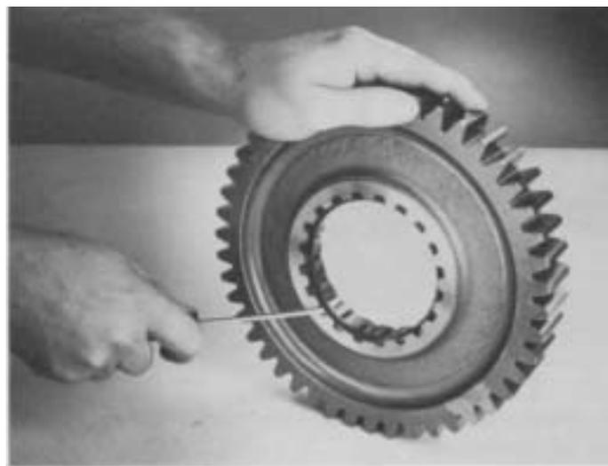
4. If necessary, remove the snap ring from low range gear of models so equipped.
