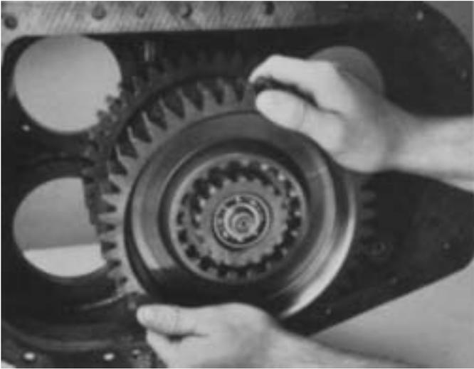
3. Pull the low range gear and washer from splines of range mainshaft.
