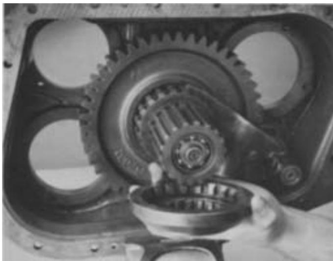
1. Install the coupler on range mainshaft, clutching teeth to the rear.
