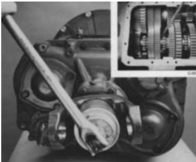
1. Lock the transmission by engaging two main-shaft gears with sliding clutches (inset). Use a large breaker bar to turn the nut from output shaft and remove washer if so equipped.
