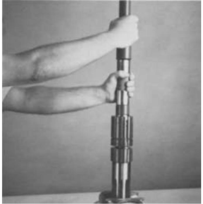
3. Install the bearings in front bore of range mainshaft. Use a small flanged-end driver to properly seat bearing in bore on mainshaft quill.
