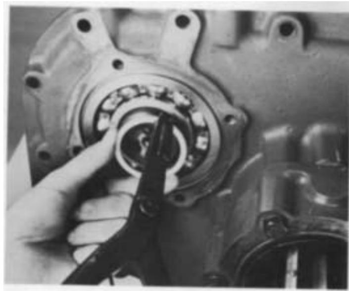
4. Install the snap ring in groove at rear of each countershaft.
