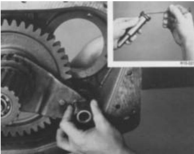
4. Pull the yoke bar from cylinder housing and remove shift yoke. If necessary, remove the O-ring from piston O.D. (inset).
