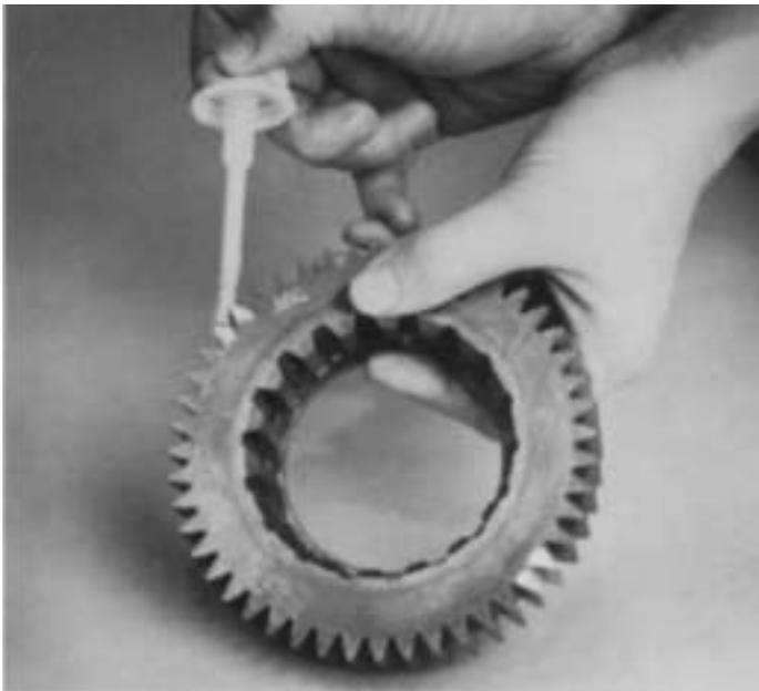
2. Mark the main drive gear for timing purposes. Mark any two adjacent teeth on drive gear and repeat the procedure for the two adjacent teeth directly opposite the first set marked. A highly visible color of toolmakers' dye is recommended for making timing marks.
