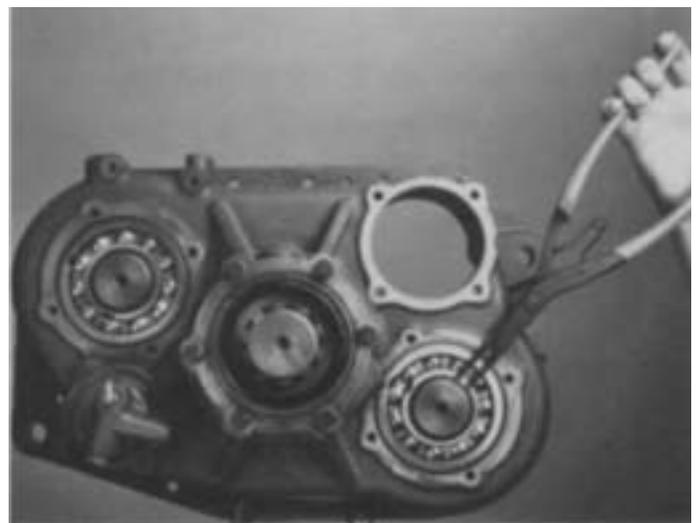
1. Turn out the capscrews and remove both countershaft rear bearing covers.
