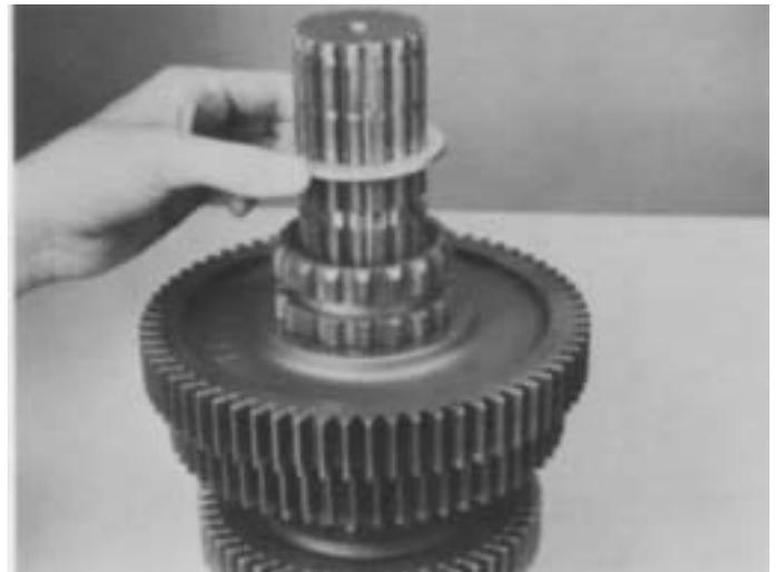
6. Turn the reverse gear limit washer to align its splines with those of mainshaft and remove washer.
