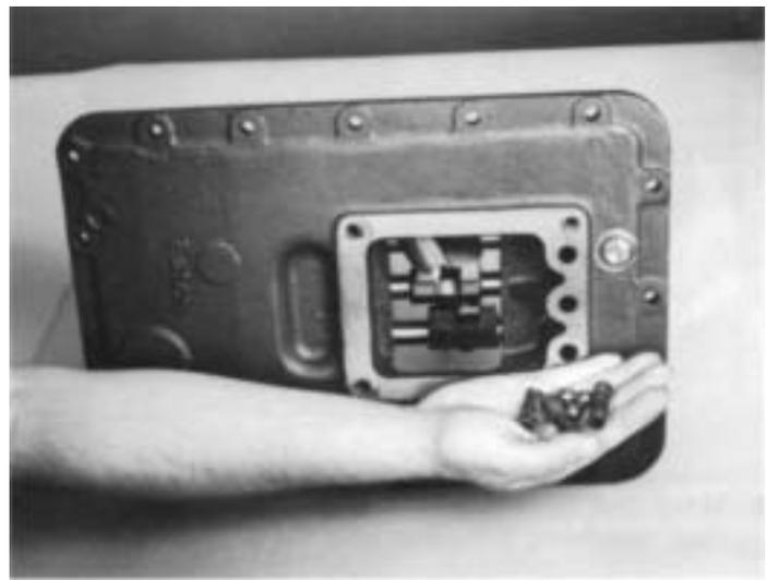
2. Tilt the assembly and remove the three sets of tension springs and balls from the housing bores.
