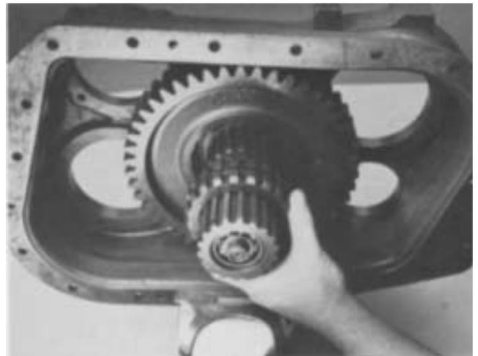
2. Remove deep reduction sliding clutch.
