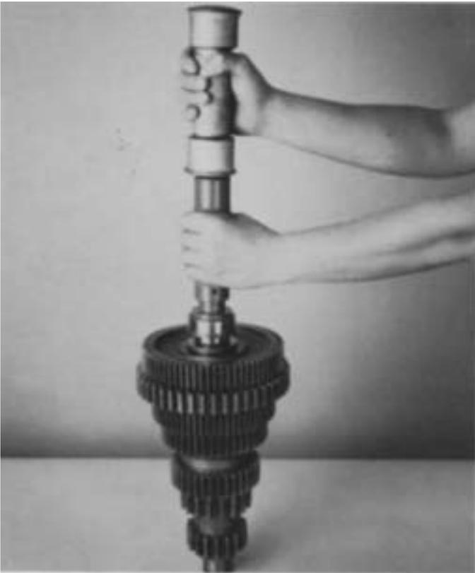
8. For models equipped with roller-type front bearings, use a rubber mallet or flanged-end driver to install bearing inner race on shaft, shoulder of race against shoulder of countershaft.
