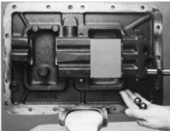
7. Move the short LO-Reverse speed shift bar to the housing rear, remove the yoke from the bar. As the shift bar is removed from the housing, two 3/4 interlock balls will drop from the rear boss bottom bore.
