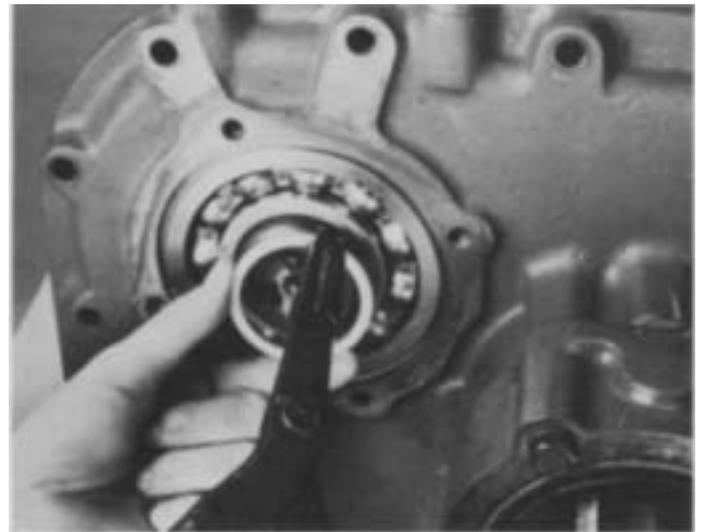
2. Remove the snap ring from groove at rear of each countershaft.
