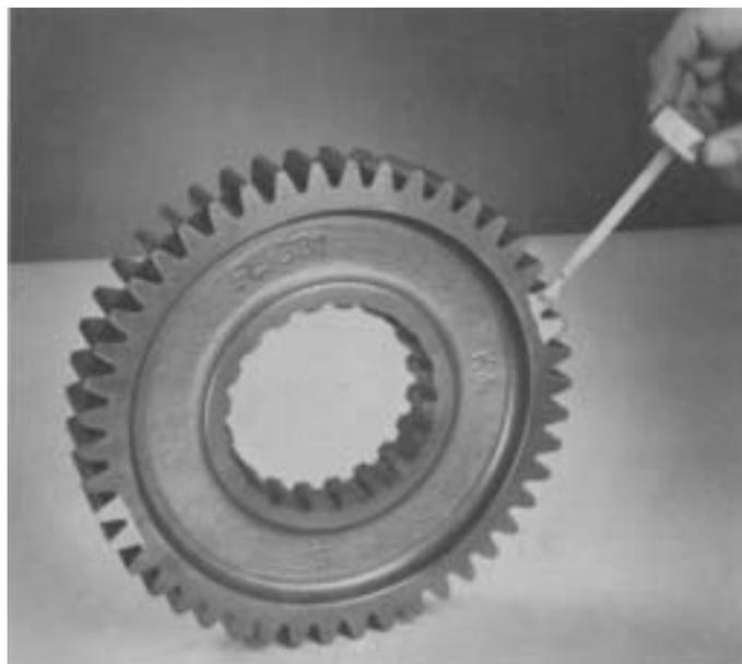
3. **IMPORTANT:** Mark any two adjacent teeth on low range gear and repeat the procedure for the two adjacent teeth directly opposite the first set marked. A highly visible color of toolmakers' dye is recommended.
