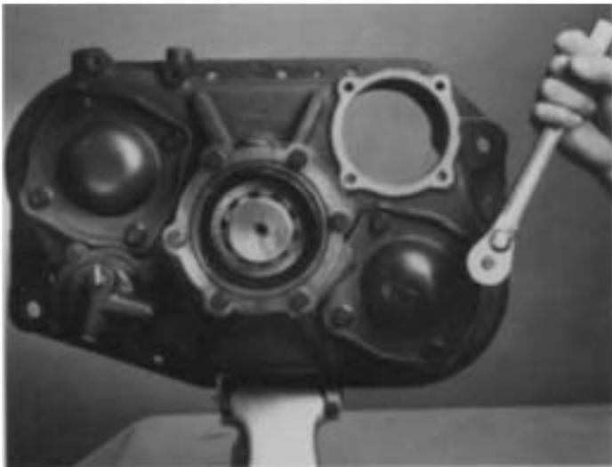
5. Position the corresponding new gasket on cover mounting surface and install both rear bearing covers. Tighten capscrews to secure covers to auxiliary housing.
