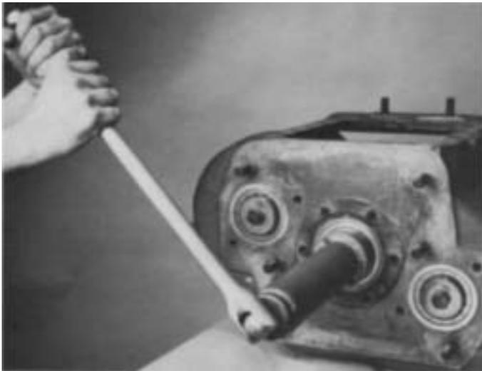
3. Install the nut on shaft (left hand threads). Using a drive gear nut installer, tighten to 250-300 lbs/ft of torque. Use a punch and maul to peen the nut into the two milled slots of input shaft.
