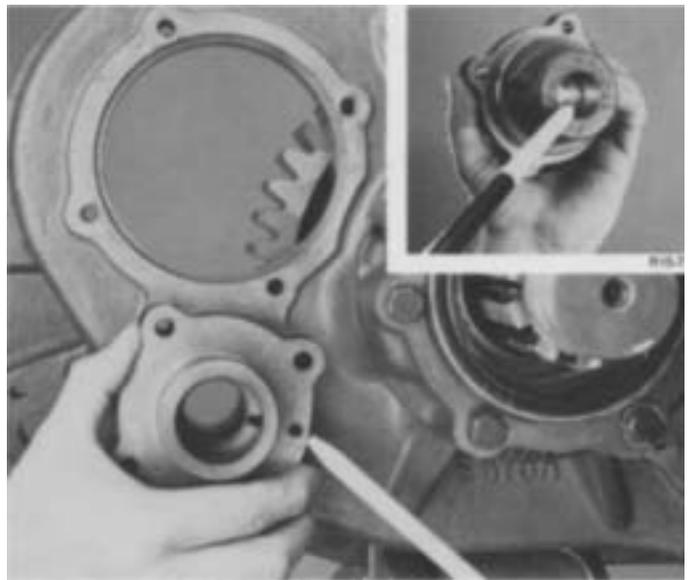
1. If previously removed, install the small O-ring in bore of cylinder housing (inset). Position the corresponding new gasket on housing mounting surface and install the deep reduction cylinder housing in rear bore of auxiliary housing, air channel to the right.
