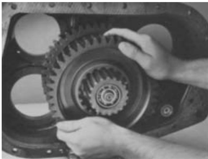
2. Install the low range gear on mainshaft against coupler, clutching teeth.
