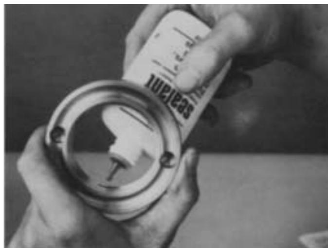
1. Apply Loctite grade 277 sealant to cleaned threads of new drive gear bearing nut. **DO NOT REUSE OLD NUT.**
