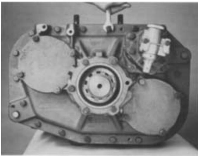
2. Install the retaining capscrews in flange of auxiliary plate/housing and tighten to secure the auxiliary section to the front section. See **TORQUE RECOMMENDATIONS**.
