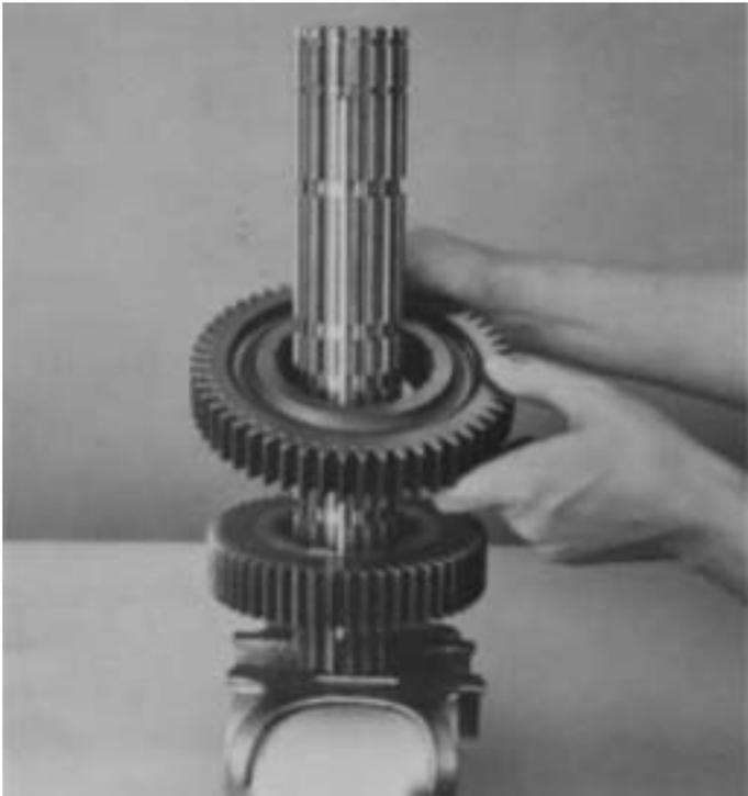
6. Install the 3rd speed gear on shaft against 4th speed (or Overdrive) gear, clutching teeth up.
