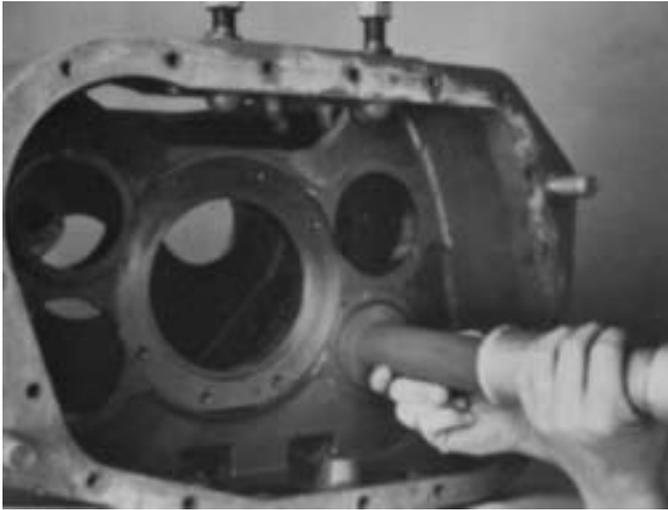
5. Install the OUTER RACE of auxiliary countershaft front bearing into case bore and against washer.
