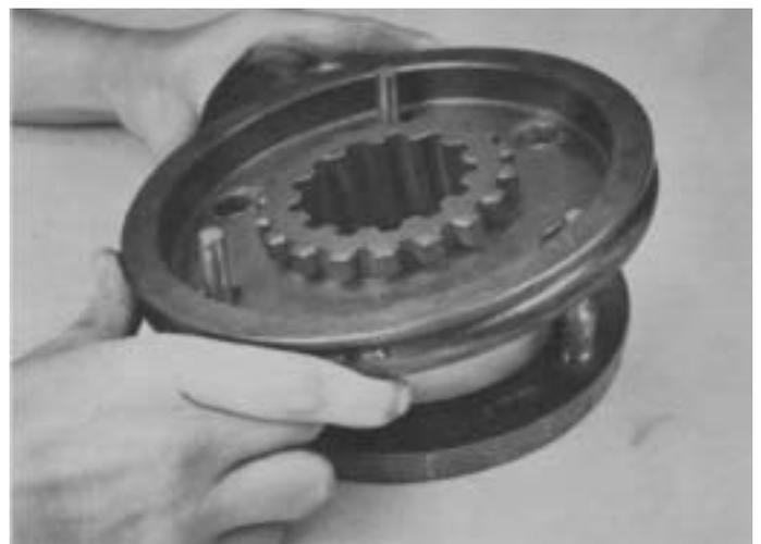
3. Remove the sliding clutch from pins of low range synchronizer ring.
