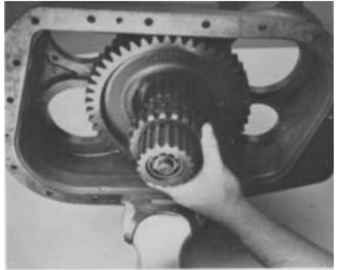
14. Remount assembly upright in vise and secure. Install the deep reduction sliding clutch on output shaft, internal splines toward gear and engaged with splines of shaft.
