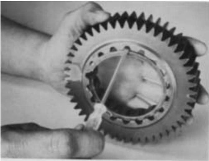
4. If necessary, remove the snap ring from drive gear.
