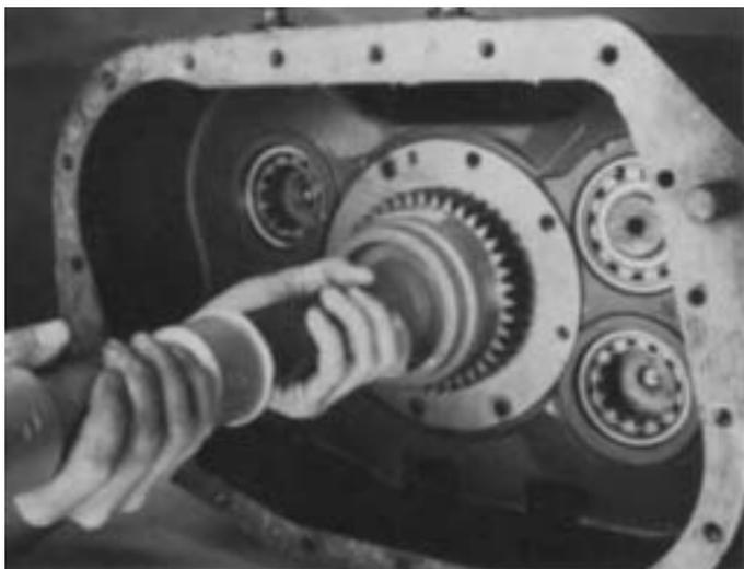
5. Reinstall the auxiliary drive gear assembly on rear of mainshaft. Use a flanged-end driver and maul to seat bearing in case bore.
