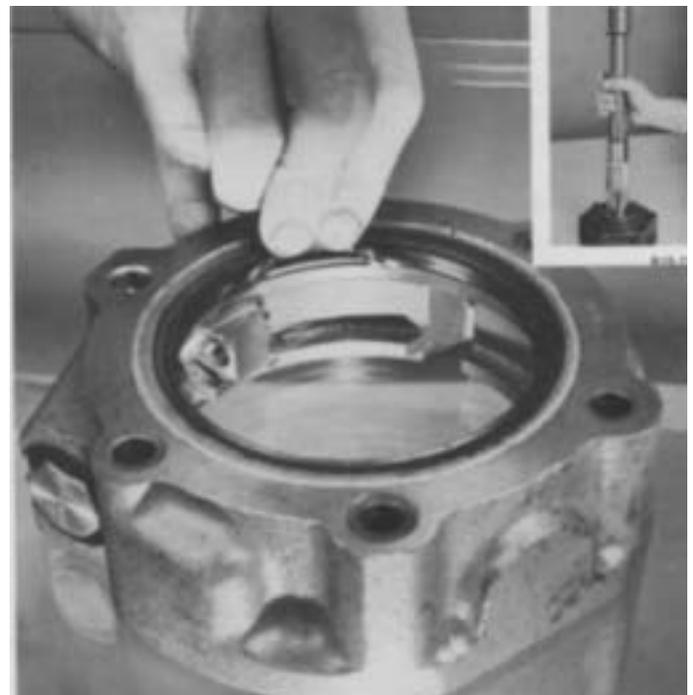
12. If previously removed, install the oil seal in rear bearing cover with a flanged driver (inset). Seal should be installed so the spring is to the front of transmission.
