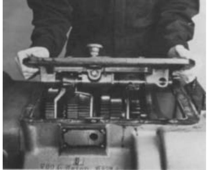
Install the new shift bar housing gasket in position on case.
