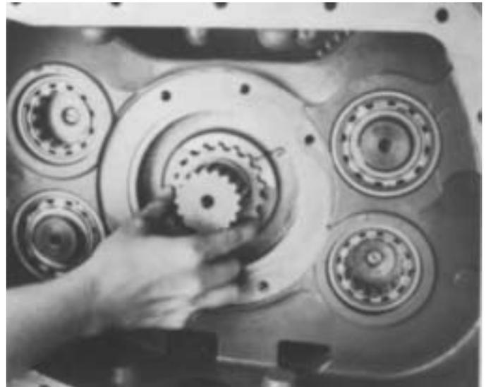
3. Align the external splines of spacer with clutching teeth of reverse gear and move spacer forward on mainshaft and into gear.
