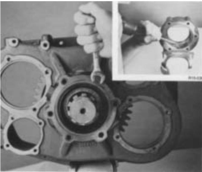
1. Turn out the capscrews and remove the rear bearing cover and gasket. If necessary, remove the oil seal from cover (inset).
