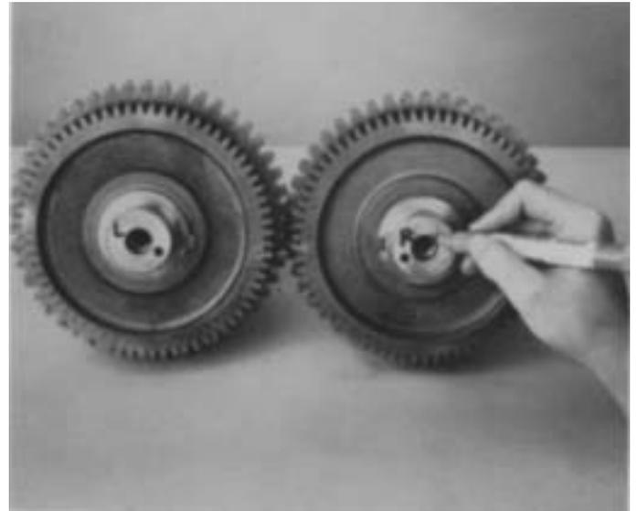
6. To avoid confusion during installation, mark the end of left countershaft with an "L"; the end of right countershaft with an "R".
