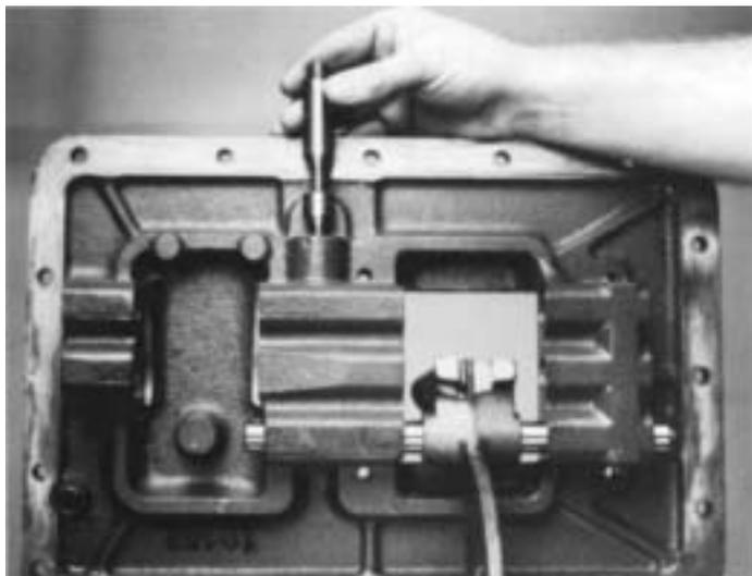
6. Remove the actuating plunger from the center boss bore.
