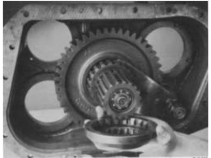
4. Remove the coupler from splines of range mainshaft.
