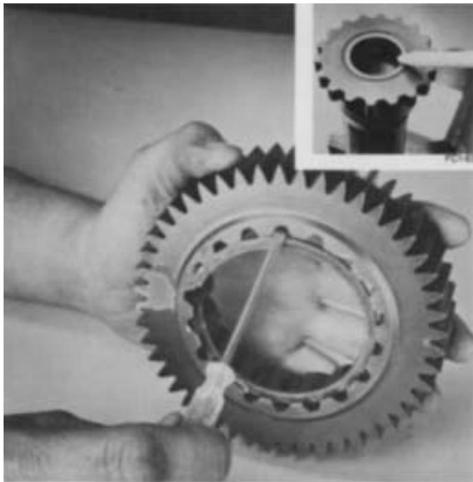
1. If previously removed, install the snap ring in I.D. of main drive gear and the bushing in pocket of input shaft (inset).
