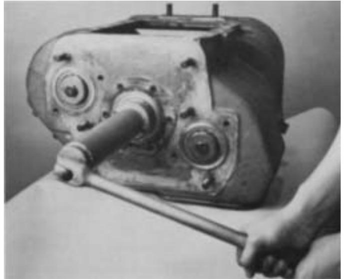
3. Engage two mainshaft sliding clutches into gear, this prevents transmission from rotating. Remove nut (left hand thread) with drive gear nut removing tool.
