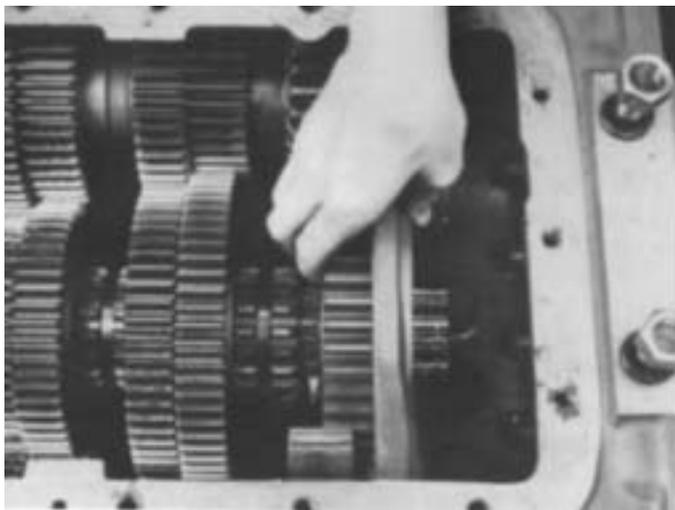
2. Move the reverse gear to the rear as far as possible, meshing teeth of gear with those of the reverse idler gears.
