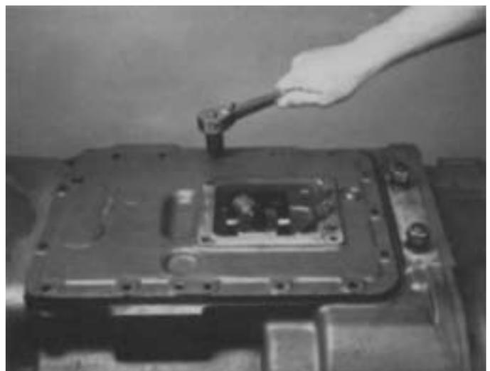
3. Install the capscrews in housing and tighten to secure the assembly to case.
