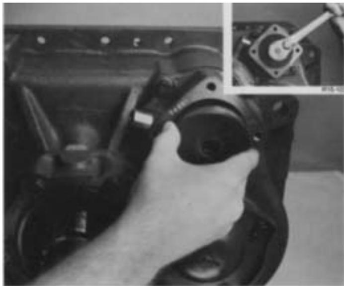
6. In cylinder housing bore, install the range piston on yoke bar, flat side to the rear. Secure with nut tightened to recommended torque ratings (inset).
