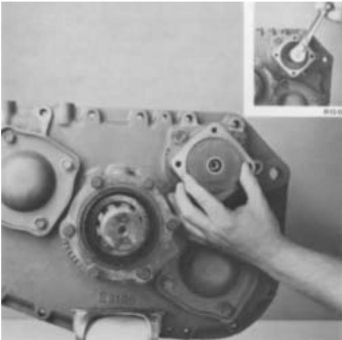
6. In cylinder housing bore, install the range piston on yoke bar, flat side to the rear. Secure with nut tightened to recommended torque ratings (inset).
