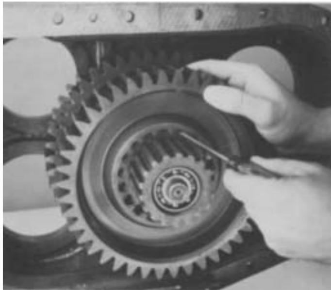
3. Install the splined tolerance washer on mainshaft and in hub of low range gear. Rotate the washer in groove of mainshaft to engage external splines with clutching teeth of gear and align square internal spline with keyway of mainshaft.
