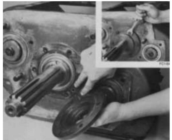
5. Install the drive gear bearing cover and gasket, making sure to align the oil return hole in case. Secure cover on case with retaining capscrews (inset).
