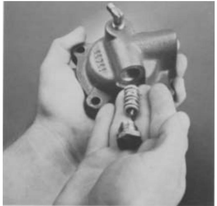
2. If necessary, turn out the insert valve retaining nut of covers so equipped and remove insert valve from bore.
