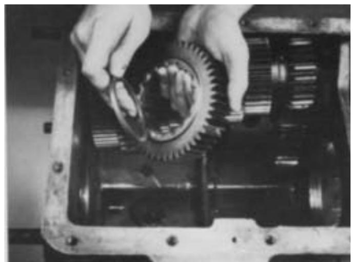
2. Move upper countershaft to right and remove drive gear and spacer from case.
