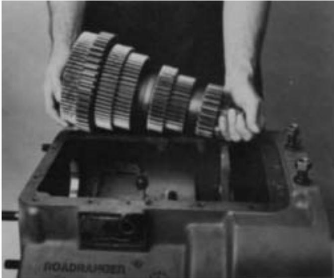
1. Move the right countershaft assembly to the rear as far as possible so front of shaft can be removed from case bore and moved to the center of case. Lift the assembly from case and repeat the procedure for left countershaft assembly.
