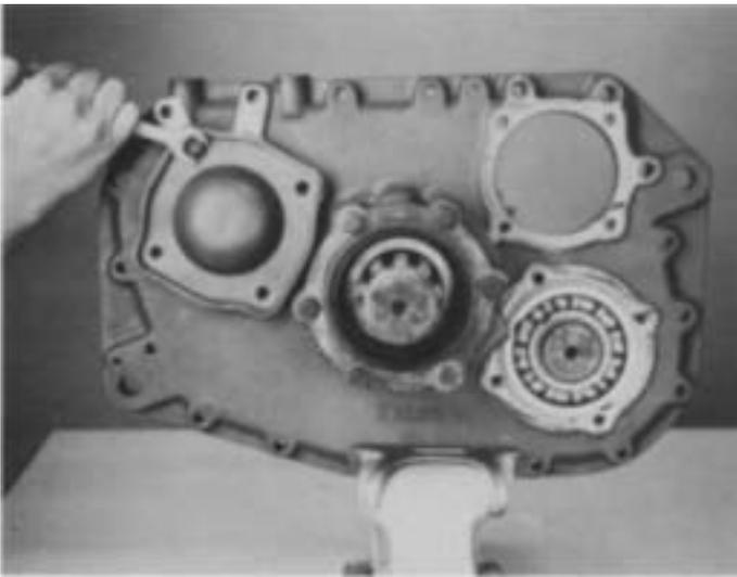
1. Turn out the capscrews and remove both countershaft rear bearing covers and gaskets.
