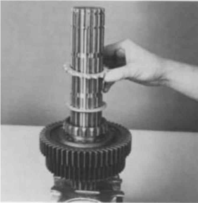
12. Install the spacer on shaft against washer.
