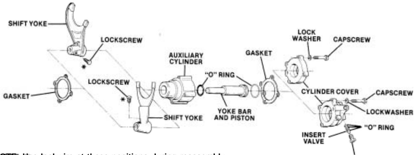
**NOTE:** Use lockwire at these positions during reassembly.
