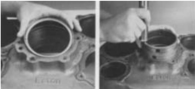
6. Place the oil retention ring in housing bore, cupped side up (left). Use a soft bar and two rear bearing outer spacers stacked on top of each other to move the oil retention ring 2" deep into bore. The ring will be at the proper depth when top of second spacer is flush with housing bore. Remove the spacers when installation is completed.
