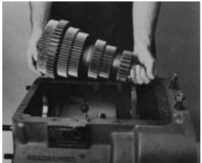
2. Place the right countershaft assembly into position in case, making sure that the "R"-marked assembly has the smaller 45-tooth PTO gear.
