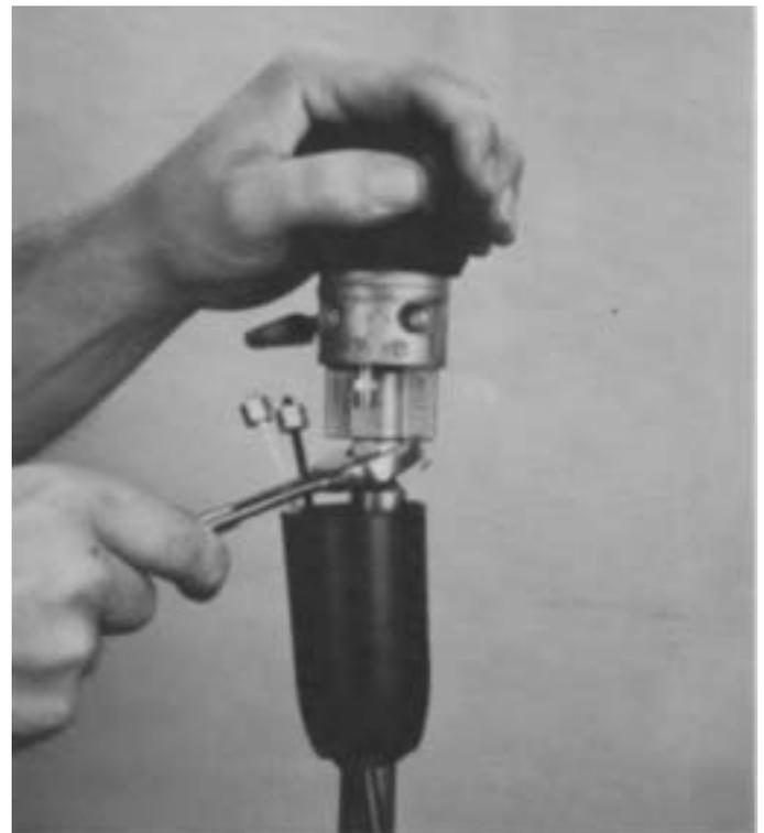
6. Loosen the jam nut and turn the Roadranger Valve and nut from gear shift lever. Remove the valve cover, air lines, sheathing and O-rings from lever.
