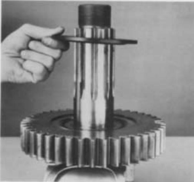
5. Install the washer on shaft; 11610, 12610 models flat side of washer facing up, 14610 models flat side of washer facing down.
