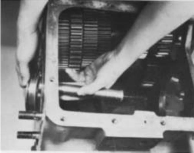
3. Drive the input shaft bearing out the front of case.
