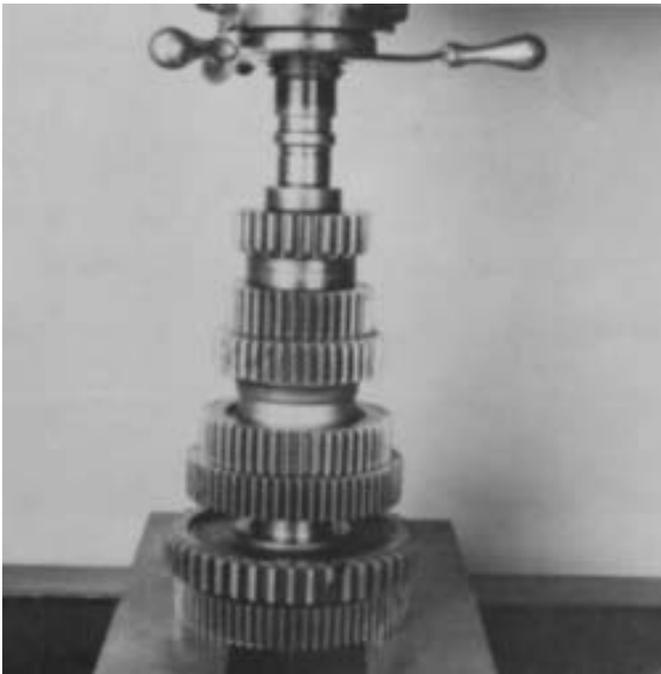
5. Start the PTO gear onto countershaft, bullet-nose side of teeth facing up and toward rear of shaft. Align keyway of drive gear with key in countershaft and press BOTH gears onto shaft, long hub of drive gear against PTO gear.
