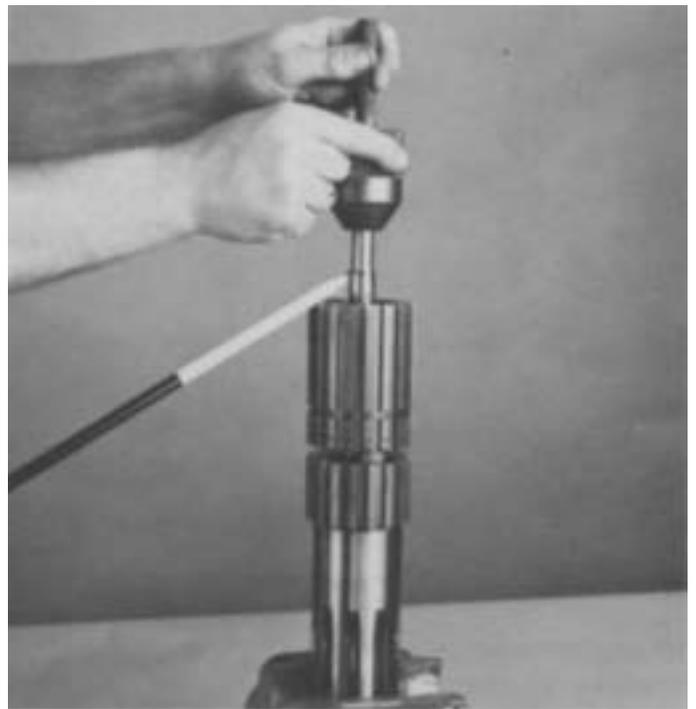
4. Install the "C" ring in groove of mainshaft quill to retain bearing.
