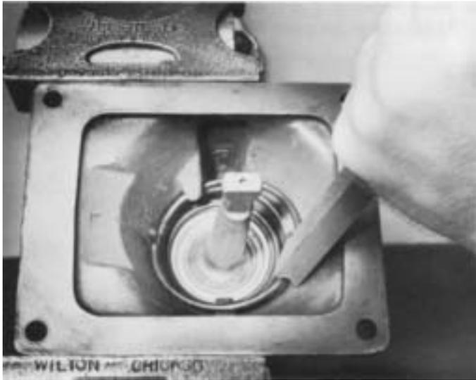
3. Install the tension spring under lugs in housing, seating one coil at a time. Use of a spring driving tool is recommended.
