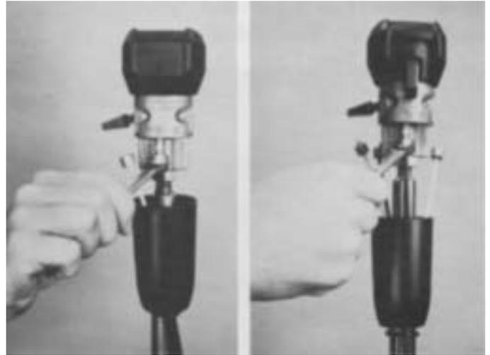
5. Slide the cover down shift lever to expose valve ports and disconnect the two 1/8" O.D. air lines at the A-5010 valve OR the four 1/8" O.D. air lines at the A-5015 valve.
