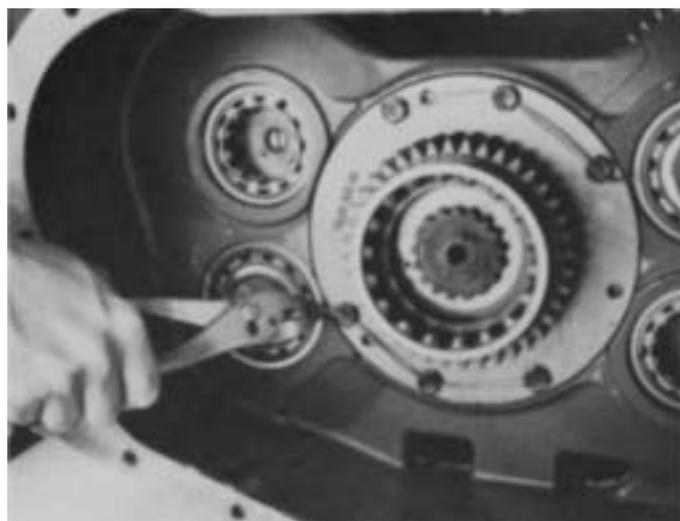
6. Align the six capscrew holes in retainer with the tapped holes in case and install capscrews. Tighten to recommended torque ratings and lock-wire the capscrews in groups of three.
