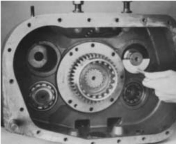
2. Insert countershaft support tool or blocking in rear bearing bore.
