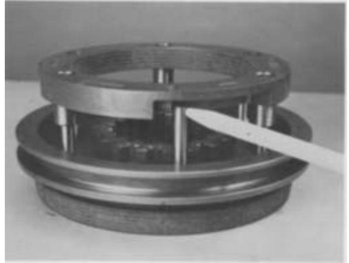
3. Place the high range synchronizer ring over blocker pins of low range synchronizer, seating the springs against pins.
