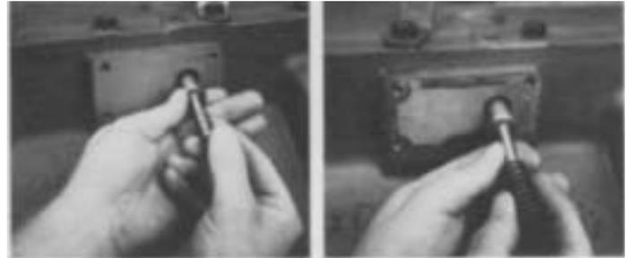
5. Remove the spring and plunger pin from bore in transmission case. Remove slave valve gasket.
