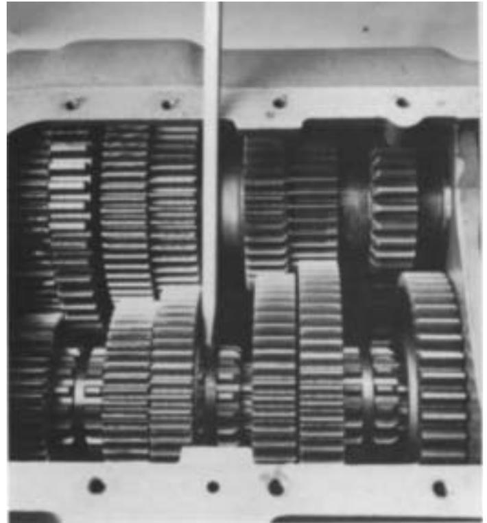
5. Move the reverse gear to the rear on mainshaft and use a screwdriver to engage sliding clutches with all forward speed gears. A sliding clutch that will not engage with a gear indicates the gear set is not in proper mesh. The bearings of the right countershaft would then need to be removed and the drive gear set retimed.
