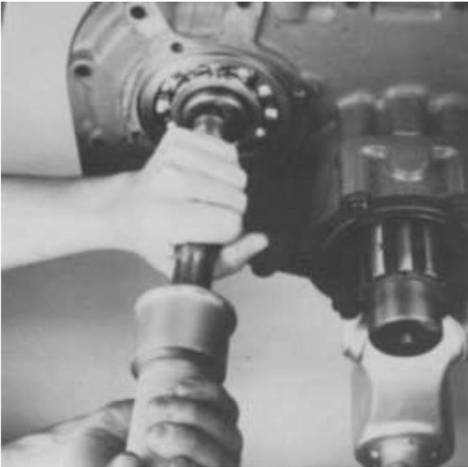
3. Use a soft bar and maul to drive the countershaft forward and from rear bearings.
