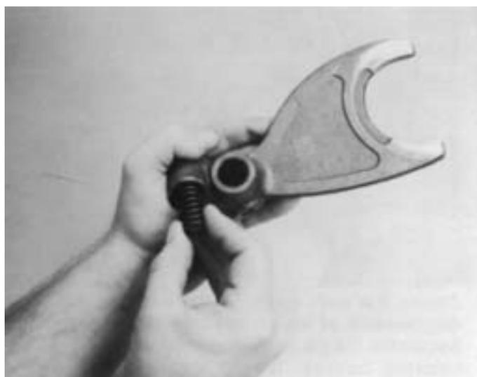
2. Install the spring in the yoke bore and on the plunger shank.
