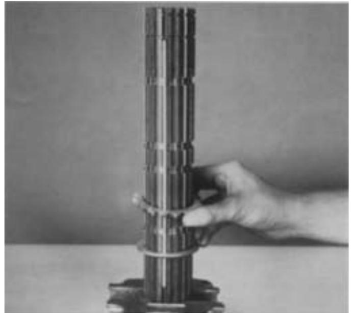
4. Install the spacer on shaft against washer.
