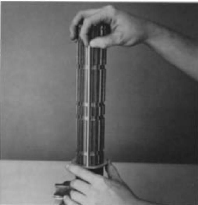
3. Install the 4th speed gear limit washer on mainshaft, flat side of washer up. Rotate washer in the 1st or bottom groove of mainshaft to align the splines of washer with those of the mainshaft. Install the key in mainshaft keyway to lock washer in place.
