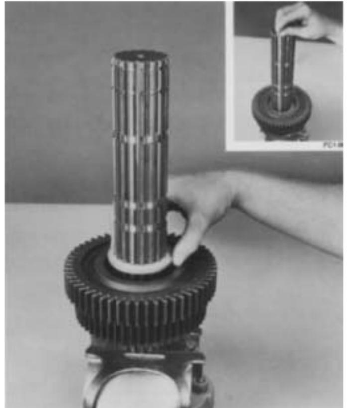
8. Remove the key from keyway and install the 3rd speed gear limit washer on mainshaft, flat side of washer down and against spacer. Rotate washer in the 2nd groove of mainshaft to align the splines of washer with those of the mainshaft and reinsert key in keyway to lock washer in place (inset).
