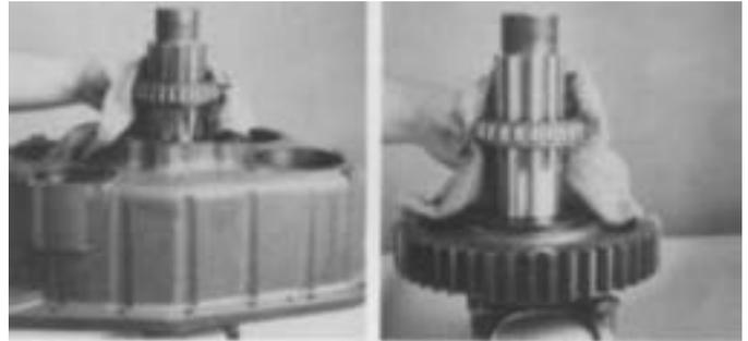
8. Heat the front bearing cone and install on output shaft against oil retention ring, bearing taper-up (left). For models not equipped with the oil retention ring in auxiliary housing, install the heated bearing cone on shaft against washer, taper up (right).
