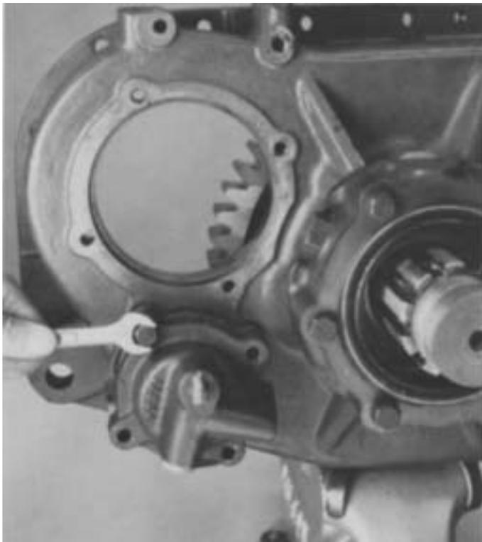
1. Turn out the capscrews and remove the deep reduction cylinder cover and gasket.
