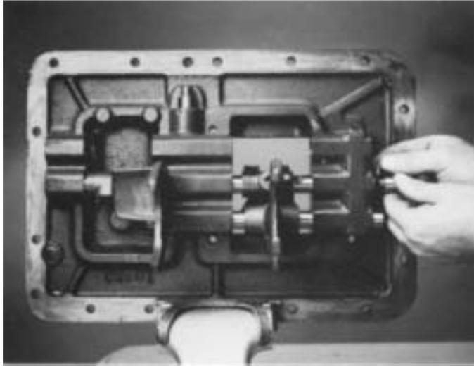
7. While holding the notched-end of the bar, install the 1st-2nd speed shift bar in the housing boss middle bore. Position the shift block on the bar between the center and rear bosses, and the yoke on the bar between the front and center bosses, long hub to the housing front. Just before inserting the notched-end of the rear boss bar, install the small interlock pin VERTICALLY in the neutral notch bore. Install the block and yoke lockscrews, tighten, and lockwire securely.
