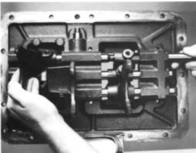
4. Move the 3rd-4th speed shift bar to the housing rear, removing the yoke and block from the bar.
