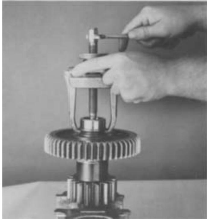
4. If necessary, secure the assembly in a vise and remove the bearing inner race from front of countershaft with jaw pullers.
