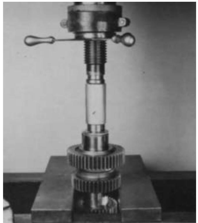
4. Using the rear face of 2nd speed gear as a base, press the 3rd speed and 2nd speed gears from each countershaft.
