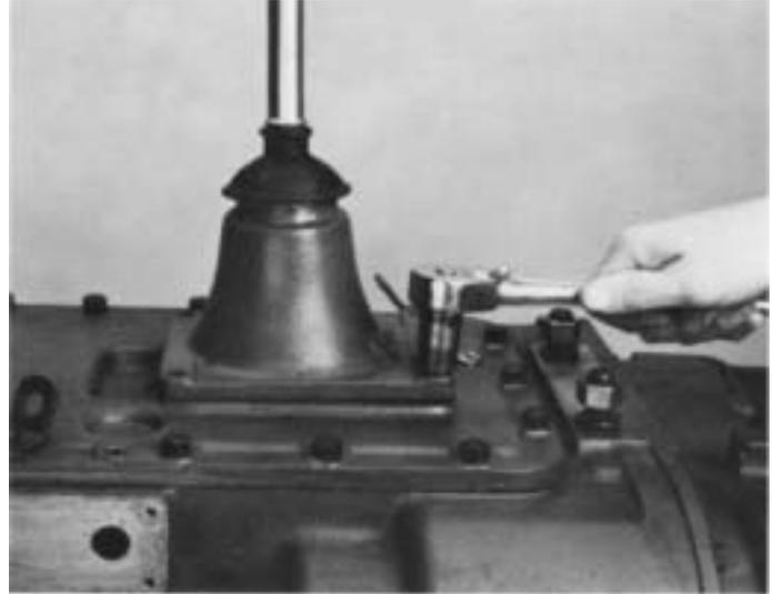
1. Turn out the four retaining cap screws, jar lightly to break gasket seal and remove the gear shift lever housing and gasket from shift bar housing.
