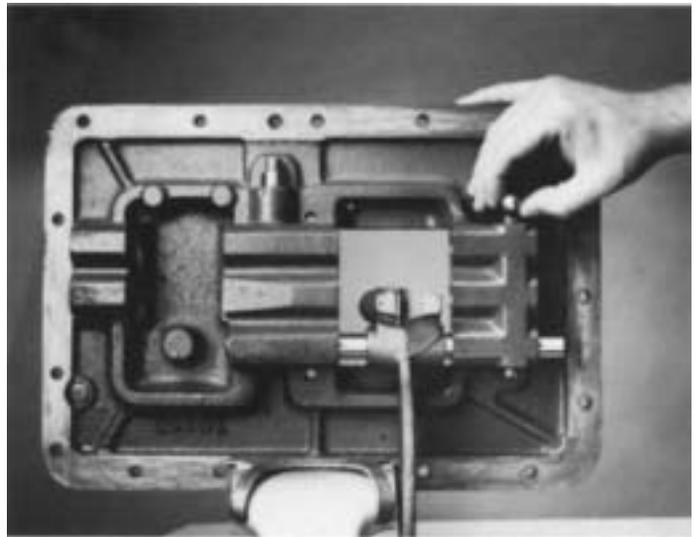
6. Install one 3/4" interlock ball in the rear boss top bore. This ball rides between LO-Reverse and 1st-2nd speed shift bars.
