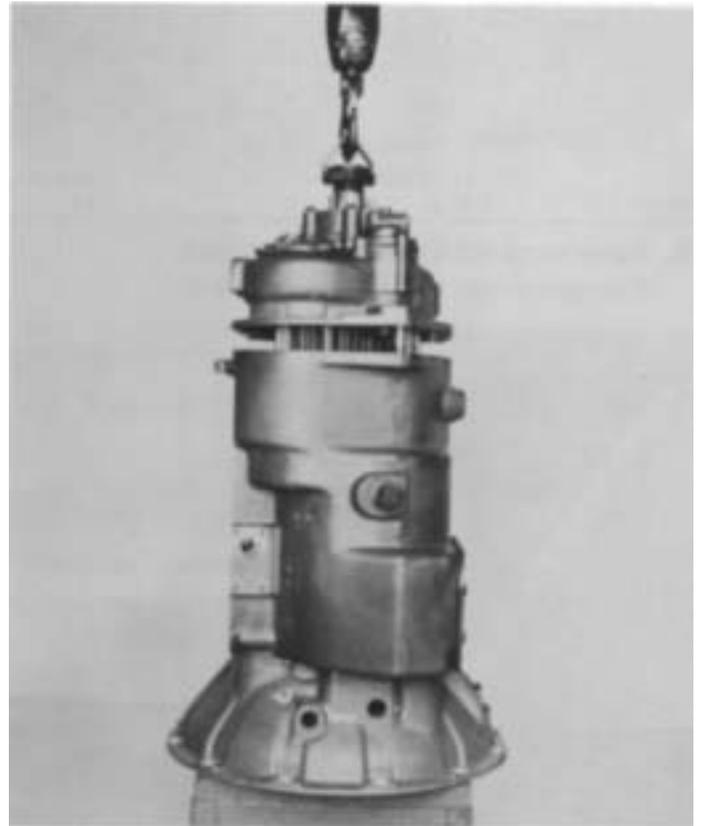
4. The auxiliary section can also be removed with transmission set in the vertical position. Block <sup>o</sup> under the clutch housing to prevent damage to the input shaft, remove the retaining capscrews in housing flange and lift the assembly from front section. Remove gasket.
