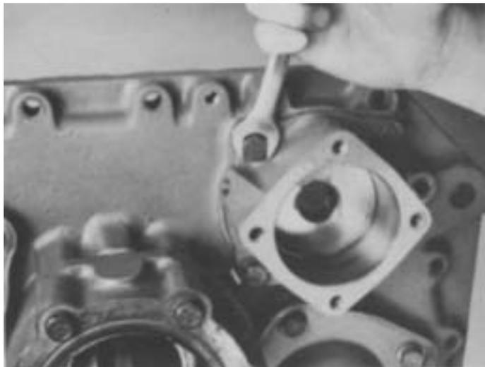
2. Position the corresponding new gasket on housing mounting surface and install the cylinder housing in rear bore of auxiliary plate, air fitting to the upper left. Secure housing to plate with capscrews tightened to recommended torque ratings.
