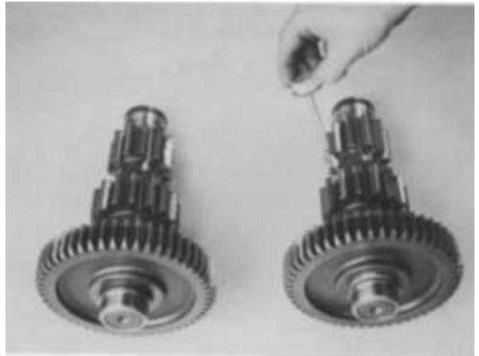
2. **IMPORTANT:** On the low range gear of each auxiliary countershaft assembly locate the "O" stamped on one tooth. Align tooth with "O", with smaller deep reduction gear tooth and mark with high visible color of toolmakers' dye.
