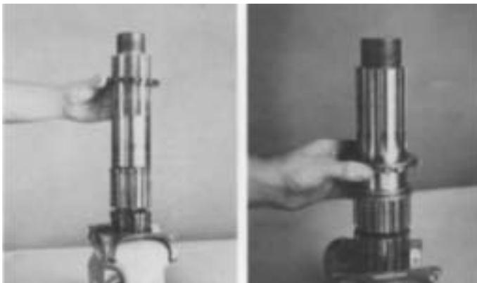
2. Install the splined spacer on output shaft. For models equipped with stepped washer on shaft, install the spacer with large diameter splines down (right).
