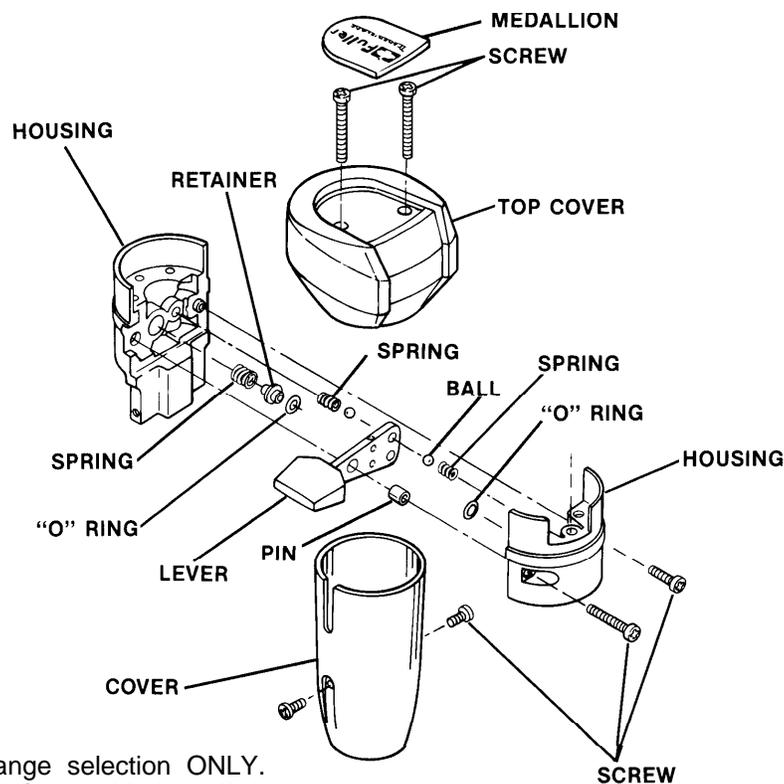
**NOTE:** This valve provides range selection ONLY. When equipped on 15-Speed Models, the dash-mounted Deep Reduction Valve is required to provide deep reduction selections.
