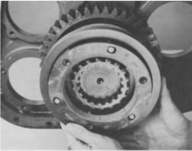
1. Pull the synchronizer assembly from the splines of output shaft.
