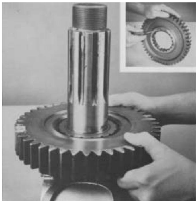
4. If previously removed, install the snap ring in low range gear of models so equipped (inset). Install the gear on output shaft, clutching teeth down and engaged with splines of spacer.
