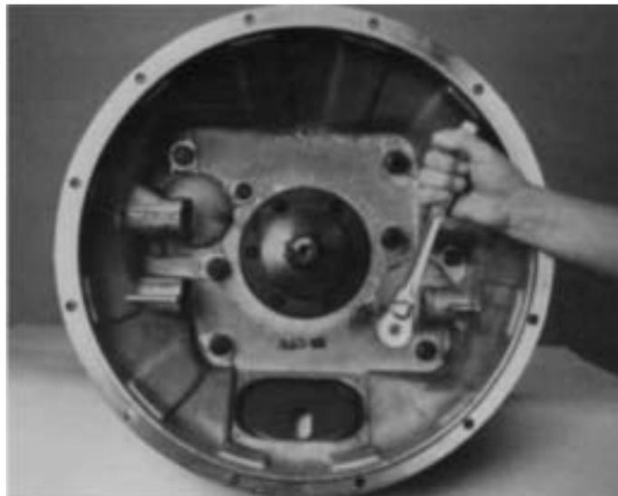
3. Install the four cap screws with lockwashers and tighten. See TORQUE RECOMMENDATIONS.
