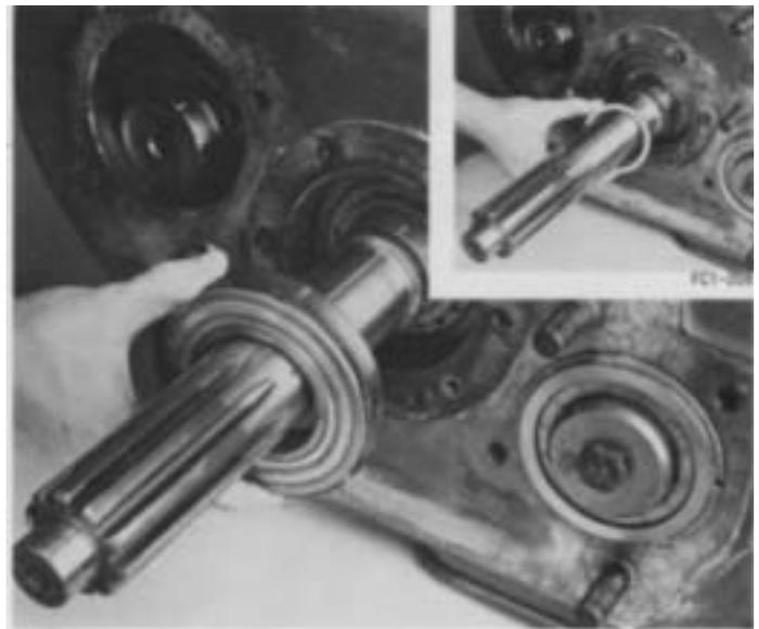
4. Install spacer (inset) and bearing on the input shaft with external snap ring to the outside.
