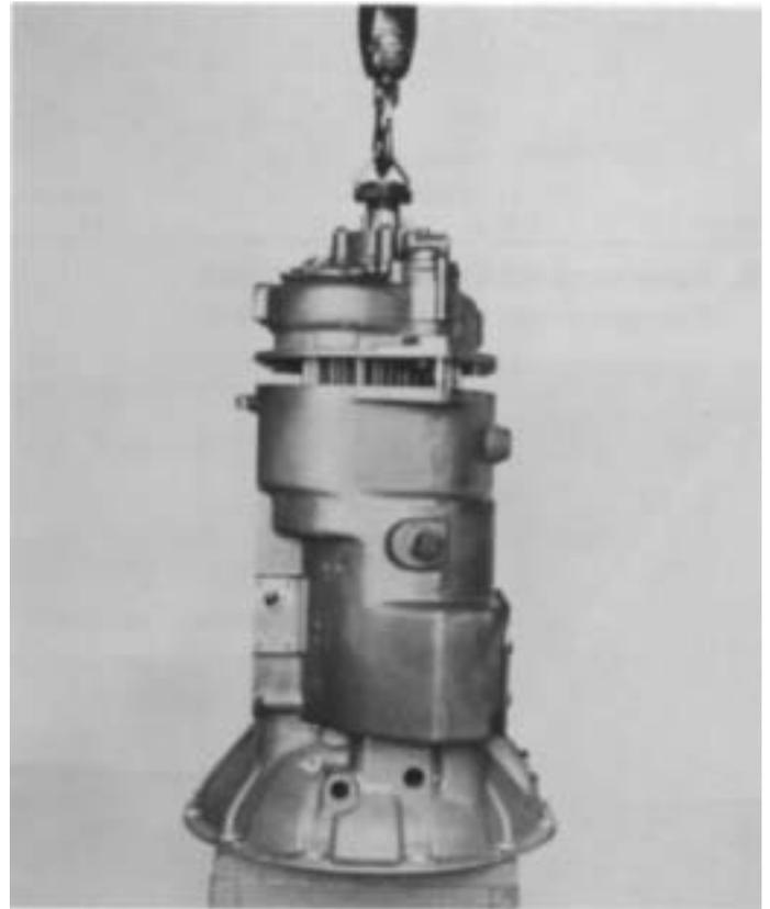
4. The auxiliary section can also be removed with transmission set in the vertical position. Block <sup>⊙</sup> under the clutch housing to prevent damage to the input shaft, remove the retaining capscrews in housing flange and lift the assembly from front section. Remove gasket.
