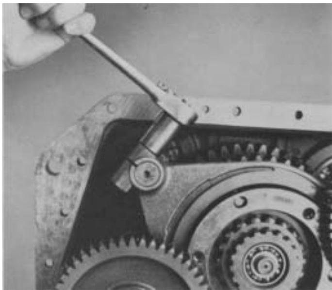
4. Install the two yoke lock screws, tighten and wire securely.
