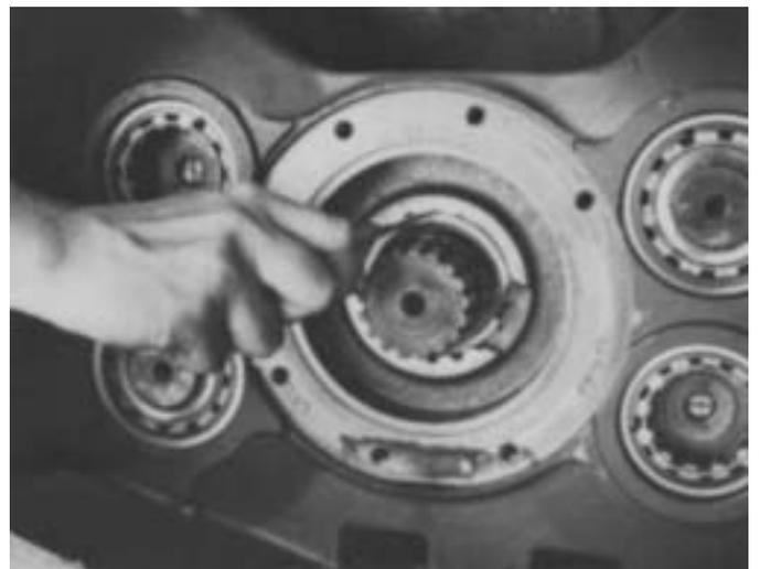
4. Install the snap ring in hub of reverse gear and move the reverse gear forward on mainshaft and into proper position in case.
