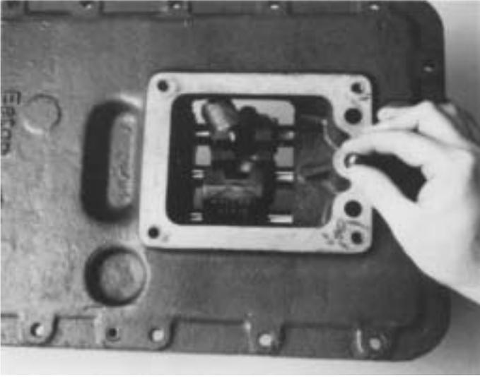
**11.** Remove the assembly from the vise. Install the three tension balls, one in each bore on the housing top.
