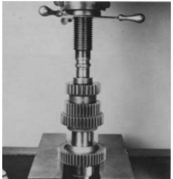
3. Press the 3rd speed gear on countershaft, long hub of gear against 2nd speed gear hub.
