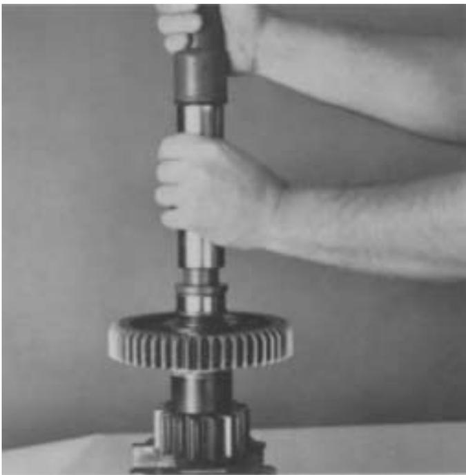
1. If previously removed, install the bearing inner race on front of each countershaft.
