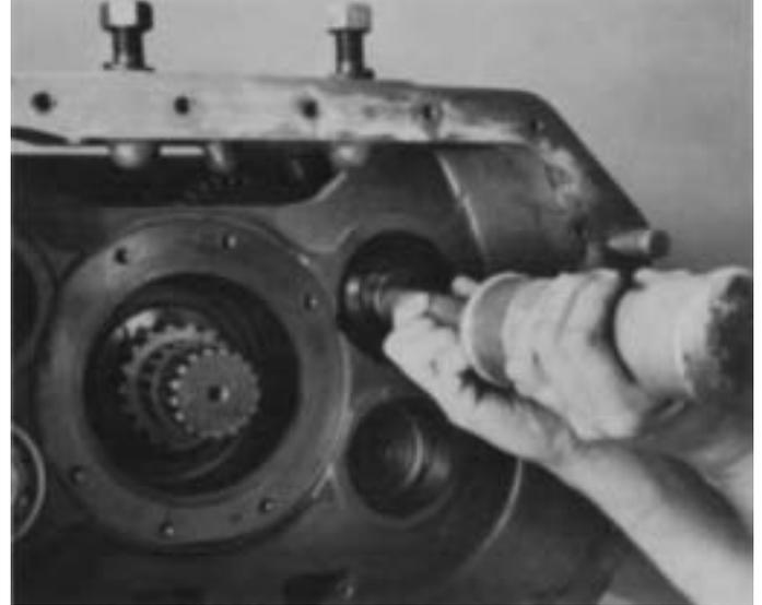
5. From the rear of case, use a soft bar and maul to drive each countershaft forward to unseat the front bearings from case bores and expose the bearing snap rings.
