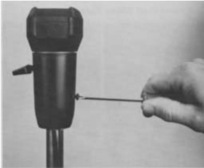
4. For models equipped with a Roadranger Valve, turn out the two mounting screws in valve cover.
