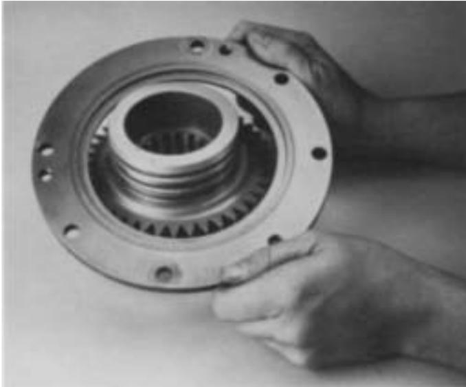
2. Install the retainer ring on auxiliary drive gear, snap ring groove facing front hub and away from gear teeth.
