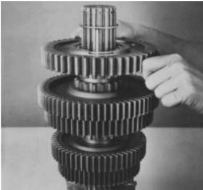
23. Install the reverse gear on mainshaft, clutching teeth down and engaged with external splines of spacer.
