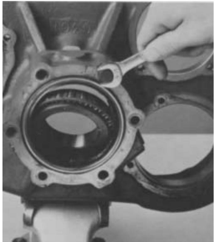
5. Remove rear bearing cover and bearing cone.
