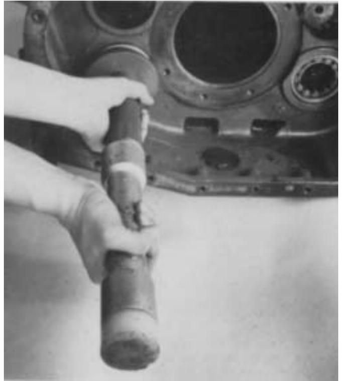
6. Remove countershaft support tool or blocking from rear case bore and install the left countershaft rear bearing with larger I.D. lead chamfer to the front of shaft and install the snap ring in groove at rear of left countershaft.
