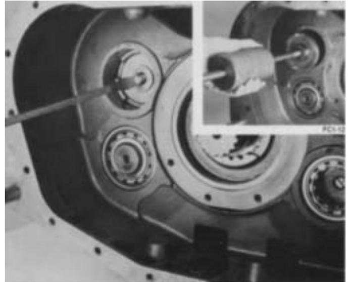
5. Remove the pipe plug from rear of idler shaft and use an impact puller, 1/2-13 threaded end, to remove shaft from case bore (inset).
