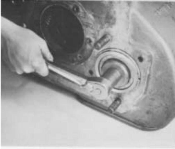
5. Position the retainer plate on front of left countershaft, roll pin in hole at end of shaft, and secure with capscrew tightening to recommended torque ratings.
