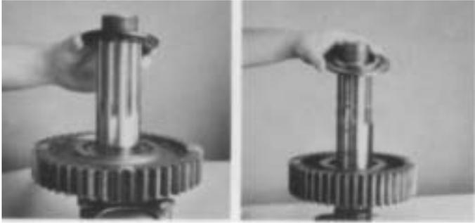
5. Install the washer on shaft against deep reduction gear, small diameter step down (Left: 11615 Models); or side with large groove up (Right: 15615 and 14615 Models).
