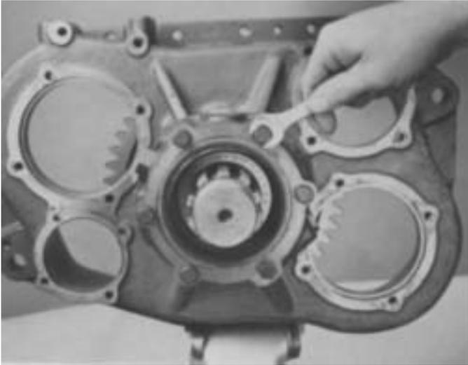
3. Temporarily reinstall rear bearing cover in position on housing **ONLY** to catch rear bearing cone released from bore in the following procedure.
