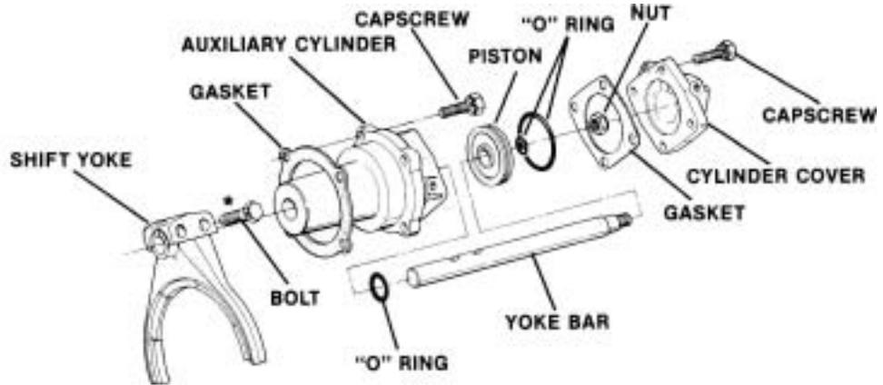
\*NOTE: Use lockwire at these positions during reassembly.
