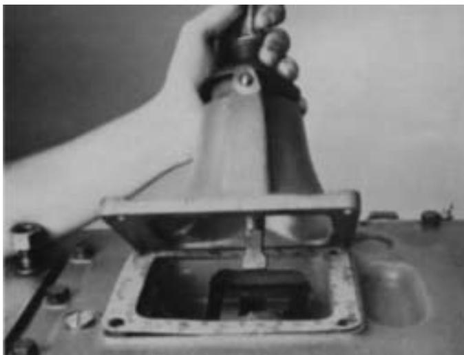
2. Install the new gear shift lever housing gasket in position on shift bar housing and install the gear shift lever housing assembly on shift bar housing, fitting the lever into shift block and yoke notches.
