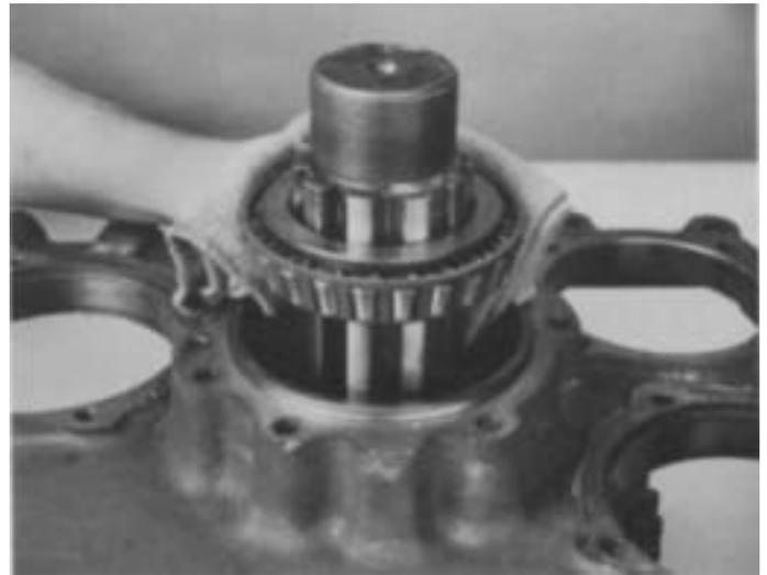
11. Install the auxiliary plate over end of output shaft assembly. Heat the rear bearing cone and install on shaft, taper down and inside bearing cup.
