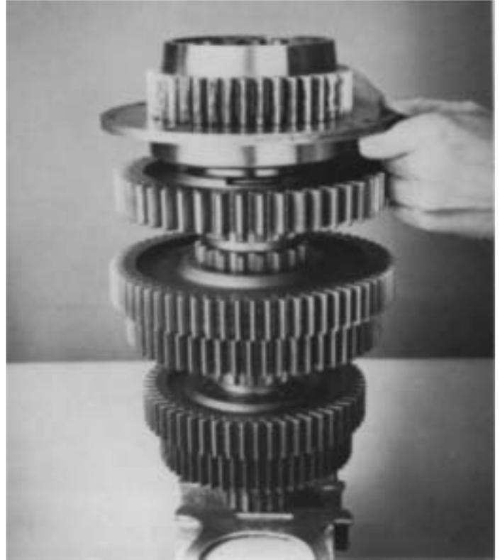
24. Install the auxiliary drive gear assembly in its proper position on rear of mainshaft.
