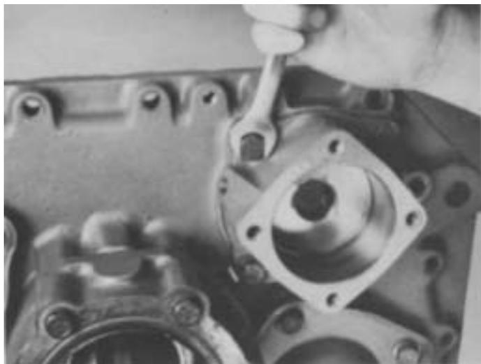
2. Position the corresponding new gasket on housing mounting surface and install the cylinder housing in rear bore of auxiliary housing, air fitting to the upper left. Tighten capscrews to secure cylinder housing to auxiliary housing.
