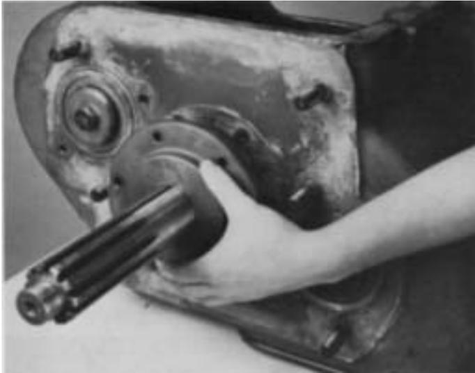
1. Turn out the retaining capscrews and remove the drivegear bearing cover and gasket.
