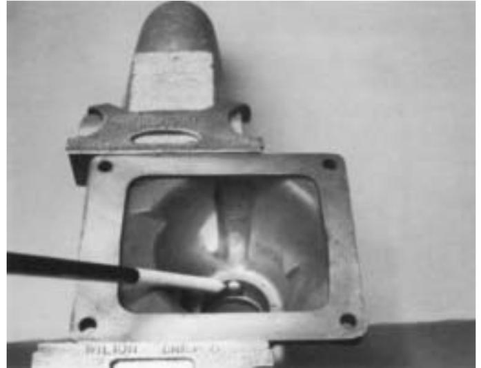
1. With the gear shift lever housing secured in vise as during disassembly, install the spade pin in bore of housing tower. If previously removed, install the O-ring in lower groove.
