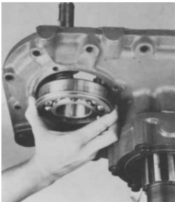
4. Remove the bearings from bores in auxiliary plate by tapping lightly and evenly to the rear with a soft bar.
