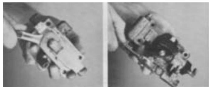
6. If necessary, remove the air line fittings from slave valve.
