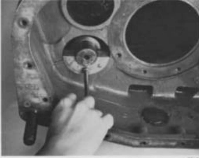
1. Move the left countershaft assembly to the rear and insert countershaft support tool or blocking to center shaft in rear case bore.
