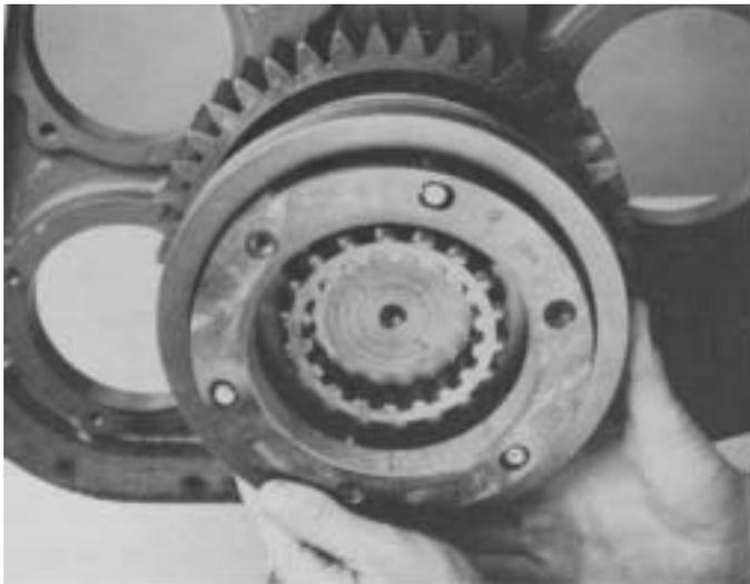
5. Install the synchronizer assembly on splines of output shaft, low range ring in recess of low range gear.
