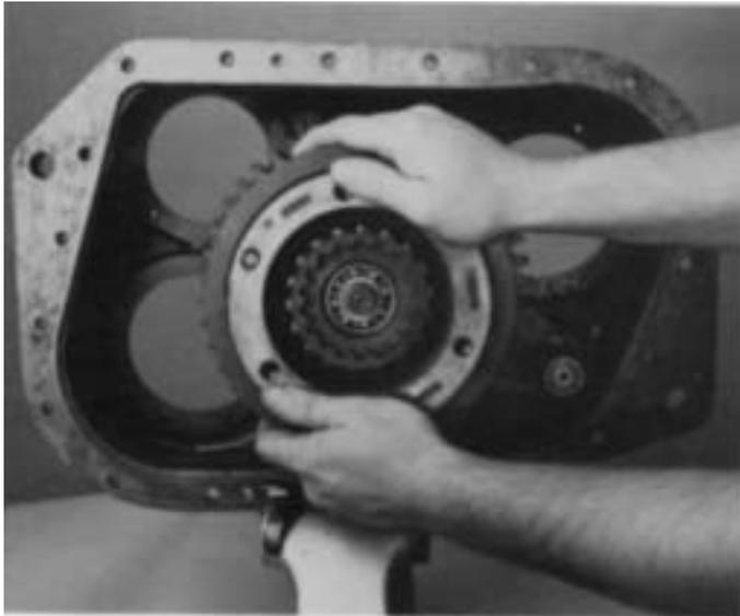
5. Install the synchronizer assembly on splines of range mainshaft, low range ring towards rear.
