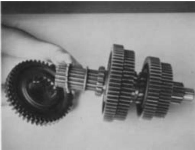
4. Remove the reverse gear and spacer from rear of mainshaft.
