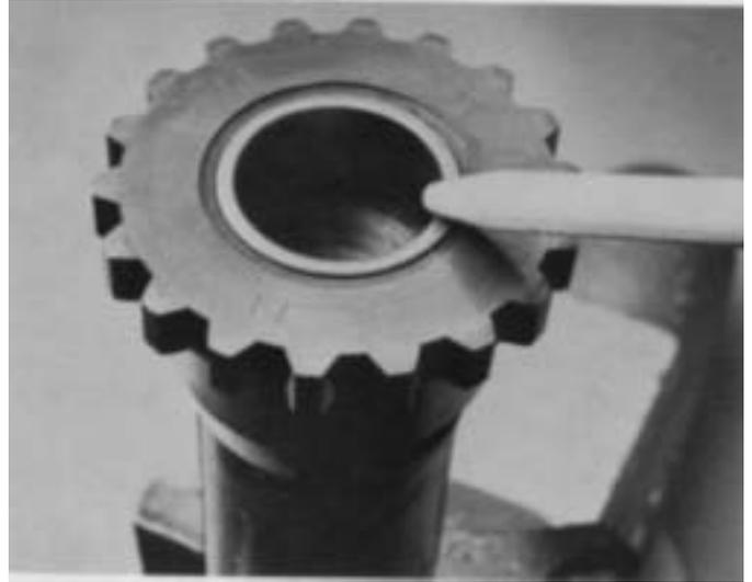
5. Check the bushing in pocket of input shaft and replace if worn or damaged.
