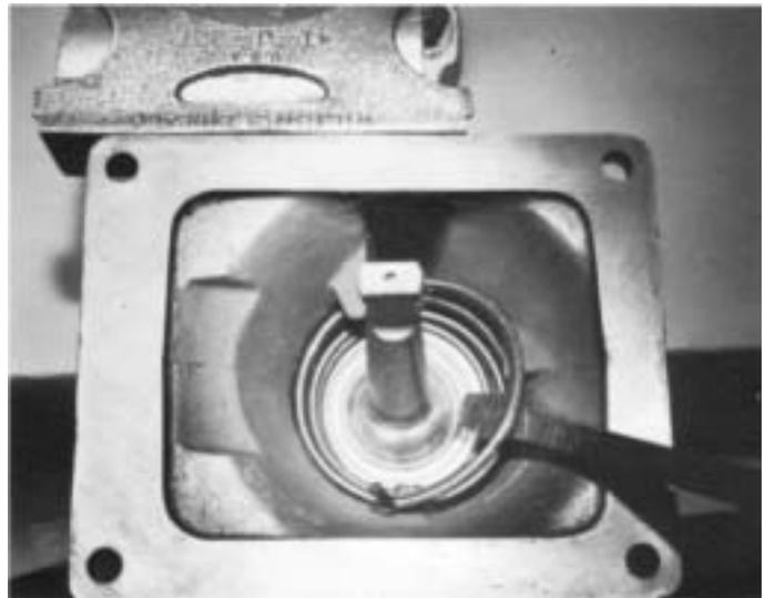
2. Remove the boot from gear shift lever and secure assembly in vise with bottom of housing up. Use a large screwdriver to twist between the spring and housing, forcing the spring from under the lugs in housing. Do one coil at a time.
