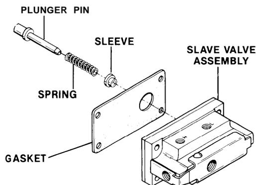
Refer to the drawing for disassembly and reassembly of the piston-type slave valve assembly. **Should the poppet-type slave valve assembly prove to be defective, replace the complete assembly, as it is non-serviceable. The actuating components used with these valve assemblies are non-interchangeable.** Failure to use the correct plunger pin, spring, and alignment sleeve during installation on the transmission will cause hard shifting in Low Range gears.
