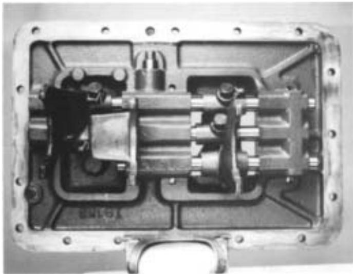
3. Secure the assembly in a vise with the plunger-side up. (The front of the housing will be to the left.) For models so equipped, cut the lockwire and turn out the retaining capscrews to remove the oil trough from the housing.
