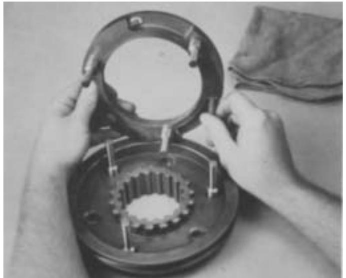
2. Install the three springs in bores of high range synchronizer ring.
