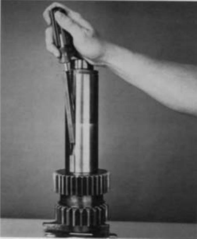
5. If necessary, remove the key and roll pin from countershaft.
