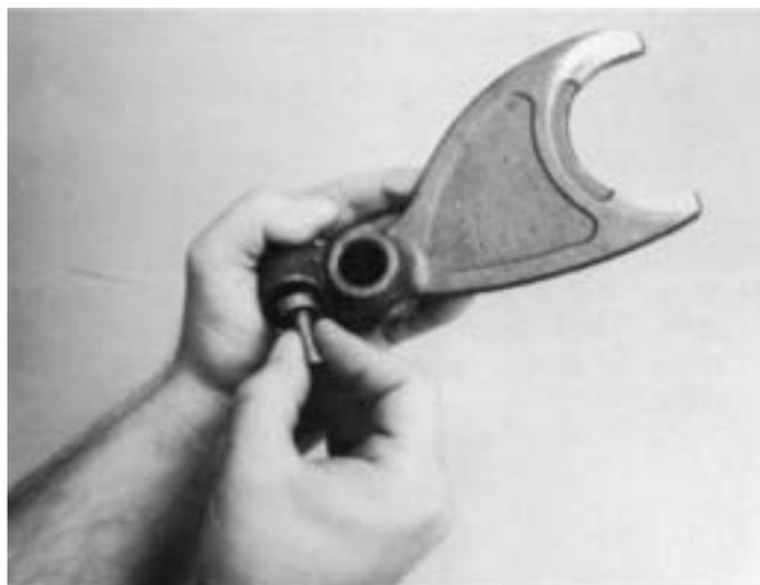
1. If previously removed, install the reverse-stop plunger in the LO-Reverse shift yoke, making sure the plunger is fully seated in the yoke slot bore.
