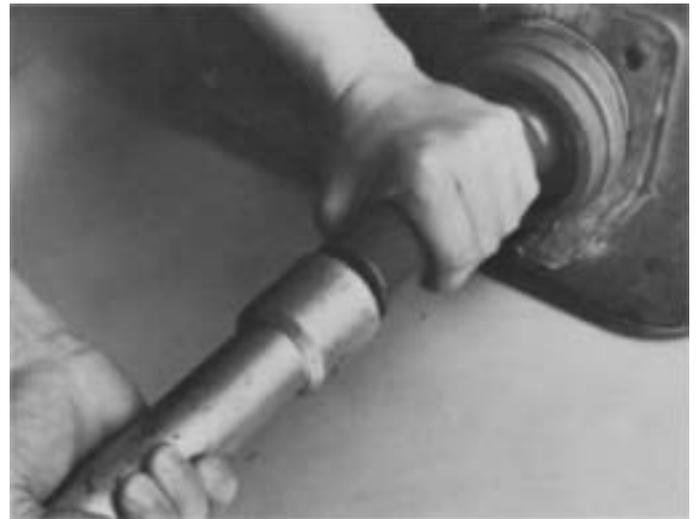
4. Use a flanged-end bearing driver to completely seat front bearing or bearing outer race in case bore.
