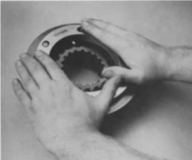
4. Apply downward pressure to the high range synchronizer ring **WHILE TWISTING COUNTER-CLOCKWISE** to compress the springs and fully seat ring on blocker pins of low range synchronizer.
