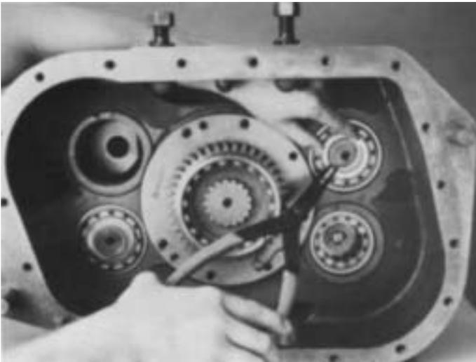
4. With bearing installation complete, install the snap ring in groove at rear of right countershaft.
