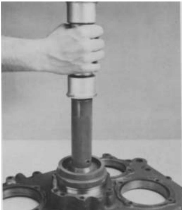
10. Place the rear bearing cup against spacer. Use a flanged-end driver to move all three parts evenly into bore until lip of rear bearing cup seats on auxiliary plate.
