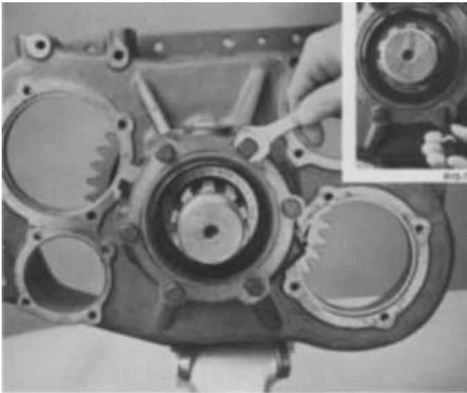
17. Position gasket on cover mounting surface and install the rear bearing cover on auxiliary housing. Use the nylon collar and brass washer with capscrew at the chamfered hole which intersects speedometer bore (inset). Tighten capscrews to secure cover to housing.
