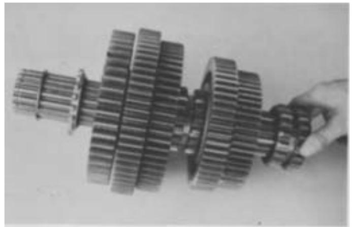
2. Remove the 4th-5th speed sliding clutch from front of mainshaft.
