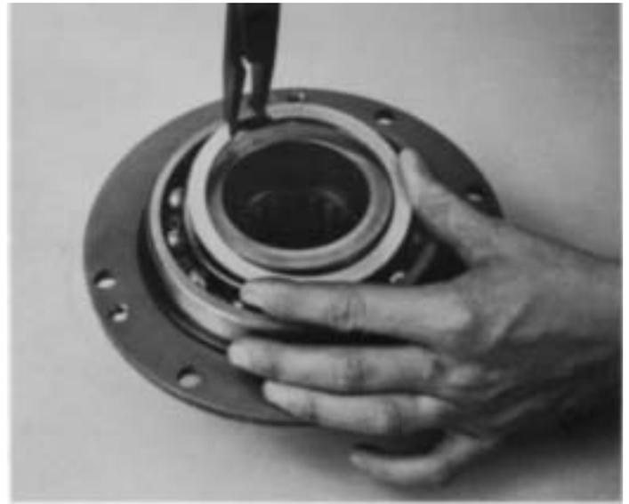
4. Install the snap ring in groove of front gear hub to retain bearing.
