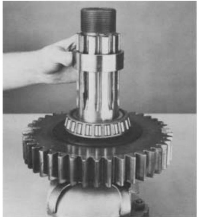
7. Install the bearing inner spacer on output shaft.
