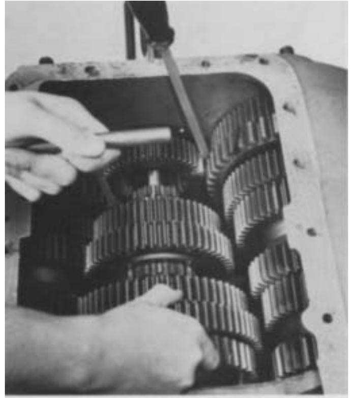
30. Move the pilot-end of mainshaft into pocket bushing of input shaft.
