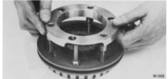
9. Place the larger low range synchronizer ring on bench.
