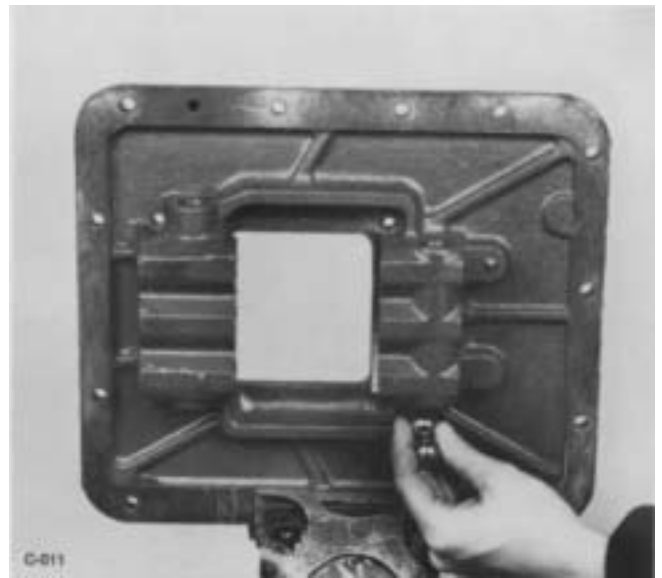
11. Remove the two interlock balls from front web.
