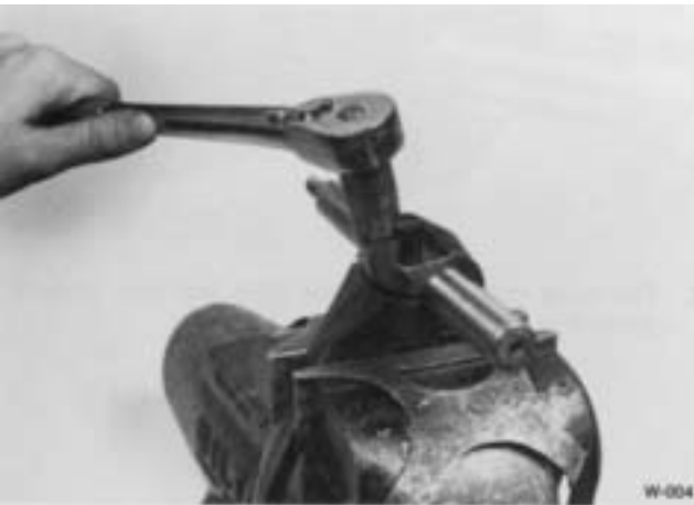
7. Remove the shaft and yoke from synchronizer assembly.
