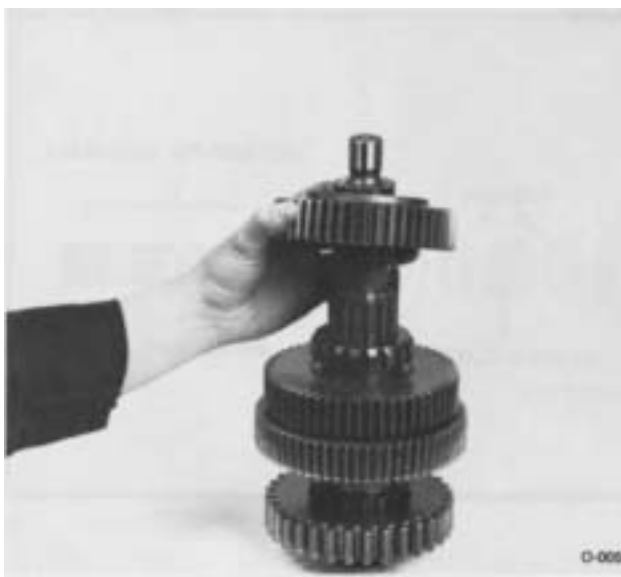
5. Remove the 3rd speed gear and washer.
