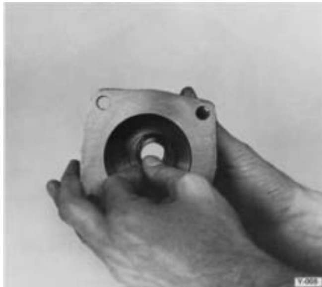
3. Remove O-ring from small bore in cylinder, if necessary.
