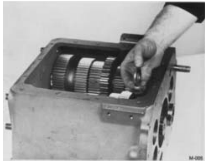
5. Remove the front idler washer from case
