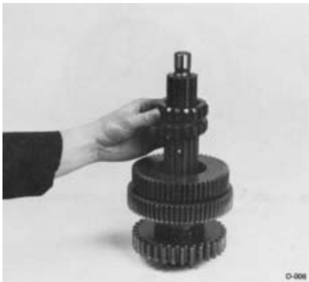
6. Remove the 2nd-3rd speed sliding clutch.
