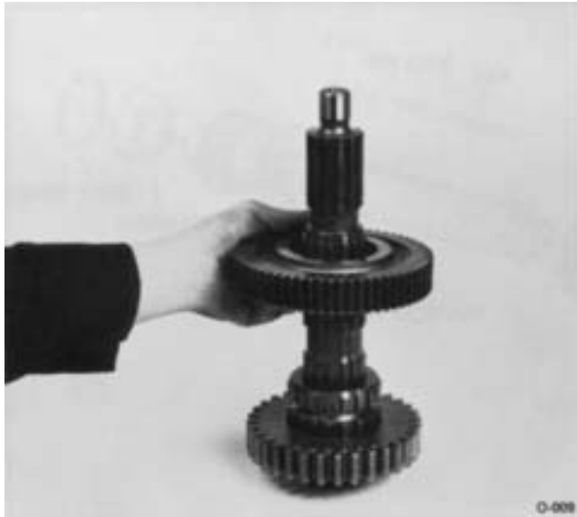
9. Remove the 1st speed gear and washer.
