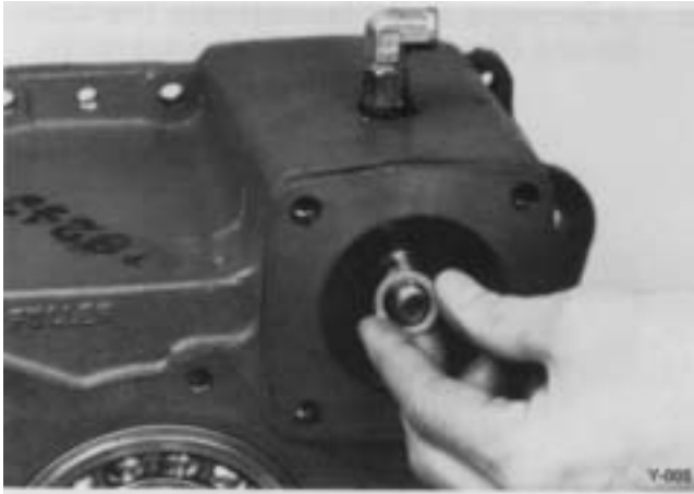
5. Remove the copper seal from shaft.
