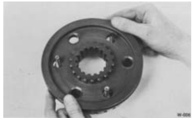
11. Remove the sliding clutch from low range synchronizer pins.
