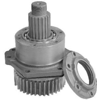
2. The capscrews holding the front bearing cap and gasket to the drive gear bearing retainer have been removed. The bearing cap has been removed from the retainer. Remove front bearing cap oil seal if it is damaged and requires replacement.
