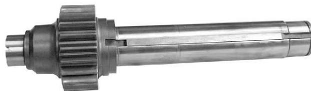
6. The Lo-Lo gear (1st speed gear) is an integral part of the countershaft and does not press off. Keys are still intact in the keyway of the counter-shaft and can be removed, if necessary.
