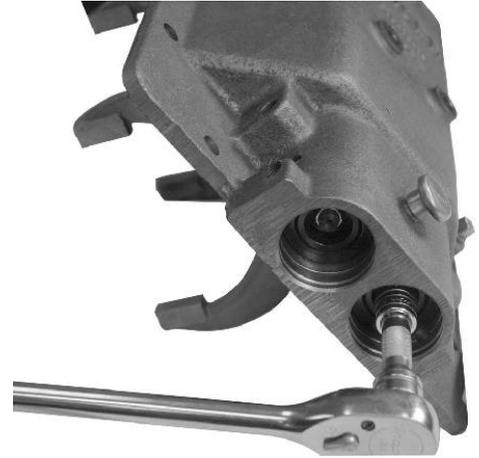
6. Also remove the locknut from the 3rd-4th piston rod.
