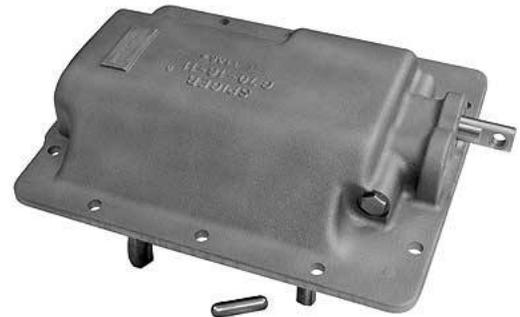
4. Drop the interlock into the interlock and poppet cross hole of the front boss. Make sure interlock seats in neutral notch of the shift rail. Secure with the poppet hole plug.
