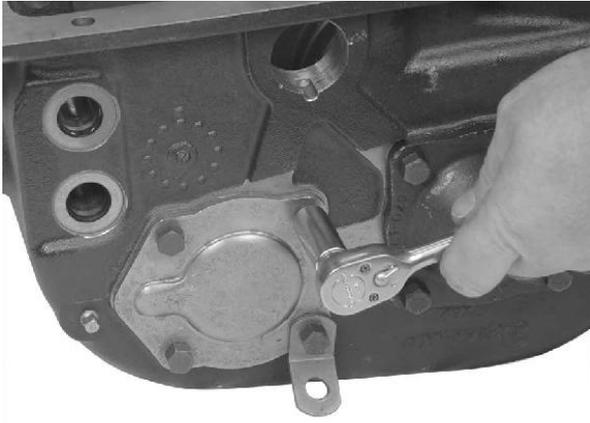
1. The four cap screws holding the reverse shaft, rear bearing cap can be removed.
