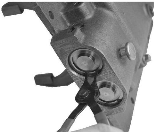
11. Place the snap ring at the front of each cylinder cap.
