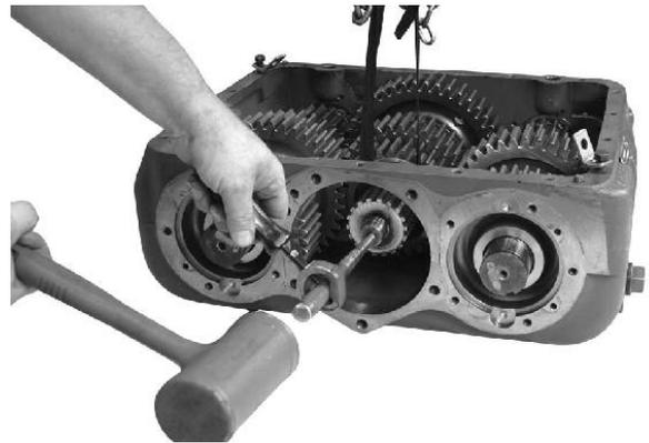
10. Here the countershaft front bearings on the right and left side have been removed. With the aid of a light chain hoist and a hook to relieve some of the weight of the mainshaft, use a soft mallet to drive the mainshaft assembly to the rear of the case.
