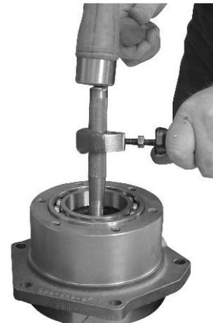
6. Use a brass drift to remove bearing from the front of the drive gear bearing retainer. The drive gear spacer can be removed from inside the retainer, at this time.
