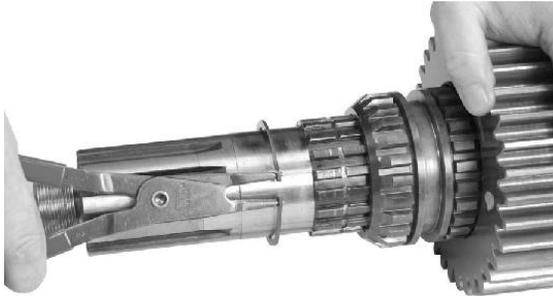
3. Remove snap ring and clutch collar from rear of the mainshaft.
