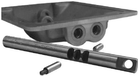
1. Install poppet spring and poppet. Assemble 3rd-4th speed shift rail is assembled to the shifter housing through the front seal and bore. The small stop sleeve and 3rd-4th speed shift forks are placed on the rail. The long hub of the fork going to the rear.
