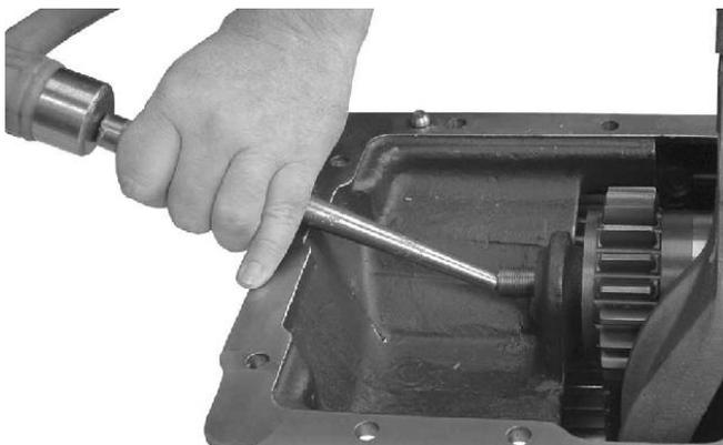
7. Use a brass punch to drive the intermediate shaft forward. Be careful no to damage the threads on the end of the shaft.
