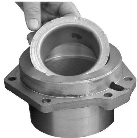
4. Place the spacer on the drive gear stem. It will rest against the drive gear rear bearing.
