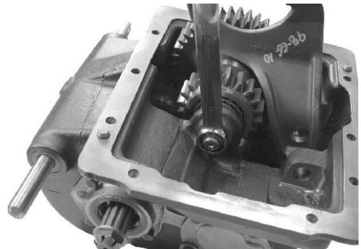
5. Pull shift rod from fork and through the front of the case.
