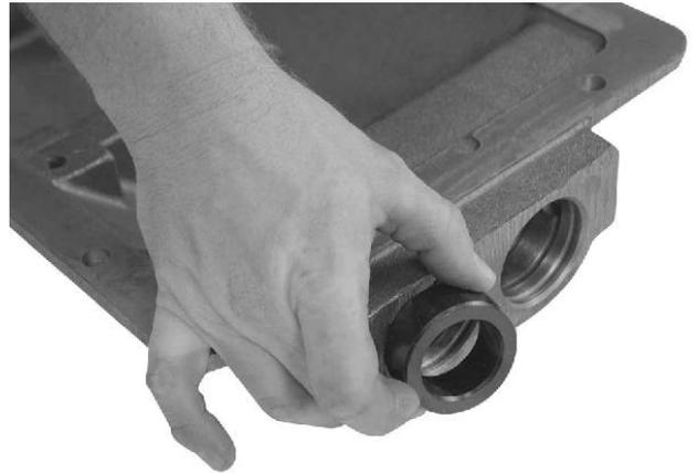
14. Remove the rear external piston from the piston housing bore. Repeat the same procedures at the adjacent piston side.
