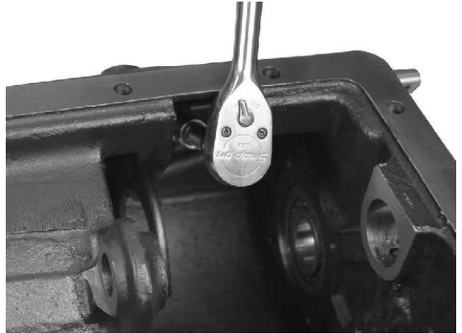
10. Remove the two cap screws holding the output sliding gear shift fork to the shift rod.
