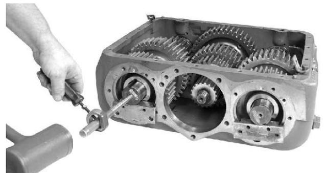
12. Drive on countershafts to move the mainshaft far enough to the rear to expose the rear bearings from the bores of the case.
