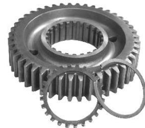
7. On the rear of the mainshaft place an internal spline and external spline thrust washer up against the 1st gear mainshaft snap ring.
