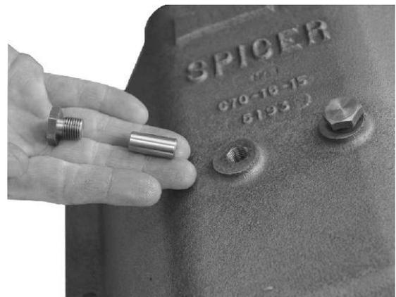
12. Place the stop pins and plugs in the top of the shifter housing. If remove reinstall air fitting to the front of the shifter.
