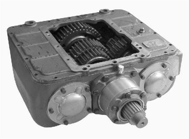
1. Shift the auxiliary into neutral. Remove the retaining capscrews holding the shifter housing to the auxiliary case. Separate the shifter housing and gasket from the case and lift straight up.
