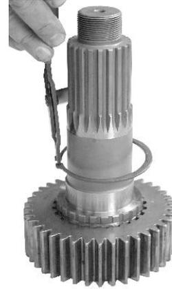
2. Install 3rd speed gear into the drive gear and install retaining snap ring.
