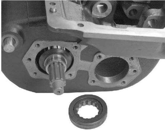
7. Place the output shaft bearing washer, with the flat side to the gear, on the rear of the output shaft. The bearing inner race goes on the shaft with the flanged end to the inside. Use a suitable driver to secure the bearing inner race to the shaft. The bearing washer will seat firmly against the shoulder of the shaft once the bearing inner race has been driven into position.
