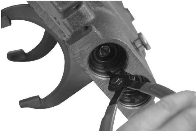
5. Remove the snap ring from inside each of the piston housing bores.
