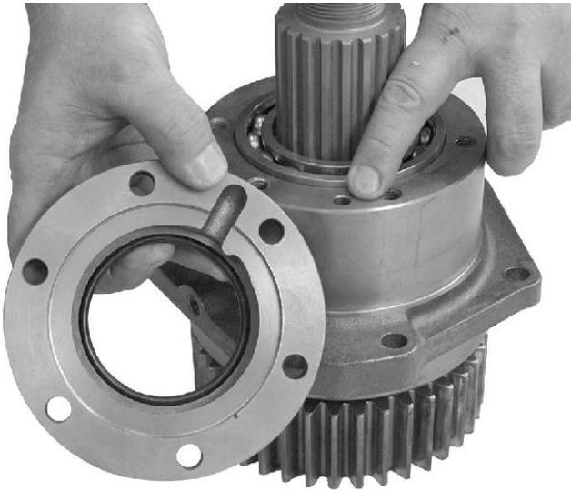
7. Install bearing retainer front cap and seal assembly. Make sure to align oil hole on cap and retainer.
