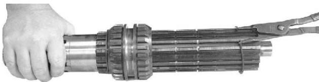
7. The 2nd speed gear snap ring to the shaft is removed. The 1st-2nd speed gear shift collar and 1st speed gear snap ring to the shaft can be taken off the mainshaft.
