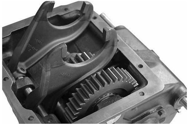
8. Align the set screw hole of the 1st-2nd shift fork to the shift rod. Secure the shift fork to the rod with the set screw. Torque the set screw to 40-50 lbs. ft.
