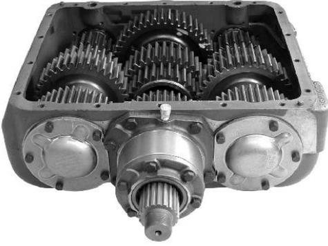
1. Lock the auxiliary in two gears by moving the two shift collars on the mainshaft forward into 2nd and 3rd gear. Use two 9/16" sockets to remove the drive gear and mainshaft end yoke locknuts and washers. Remove the drive gear and mainshaft rear end yokes. Use a puller if the end yokes will not come off readily.
