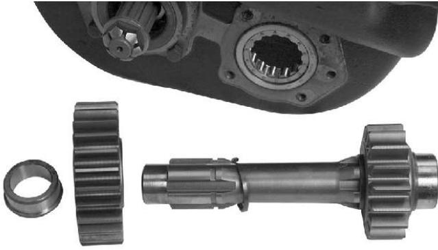
6. With the aid of a small arbor press and by supporting the gear with parallel bars, the bearing inner race can be removed from each end of the shaft. If the snap rings have been distorted, remove them from the shaft and replace with new snap rings.
