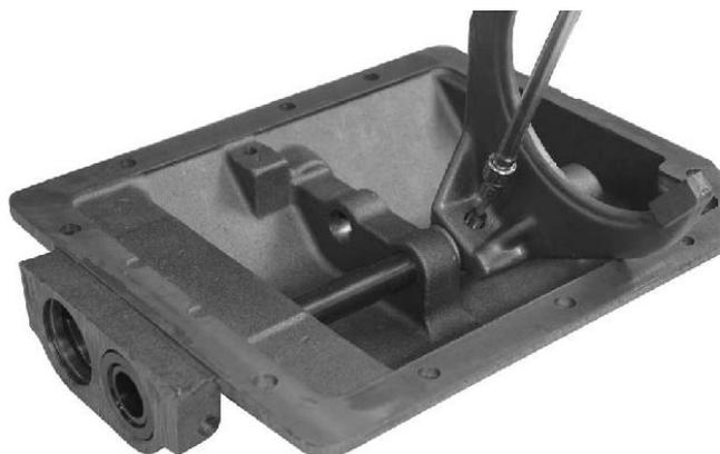
3. Secure the shift fork to the piston rod with the set screw. Torque the set screw to 40-50 lbs.ft. Use a suitable driver to drive the piston rod bushing into the piston housing bore. Flange on bushing will seat against the face inside the piston housing bore.
