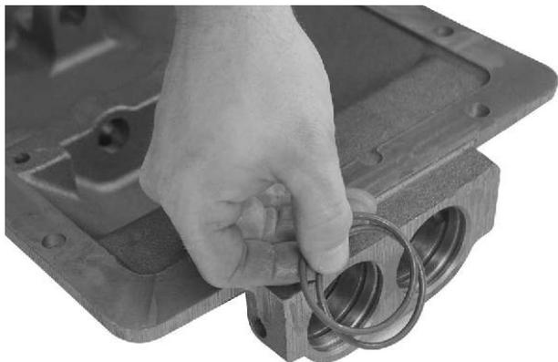
1. Inspect and replace all damaged or worn "O" rings before reassembly of the cover
