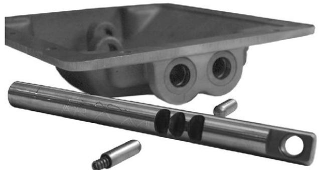
6. Remove the interlock from the interlock hole between the two shift rails. If the shift rod seals at the front of the cover are to be replaced, then remove the seals from the housing bores at this time.
