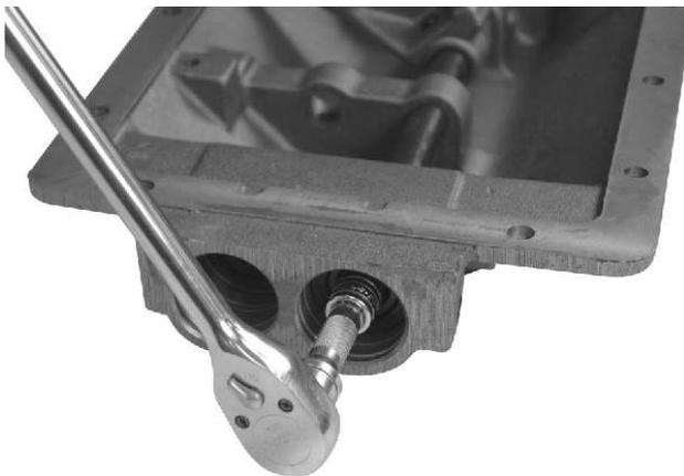
9. Remove the locknut from the 1st-2nd speed piston rod
