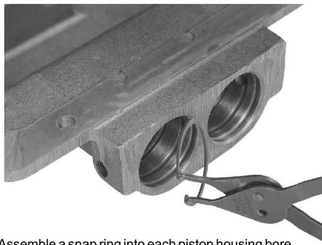
6. Assemble a snap ring into each piston housing bore.
