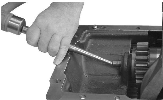
5. Slide the intermediate shaft through the front of the case and into the intermediate gear. Make sure the front bearing washer slides onto the shaft and does not drop to the bottom of the case. Drive the intermediate shaft into its final position.
