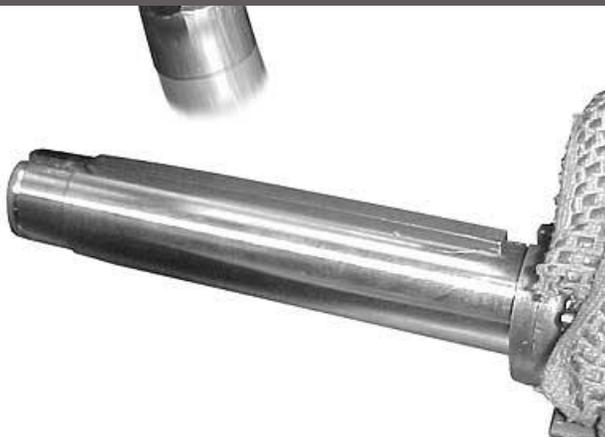
1. Secure the key into keyway of countershaft by driving on the key with a hammer. Support 2nd speed gear (underdrive) with long hub up. Align key with gear keyway and press shaft and key into gear. Seat the gear face of shaft firmly against the face of 2nd speed gear (underdrive). Key must be under the face of gear.
