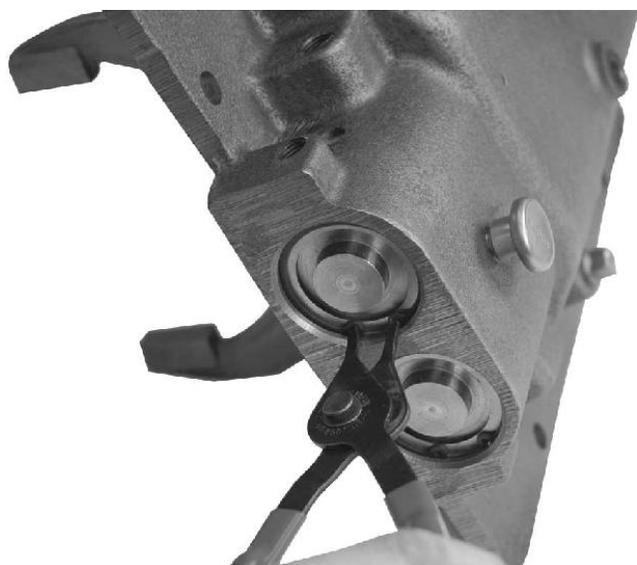
3. Remove the snap ring from in front of the piston cylinder cap.
