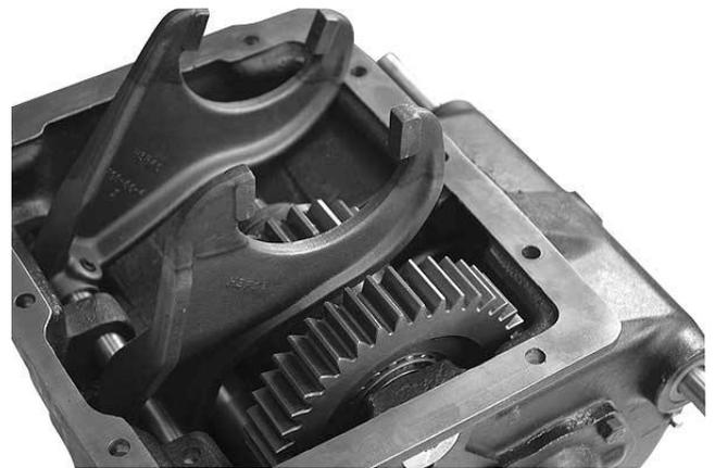
3. The retainer, poppet spring and ball is removed from the output shift rod poppet hole.
