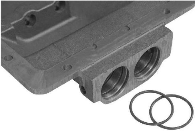
7. Assemble the front outer piston "O" ring into each piston housing bore.
