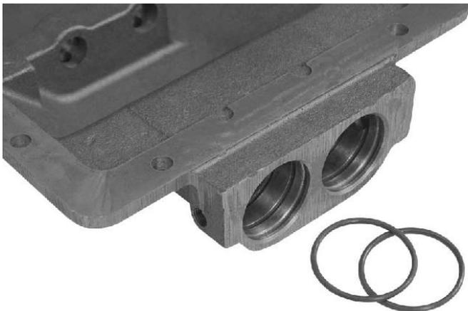
15. Remove the two external piston "O" rings in each of the piston housing bores.
