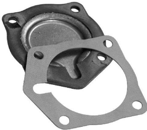
5. Align the oil return holes of the bearing cap and gasket to the oil port hole in the case.
