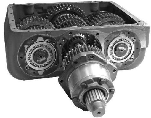
4. Drive gear bearing retainer and drive gear assembly removed.
