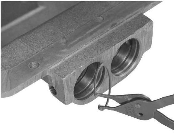
13. Remove the cylinder snap ring from the bore of the piston housing.
