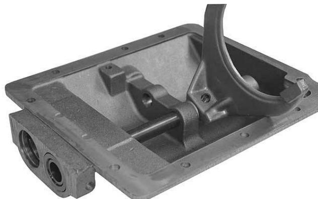
2. Place the 1st-2nd speed piston rod into the shifter housing. Place the 1st-2nd speed shift fork on the piston rod with the long hub toward the front. Place the brass internal piston rod bushing on the end of the rod. Check and make sure the interlock is still in the cross hole between the rods.
