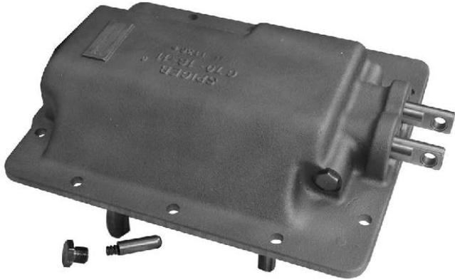
1. Remove the retainer plugs, poppet springs and poppets at the front of the shifter housing located on either side of the shift rails.
