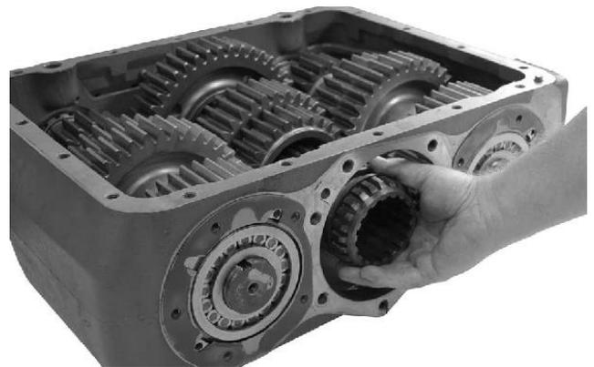
4. Leave the hoist and sling in place for support on the mainshaft in its position until the drive gear assembly and mainshaft rear bearing have been assembled into the case. Place the 3rd-4th speed shift collar on the mainshaft.
