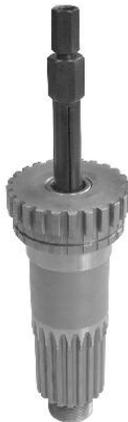
5. Remove the drive gear pocket bearing by prying out with a large screwdriver or equivalent. Use caution not to mar, or gouge pocket machined diameter with screwdriver or similar tool.
