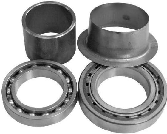
3. Install bearings and spacers into drive gear bearing retainer.
