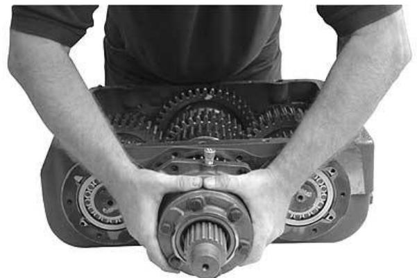
6. Install the front drive gear and bearing cap assembly with gasket into the front case bore and onto the pilot stem of the mainshaft. Torque the capscrews to 60-80 lbs. Ft.
