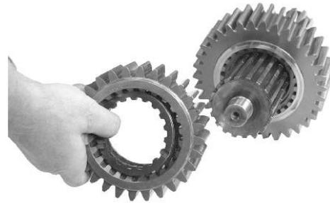
5. Place the 4th speed gear (overdrive) on the mainshaft. The snap ring is in the bore of the gear and the long spline of the gear bore faces the front of the shaft. Place an external spline thrust washer on the shaft and into the bore of the gear.
