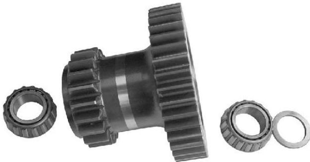
3. The intermediate gear, with the front and rear bearing cups seated in the gear bore, and the bearing cones are ready to be assembled in the case.
