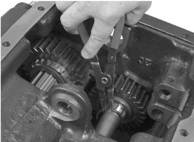
3. Remove the reverse drive gear snap ring from the snapping groove to the center of the shaft.
