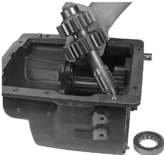
5. Lift the reverse shaft assembly up and out of the case.
