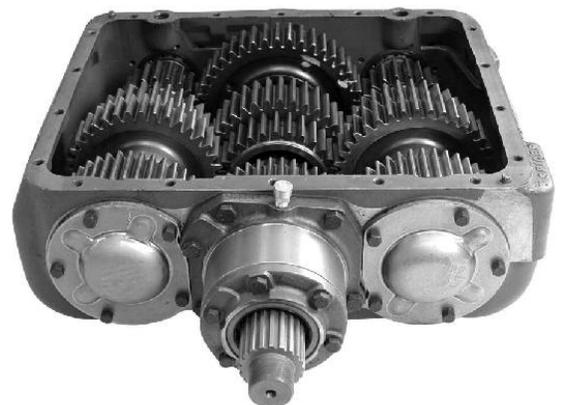
12. Install the countershaft front bearing caps with gaskets to the case face. Secure the caps with the capscrews and torque to 25-32 lbs. Ft.
