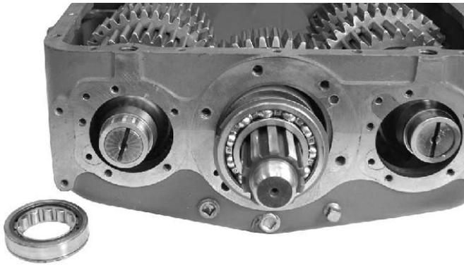
13. The rear countershaft bearings are two-piece bearings. The outer race and roller assembly can be removed from the inner race. Do not remove the inner race from the shaft unless the bearing is going to be replaced.
