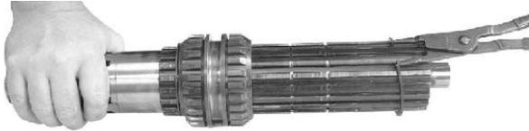
2. Install the 1st & 2nd speed clutch collar & retaining snap rings in the grooves on the mainshaft on either side of the 1st-2nd speed gear shift collar.
