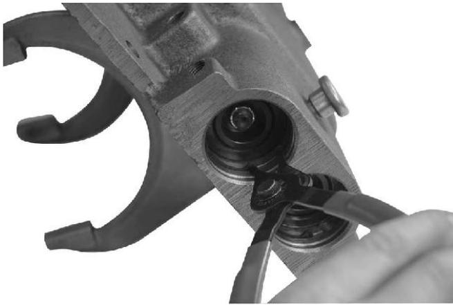
9. Assemble the snap ring to each piston housing bore.
