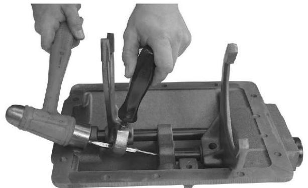
8. Use a brass drift to drive the 3rd-4th speed piston rod forward. As the rod comes forward, the internal piston can be removed from the front of the housing. The piston rod with the brass piston rod bushing can also be pulled from the front of the housing.
