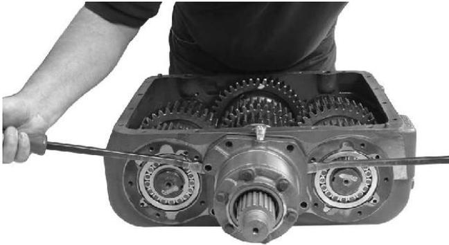
3. Remove the capscrews from the front counter shaft bearing caps. Remove the front bearing caps and gaskets. Then use a pair of pry bars, between the case and the retainer, and pry evenly until the bearing retainer and drive gear assembly is removed from the case bore.
