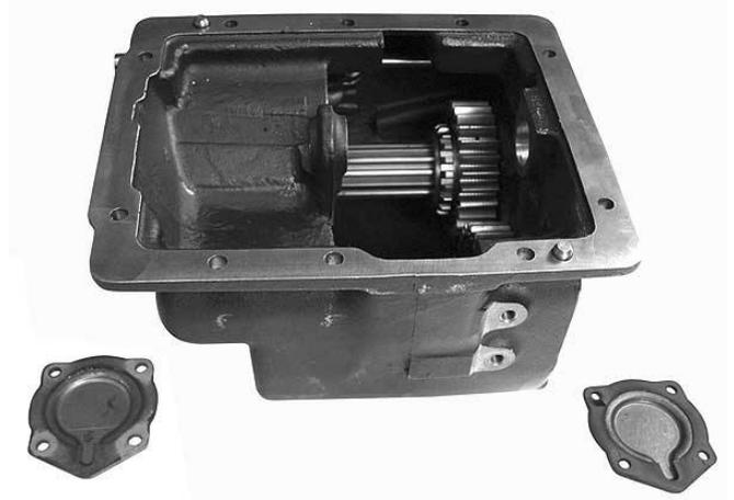
2. The reverse shaft rear bearing cap and gasket is now off the case. The four cap screws holding the reverse shaft front bearing cap can be removed.
