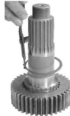
4. Use snap ring pliers to remove drive gear retaining snap ring.
