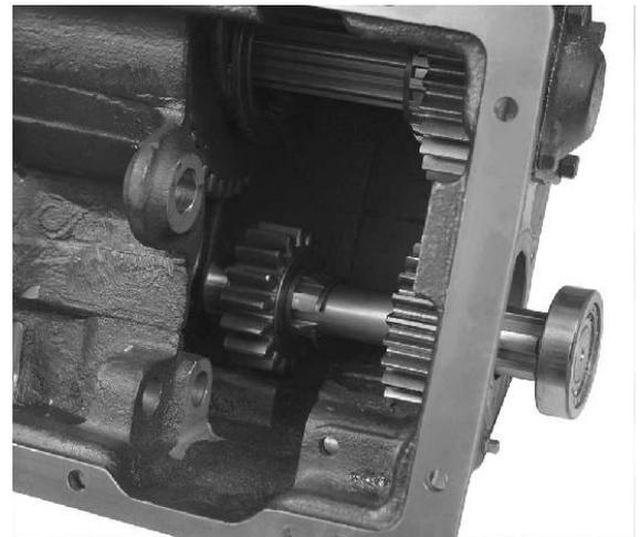
4. Move the reverse shaft forward until the outer race with cylindrical roller bearings comes out of the case bore.
