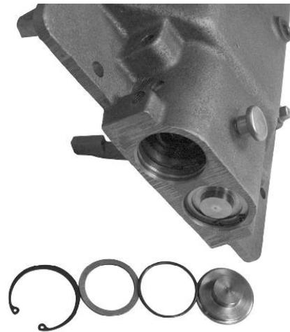
10. Assemble the cylinder caps with "O" ring and washer in each piston housing bore.
