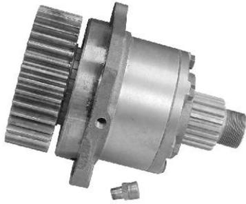
1. The drive gear front bearing cap and drive gear assembly as it was removed from the front of the case.
