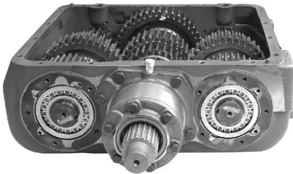
9. *Important:* With all timing gears painted, bring timing teeth of countershaft head end gears parallel to bottom of case, or pointing to the center of the case. Position drive gear timing teeth (two) where they will match and mate to the timing teeth of the countershaft gears.
