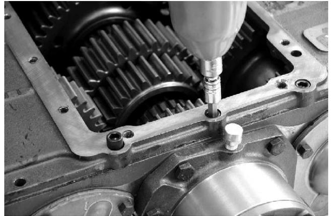
2. Remove two nuts and washers from the two rear anchor studs. Remove all retaining cap screw from adapter plate.
