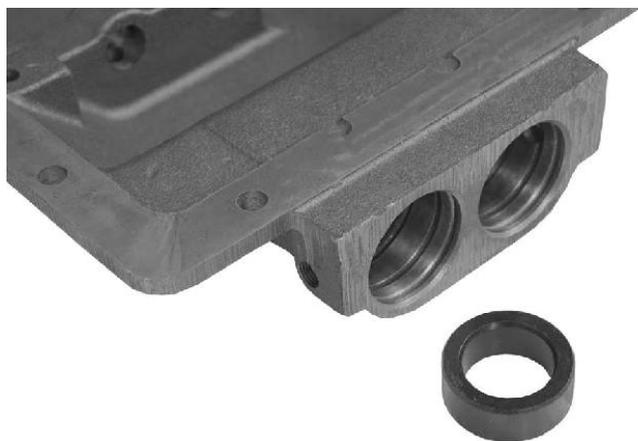
5. Place the rear outer piston into each piston housing bore.
