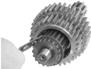
6. Place an internal spline thrust washer on the shaft and into the bore of the gear. Install the snap ring in the last groove on the mainshaft in the bore of the overdrive gear. Make certain all snap rings are seated firmly in place.
