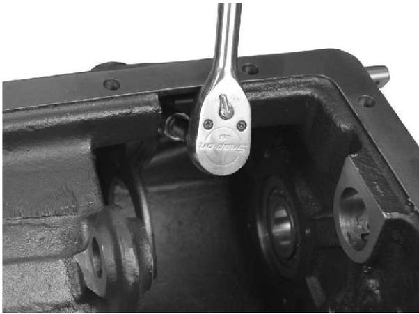
1. Assemble the output slide gear shift fork to the shift rod with the two cap screws. The spot face on the shift fork facing out. Torque the two cap screws to 40-50 lbs. ft.
