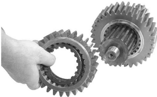
5. Remove the internal and external spline thrust washers of the overdrive gear. Remove the overdrive gear with the snap ring from the mainshaft.
