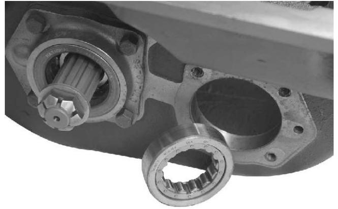
7. Use a soft hammer to tap the reverse shaft rear bearing outer race and rollers from the case bore.
