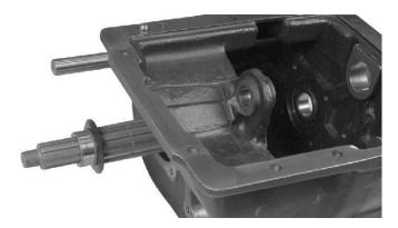
5. The two-piece bearing and bearing washer on the front of the output shaft are removed as the shaft is driven rearward.
