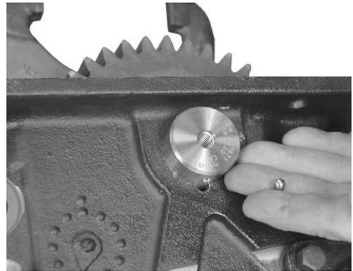
8. While driving shaft out - catch ball coming out of the front of shaft - also catch the shaft.
