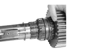
3. Remove snap ring and clutch collar from rear of the mainshaft.
