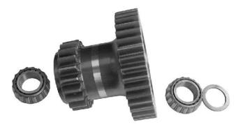
3. The intermediate gear, with the front and rear bearing cups seated in the gear bore, and the bearing cones are ready to be assembled in the case.
