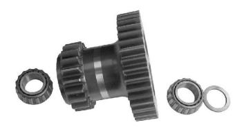
12. If the bearing cones or bearing cups are damaged and need to be replaced, use a brass drift to drive the bearing cups from the inside out of the gear bore.
