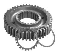
1. Remove 1st speed gear with snap ring and external spline thrust washer from the rear of the mainshaft.
