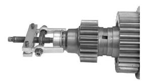
1. If the countershaft rear bearings are to be replaced, use a puller to remove the inner race off the countershaft.
