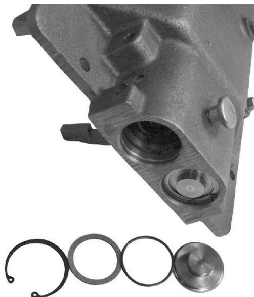
4. Remove the piston cylinder cap with "O" ring and washer. Follow the same procedure for the adjacent shift rail.
