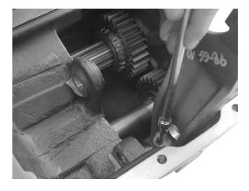
14. After removing the set screw from the transmission shift fork, slide the shift rod from the fork and out through the front of the case.
