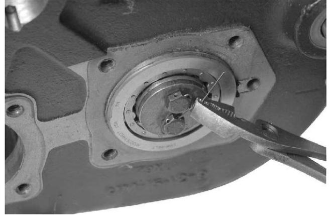
8. Secure the bearing to the shaft with the bearing retaining washer and two cap screws. Torque the cap screws to 25-32 lbs. Ft. Lockwire the two cap screws.
