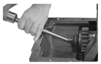
7. Use a brass punch to drive the intermediate shaft forward. Be careful no to damage the threads on the end of the shaft.
