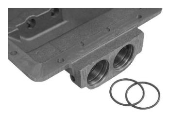
7. Assemble the front outer piston "0" ring into each piston housing bore.
