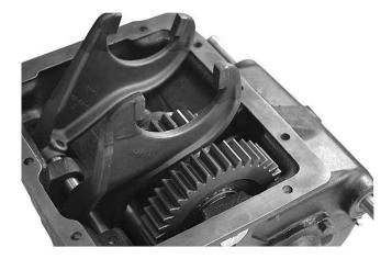
4. Remove the set screw holding the shift fork to the shift rod. Pull the shift rod from the fork and out through the front of the case.
