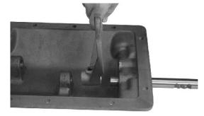
2. Slide the long stop sleeve on the shift rail behind the fork.
