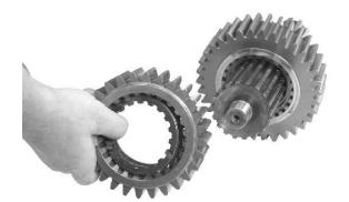
5. Remove the internal and external spline thrust washers of the overdrive gear. Remove the overdrive gear with the snap ring from the mainshaft.
