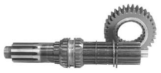
4. With the 2nd speed gear snap ring in the gear, place the 2nd speed gear on the mainshaft. The long spline in the gear bore toward the shift collar.
