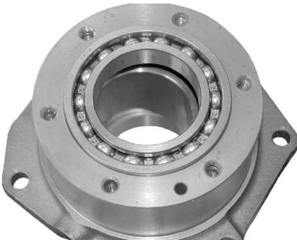
5. Bearings and spacers installed.
