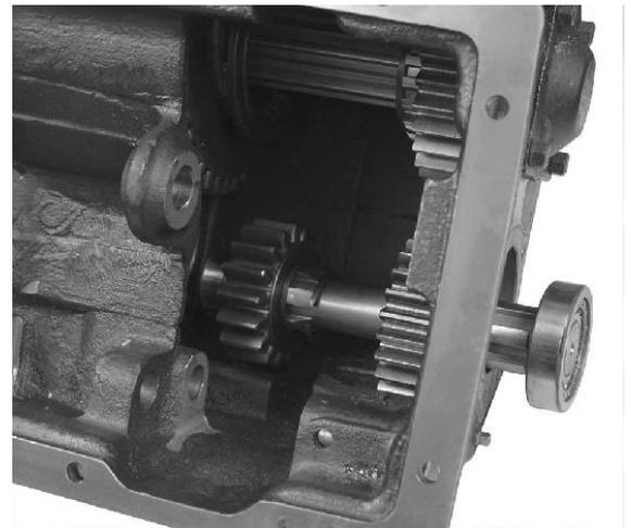
4. Move the reverse shaft forward until the outer race with cylindrical roller bearing comes out of the case bore.
