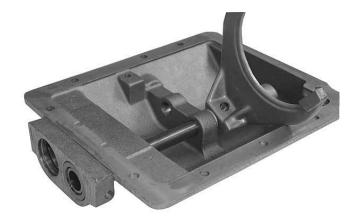
2. Place the 1st-2nd speed piston rod into the shifter housing. Place the 1st-2nd speed shift fork on the piston rod with the long hub toward the front. Place the brass internal piston rod bushing on the end of the rod. Check and make sure the interlock is still in the cross hole between the rods.
