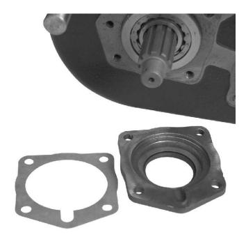
9. The output bearing cap and gasket is then removed from the case. Inspect and replace the output bearing cap oil seal if worn or damaged.
