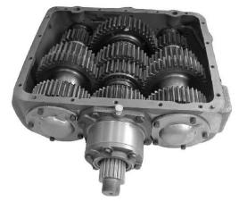
10. Install the countershaft front bearing onto the countershaft. Install the other front counter-shaft bearing in the same manner. Make certain timing marks of countershaft head end gear and drive are still in mesh.
