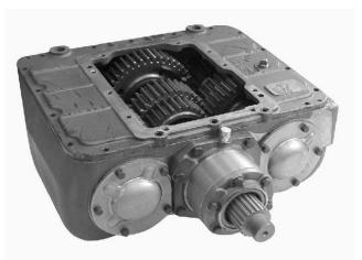
1. Shift the auxiliary into neutral. Remove the retaining capscrews holding the shifter housing to the auxiliary case. Separate the shifter housing and gasket from the case and lift straight up.
