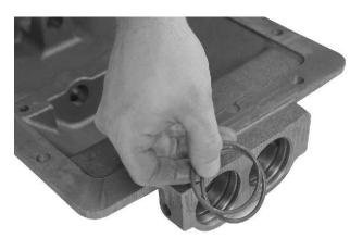
1. Inspect and replace all damaged or worn "0" rings before reassembly of the cover
