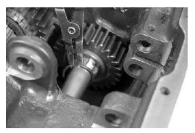
3. Place the reverse drive gear snap ring into the snap ring groove in the shaft.
