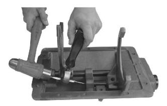
8. Use a brass drift to drive the 3rd-4th speed piston rod forward. As the rod comes forward, the internal piston can be removed from the front of the housing. The piston rod with the brass piston rod bushing can also be pulled from the front of the housing.
