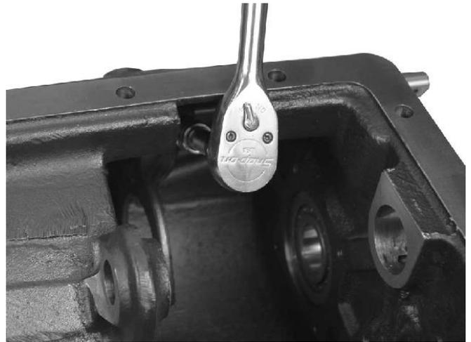
10. Remove the two cap screws holding the output sliding gear shift fork to the shift rod.
