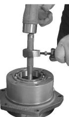
6. Use a brass drift to remove bearing from the front of the drive gear bearing retainer. The drive gear spacer can be removed from inside the retainer, at this time.
