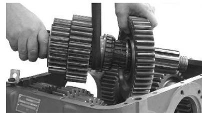
8. The 1st speed gear with the snap ring in the gear bore is placed on the shaft. The long spline in the gear bore going toward the 1st-2nd speed shift collar. Lay the mainshaft on the bench for later installation into the case.
