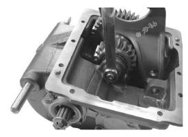
6. Remove the nut and washer from the rear of the intermediate shaft. 35
