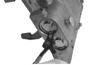
11. Place the snap ring at the front of each cylinder cap.
