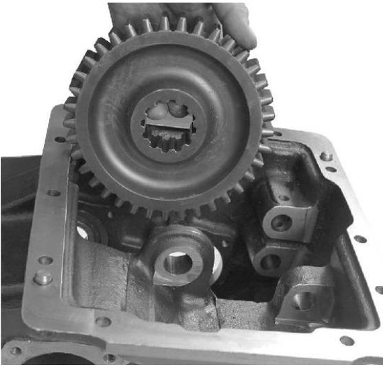
9. The output sliding gear can be lifted from the bottom of the case.
