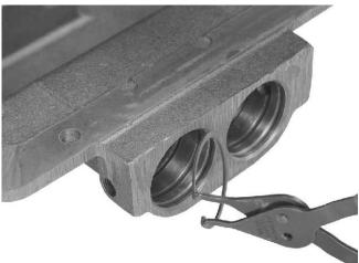
6. Assemble a snap ring into each piston housing bore.
