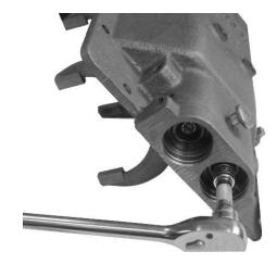
8. Place the internal piston with the front outer piston assembled to it, into the bore and onto the piston rod. Repeat the same procedure for the adjacent piston rod. Secure the internal pistons on the piston rods with the locknuts.
