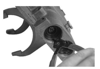
5. Remove the snap ring from inside each of the piston housing bores.
