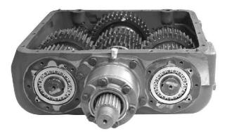
9. *Important:* With all timing gears painted, bring timing teeth of countershaft head end gears parallel to bottom of case, or pointing to the center of the case. Position drive gear timing teeth (two) where they will match and mate to the timing teeth of the countershaft gears.
