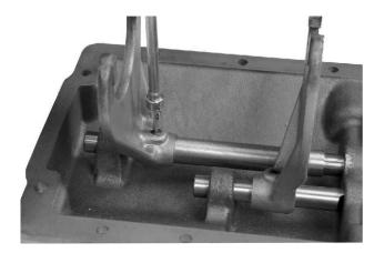
2. With the cover lying on its top on a work bench remove the set screw holding the 1st-2nd shift fork to the shift rail.
