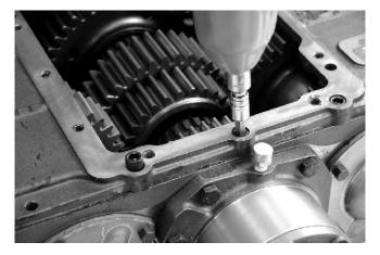
2. Remove two nuts and washers from the two rear anchor studs. Remove all retaining cap screw from adapter plate.
