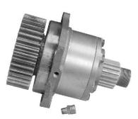
1. The drive gear front bearing cap and drive gear assembly as it was removed from the front of the case.
