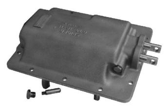
1. Remove the retainer plugs, poppet springs and poppets at the front of the shifter housing located on either side of the shift rails.
