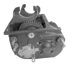
1. For disassembly, place the PTO on the bench with the forks upright. If the output yoke or flange has not been removed from the output shaft do so now.
