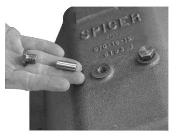
2. Remove the two retaining plugs and stop pins from the top of the shifter housing.
