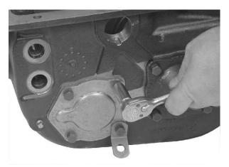
1. The four capscrews holding the reverse shaft, rear bearing capCpan be removed.
