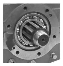
7. Use a piece of tubing or suitable driver to drive on the inner race of the mainshaft rear bearing. Seat the outer snap ring on the bearing against the main case counterbore.
