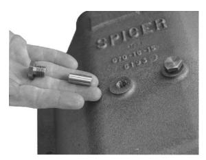
12. Place the stop pins and plugs in the top of the shifter housing. If remove reinstall air fitting to the front of the shifter.
