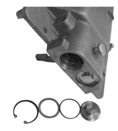
10. Assemble the cylinder caps with "0" ring and washer in each piston housing bore.
