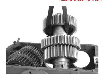
2. Install countershaft subassemblies. Try to keep the timing marks (notch) toward the center of the case. This timing mark must be mated to the drive gear timing mark later in assembly. Do not install countershaft front or rear bearings at this time.
