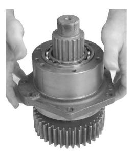
6. Install bearing retainer onto drive gear assembly.
