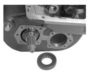
7. Place the output shaft bearing washer, with the flat side to the gear, on the rear of the output shaft. The bearing inner race goes on the shaft with the flanged end to the inside. Use a suitable driver to secure the bearing inner race to the shaft. The bearing washer will seat firmly against the shoulder of the shaft once the bearing inner race has been driven into position.
