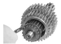
6. Place an internal spline thrust washer on the shaft and into the bore of the gear. Install the snap ring in the last groove on the mainshaft in the bore of the overdrive gear. Make certain all snap rings are seated firmly in place.
