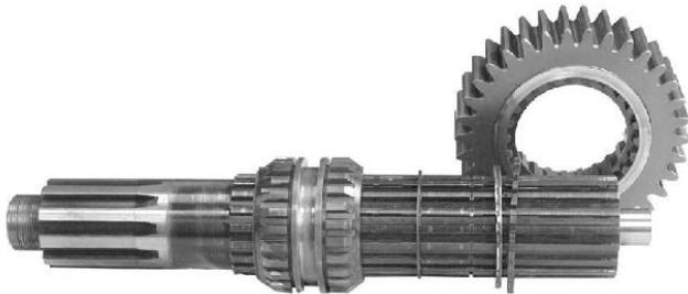
4. With the 2nd speed gear snap ring in the gear, place the 2nd speed gear on the mainshaft. The long spline in the gear bore toward the shift collar.
