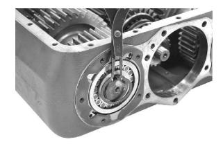
8. Use brass punch to tap on the rear of each countershaft. Tap on the countershafts until the front bearings have moved forward about 1/4 inch, enough to get the puller on the outside snap rings of the front bearings.
