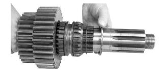
2. Remove 1st speed gear internal spline thrust washer from the rear of the mainshaft.
