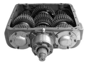
12. Install the countershaft front bearing caps with gaskets to the case face. Secure the caps with the capscrews and torque to 25-32 lbs. Ft.
