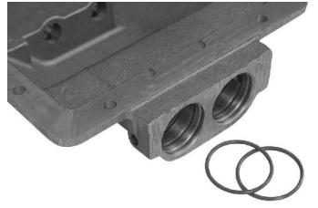
15. Remove the two external piston "0" rings in each of the piston housing bores.
