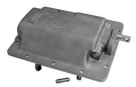
4. Drop the interlock into the interlock and poppet cross hole of the front boss. Make sure interlock seats in neutral notch of the shift rail. Secure with the poppet hole plug.
