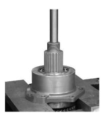
3. Support bearing retainer assembly on its flange and press drive gear free of bearing retainer, bearings and spacer.
