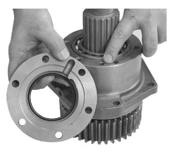
7. Install bearing retainer front cap and seal assembly. Make sure to align oil hole on cap and retainer.
