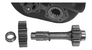
6. With the aid of a small arbor press and by supporting the gear with parallel bars, the bearing inner race can be removed from each end of the shaft. If the snap rings have been distorted, remove them from the shaft and replace with new snap rings.
