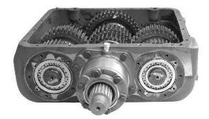
2. Remove the capscrews from the drive gear bearing retainer. Use soft hammer and tap on the retainer until it is separated from the case.
