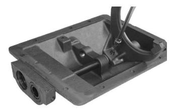
11. Remove the set screw holding the shift fork to the piston rod. Take the shift fork from the piston rod. The internal piston with the front external piston can be removed from the end of the rod. Remove the 1st-2nd speed piston rod with the piston rod brass bushing from the housing.
