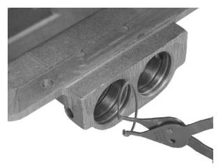
13. Remove the cylinder snap ring from the bore of the piston housing.
