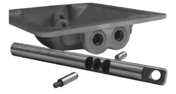
6. Remove the interlock from the interlock hole between the two shift rails. If the shift rod seals at the front of the cover are to be replaced, then remove the seals from the housing bores at this time.
