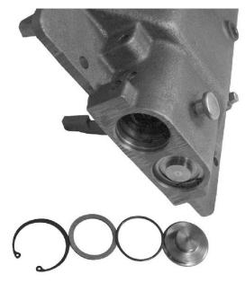
4. Remove the piston cylinder cap with "0" ring and washer. Follow the same procedure for the adjacent shift rail.
