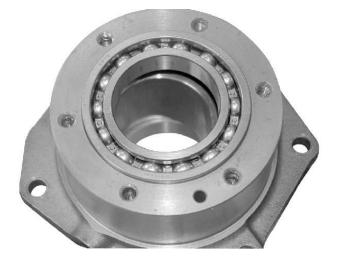
5. Bearings and spacers installed.
