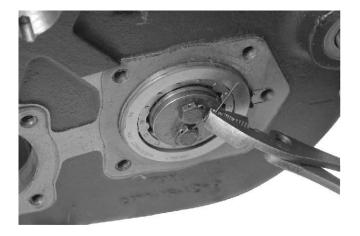
8. Secure the bearing to the shaft with the bearing retaining washer and two capscrews. Torque the capscrews to 25-32 lbs. Ft. Lockwire the two capscrews.
