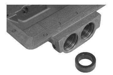
5. Place the rear outer piston into each piston housing bore.
