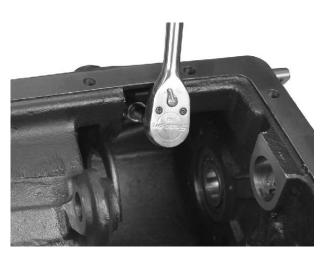
1. Assemble the output slide gear shift fork to the shift rod with the two capscrews. The spot face on the shift fork facing out. Torgue the two capscrews to 40-50 lbs. ft.
