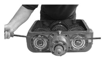
3. Remove the capscrews from the front counter shaft bearing caps. Remove the front bearing caps and gaskets. Then use a pair of pry bars, between the case and the retainer, and pry evenly until the bearing retainer and drive gear assembly is removed from the case bore.
