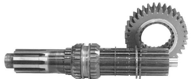
6. Remove 2nd speed gear with snap ring. The external and internal spline thrust washers of the 2nd speed gear can be removed from the shaft.
