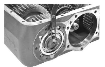
11. Install the countershaft front bearing retaining snap rings.
