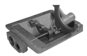
10. Use a soft mallet to drive the 1st-2nd speed piston rod forward.
