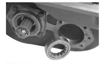
7. Use a soft hammer to tap the reverse shaft rear bearing outer race and rollers from the case bore.
