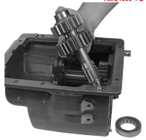
2. Lower the reverse shaft assembly into the case. The reverse gear goes to the rear of the case.
