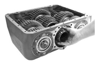
5. The 3rd-4th speed shift collar can be pulled from the mainshaft through the front of the case.
