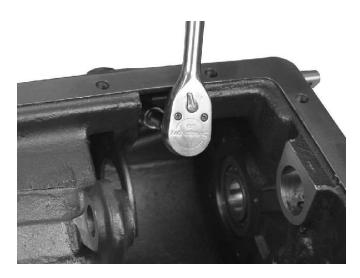
10. Remove the two capscrews holding the output sliding gear shift fork to the shift rod.
