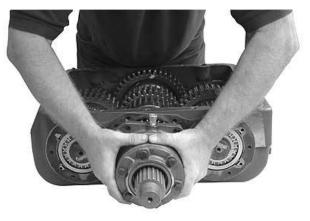
6. Install the front drive gear and bearing cap assembly with gasket into the front case bore and onto the pilot stem of the mainshaft. Torque the capscrews to 60-80 lbs. Ft.
