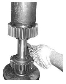
3. Secure the third key in the keyway of the countershaft. Support the 3rd speed gear (direct drive) with the long hub up. Press the shaft into the gear, seating the gear face firmly against the face of the 4th speed gear (overdrive). The key must be under the face of the gear.
