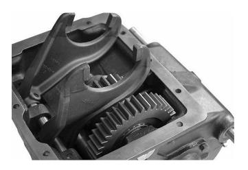
8. Align the set screw hole of the 1st-2nd shift fork to the shift rod. Secure the shift fork to the rod with the set screw. Torque the set screw to 40-50 lbs. ft.
