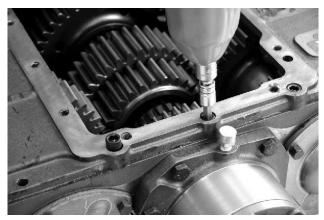
16. Install the three Allen head cap screws.
