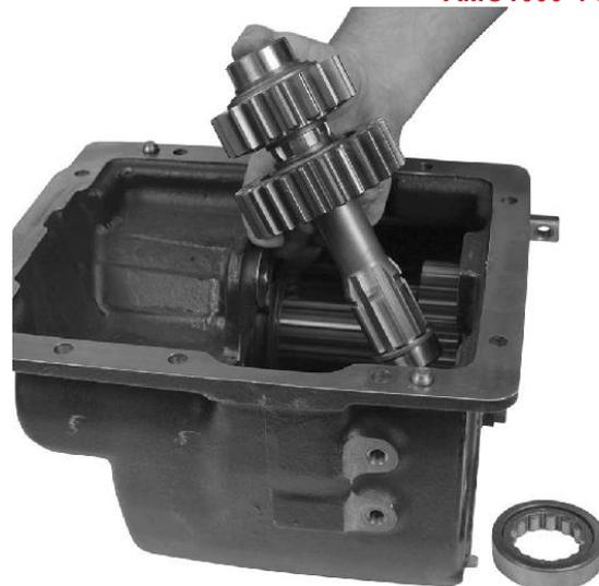
2. Lower the reverse shaft assembly into the case. The reverse gear goes to the rear of the case.
