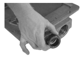
14. Remove the rear external piston from the piston housing bore. Repeat the same procedures ar the adjacent piston side.
