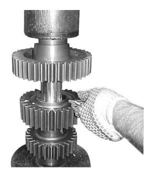
2. Secure the key for the 4th speed gear (over-drive) into the countershaft keyway. Support the overdrive gear with the long hub down. Press the shaft and key into the gear. Seat the gear face firmly against the face of the underdrive speed gear. The key must be under the face of the gear.
