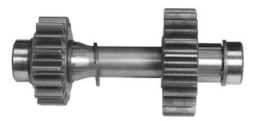
1. Assemble the reverse gear to the reverse shaft with the ground face of the gear hub facing out. Place the snap ring into position in the snap ring groove behind the reverse gear. Drive the inner race on the on the reverse shaft with the flanged end seating firmly against the reverse gear hub. Do not secure the reverse drive gear and snap ring into position on the shaft, at this time.
