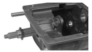
3. Slide the output shaft through the rear case bore. Align the spline of the output shaft with the splined bore of the slide gear and move the shaft on through the gear until the snap ring rests against the hub of the output slide gear. Check to make sure the sleeve pin is aligned to one of the grooves in the output shaft spline.
