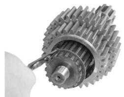
4. At the front of the mainshaft, remove the snap ring from the mainshaft groove located under the bore of the overdrive gear.
