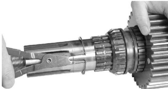
3. Remove snap ring and clutch collar from rear of the mainshaft.
