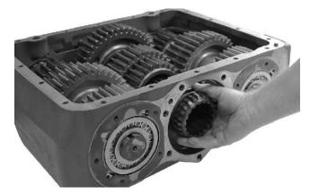
4. Leave the hoist and sling in place for support on the mainshaft in its position until the drive gear assembly and mainshaft rear bearing have been assembled into the case. Place the 3rd-4th speed shift collar on the mainshaft.
