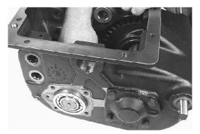
4. Use a suitable driver to secure the bearing inner race on the shaft. The flanged end seats firmly against the hub of the reverse drive gear. Align the shaft in the center of the case bore and place the outer race with cylindrical rollers on the inner race. Tap evenly on the outer bearing in the case bore. Repeat procedure for the inner race and outer cylindrical rollers at the rear of the reverse shaft.
