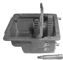
10. The shaft is removed from the intermediate gear and case.
