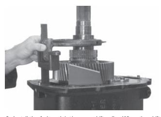
6. Install the fork and 1st/reverse shift collar. When the shift bar won't drop further, push in on the fork bars at the shift tower opening while pushing the fork bar bracket down. This will aid alignment.
