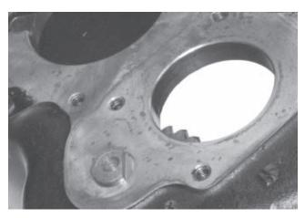
11. The straight edge on the end of the idler shaft must be positioned as shown here. Tap it into the case so the top portion of the shaft is flush with the case, or not more than .030" below the case surface. The lower portion of the idler shaft will extend about 1/4" above the case.
