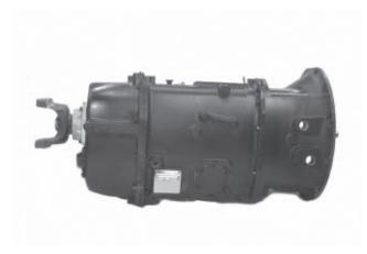
1. After removing the transmission from the vehicle, drain the oil. **Let the unit cool down first.** Otherwise, hot transmission fluid could cause burns.
