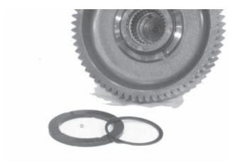
24. Remove the thrust washer and lock ball next.
