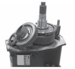
9. Next install the caged bearing and reverse gear. The gear hub should face the bearing. Also install the thrust washer, with the tapered side up.
