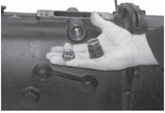
5. If the driver has experienced shifting problems, check the crossgate plunger and spring at this time. Replace them if they are worn or damaged. If no problems have occurred, it is not necessary to remove the plunger and spring.
