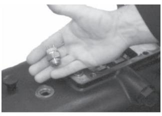
4. The backup light switch can be removed if it is going to be replaced. Otherwise, it does not have to be removed during servicing.
