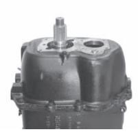
12. Coat the case sealing surface with purple Loctite 515 or the equivalent. Then install the rear case with the aid of a chain hoist. Secure with capscrews. Torque them to 25 - 41 ft. lbs. If a new 1st/reverse shift bar support was installed in the rear case, make sure the 1st/reverse bar is shifting properly.
