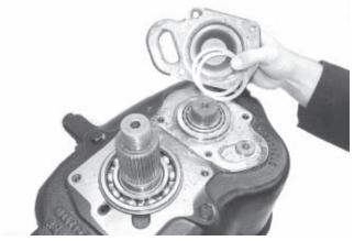
13. Coat the countershaft bearing cap with purple Loctite 515 or the equivalent. Do not put sealant in the oil groove because it could prevent proper unit lubrication.
