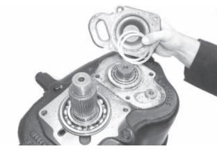
10. Remove the countershaft bearing cap and shims.
