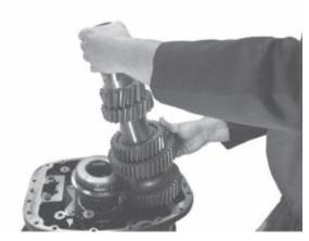
7. The countershaft is installed next. Tilting the countershaft toward the mainshaft is the easiest way to do this. Notice that there aren't any timing marks on the gears. There is no need to time the countershaft to the mainshaft.
