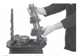
5. Tilt the countershaft and lift it from the housing.
