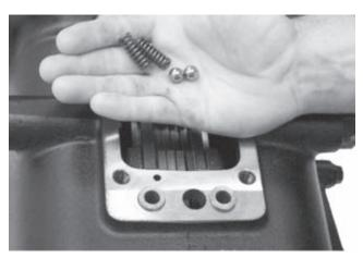
23. Install detent ball and detent springs.
