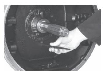
12. Use the milled slot to pry the bearing cap away from the housing.
