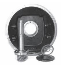
13. Remove the cap and oil baffle. Then tap the drive gear out of the clutch housing.
