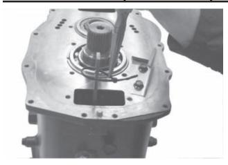
1. Remove zip tie with needle nose pliers and discard.
