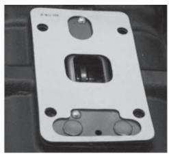
27. Install final gasket and note the position of the interlock plate. This photograph shows the correct position.
