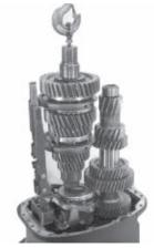
3. Lift the mainshaft from the case with the help of a hoist.
