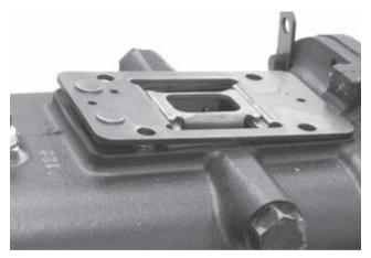
26. Install the interlock on top of interlock retaining plate. Top surface of interlock should be flush with the retaining plate.
