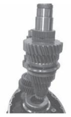
8. Oil the pocket bearing race, then slide the mainshaft assembly into place. It may be necessary to tip the countershaft away from the mainshaft to do this.
