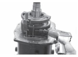
8. Attach 1st/reverse fork to shift rail and torque bolt to 21 - 45 ft. lbs.
