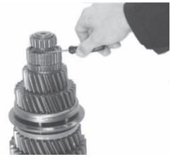
2. Remove the spiral snap ring from the groove. The easiest way to do this is to place a screwdriver under one end and work it around the snap ring.
