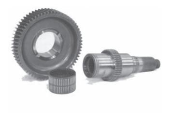
26. Remove 1st gear and the bearing from the shaft. The clutch gear is a part of the shaft.
