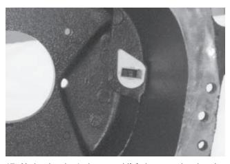
17. Notice that the 1st/reverse shift fork support bracket also stays in the housing. This bracket should not be removed unless it is broken and is going to be replaced.
