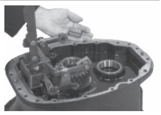
10. If the overdrive shift fork clips or the direct dirve shift fork shoes are worn, they must be removed and replaced.
