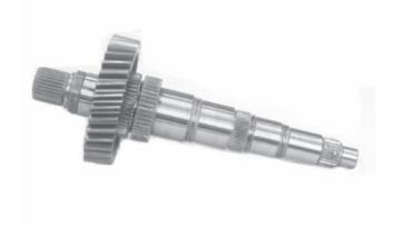
1. Lubricate all bearings with oil before beginning reassembly. Continue by placing the caged needle bearing and 2nd speed gear (hub toward clutch gear) on the shaft. Position the thrust washer on the shaft, then press the bearing race into place.
