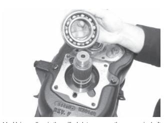
11. Using pullers in the milled slots, remove the rear mainshaft bearing.
