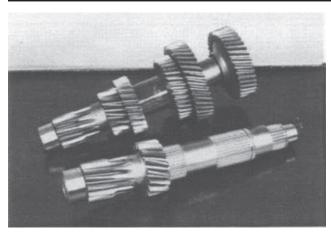
1. The countershaft gears are easily pressed off and on this shaft. The rolled involute splines provide increased torque capacity.
