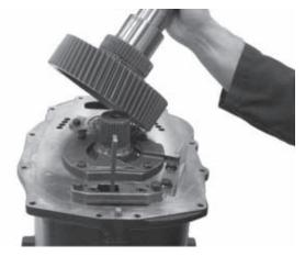
6. Use Moly #2 lubricant to coat the mainshaft splines. Then install the rear mainshaft.
