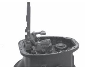
6. Install the overdrive fork if it was removed earlier. Secure it with bolts. Torque the bolts to 25 - 41 ft. lbs. If working on a direct-drive model, install the 6th/7th speed fork.
