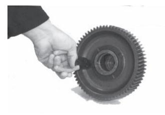
Next install the bearing and 1st gear onto the rear mainshaft.
