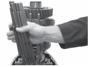
3. Remove shift rails from rail channel.
