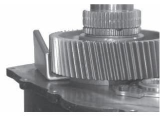
7. If the trough was removed earlier, check now to make sure there is proper clearance between it and 1st gear.
