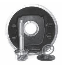
13. Remove the cap and oil baffle. Then tap the drive gear out of the clutch housing.
