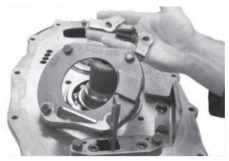
4. Install the intermediate bearing caps. The mainshaft bearing cap has a groove that lines up with the lubrication hole in the housing. Do not use gaskets or sealing compounds on either cap because it could prevent proper lubrication to the unit. Torque the cap screws to 25 - 41 ft. lbs.
