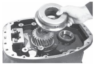
6. Next lubricate then install the 6th/7th speed synchronizer. Shift it down toward the drive gear. This will aid alignment.
