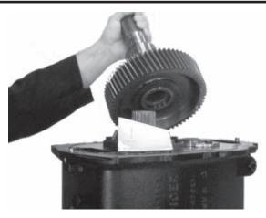
4. Use Moly #2 lubricant to coat the mainshaft splines. Then install the rear mainshaft.
