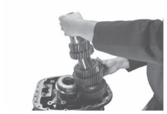
8. Remove countershaft (tilting the countershaft is the easiest way to do this).
