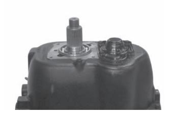
15. Secure the cap with cap screws. Torque them to 25 - 41 ft. lbs.
