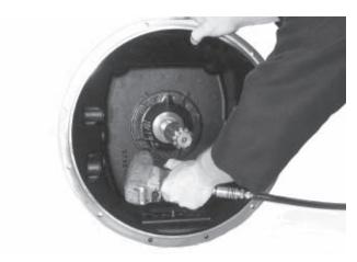
11. Next, tip the clutch housing up. Remove the four drive gear bearing cap capscrews.
