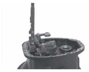
7. The overdrive fork is pictured here. It is not necessary to remove this fork, although the technician may wish to do so.
