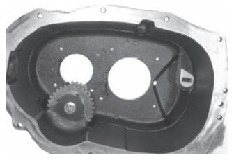
9. Assemble the bearings and gear onto the idler shaft and install the assembly. Make sure the bearings are packed with Moly #2 lubricant.
