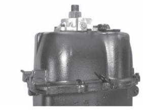
16. Secure the bearing cap with cap screws. Torque them to 25 - 41 ft. lbs.
