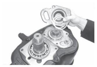
14. Coat the countershaft bearing cap with purple Loctite 515 or the equivalent. Do not put sealant in the oil groove because it could prevent proper unit lubrication.
