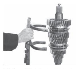
9. **Lift the mainshaft with a hoist.** While it is in the air, install 2nd/3rd and 4th/5th speed forks into place.
