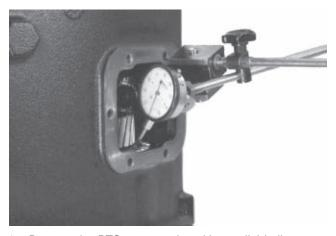
17. Remove the PTO cover and position a dial indicator as shown. Use a pry bar to lift up on a gear. End play should measure between .001"-.008". If end play is correct, replace the PTO cap and torque the cap screws to 25 - 41 ft. lbs. If end play is not correct, add or subtract shims under the rear countershaft bearing cap.
