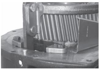
7. Secure the bracket with cap screws. Torque the cap screws to 25 - 41 ft. lbs.
