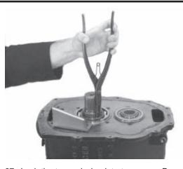
27. Lock the transmission into two gears. Remove the snap ring or mainshaft intermediate nut, depending on which component your unit contains. If your unit contains the mainshaft intermediate nut, the easiest way to remove it is to use the special socket pictured on the tool reference page.
