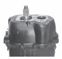
11. Coat the case sealing surface with purple Loctite 515 or the equivalent. Then install the rear case with the aid of a chain hoist. Secure with capscrews. Torque them to 25 - 41 ft. lbs. If a new 1st/reverse shift bar support was installed in the rear case, make sure the 1st/reverse bar is shifting properly.
