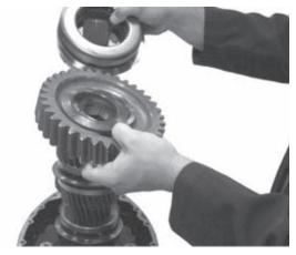
6. Remove 2nd speed gear assembly and 2nd/3rd synchronizer.
