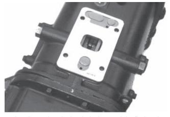
23. Install a gasket, the interlock plate, and the final gasket. Note the position of the interlock plate. This photograph shows its correct position. Next, shift into direct and install the transmission into the vehicle. Install the shift tower. Secure it with cap screws torqued to 25 - 41 ft. lbs.
