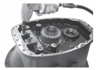
5. Place the clutch housing, drive gear face down, on the workbench and install front bar support, secure with bolts and torque to 25 - 41 ft. lbs.
