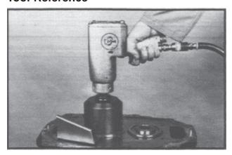
This Spicer transmission can be repaired with ordinary mechanic's tools. However, if your transmission has a mainshaft intermediate nut rather than a snap ring, vehicle downtime can be minimized with the use of this special socket. It is available through Sealed Power Corporation, part number OEM6599 To order, contact:
