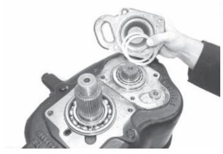
10. Remove the countershaft bearing cap and shims. Note: Some models have a rear countershaft PTO option. In this situation, the countershaft will come out with the rear case when it is removed.
