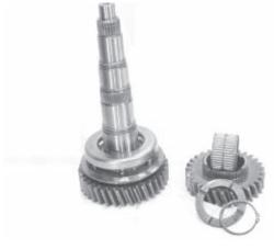
8. The snap ring, thrust washer, and lock ball can be removed. Also remove 3rd speed gear and the caged needle bearing.
