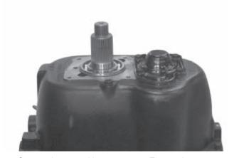
14. Secure the cap with cap screws. Torque them to 25 - 41 ft. lbs.
