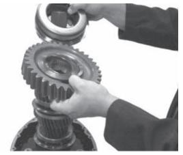
9. Lubricate the 2nd/3rd synchronizer with oil, then slide it onto the shaft. Continue by placing the caged needle bearing and 2nd speed gear (hub toward synchronizer) on the shaft. Position the thrust washer on the shaft.
