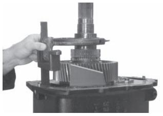
21. Unbolt the rear shift bar support bracket. Lift the 1st/reverse fork and collar assembly from the housing.
