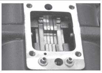
22. Check the alignment of the shift rails and shift rail channel.
