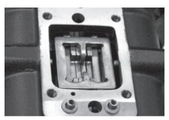
24. Install cross slide between the shift rails making sure all 4 rails are aligned in neutral and the cross slide is sitting flat.
