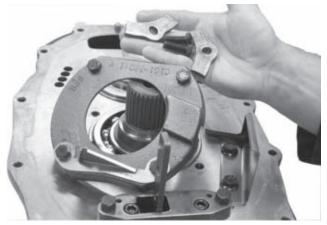
27. Continue by removing the two intermediate bearing caps. The large oil trough connected to the housing doesn't have to be removed.
