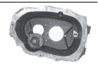
16. The reverse idler shaft and gear stay in the housing.
