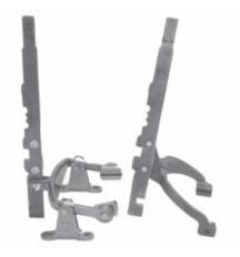
8. The direct shift fork, shown at left, also could be removed at this time.
