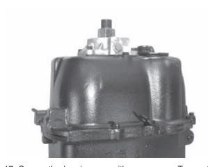
17. Secure the bearing cap with cap screws. Torque them to 25 - 41 ft. lbs.
