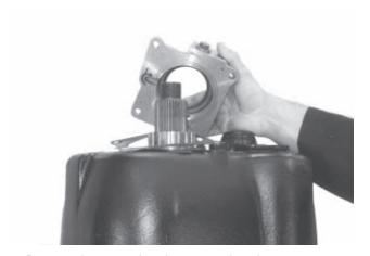
8. Remove the output bearing cap and gasket.
