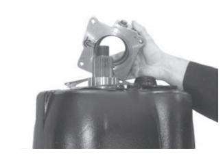
15. Install the signal gear and the mainshaft bearing cap and gasket. Make sure the bearing cap oil passage lines up with the oil passage in the transmission housing.
