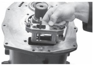
2. Slide rear support on to the end of the rail channel, secure with bolts. Torque to 21 - 45 ft. lbs.
