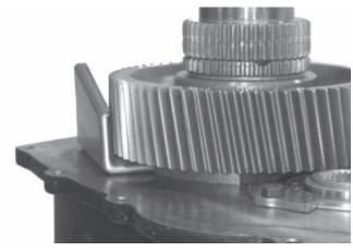
5. If the trough was removed earlier, check now to make sure there is proper clearance between it and 1st gear.
