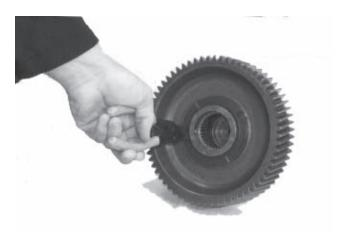
23. To remove 1st gear from the mainshaft, first remove the snap ring. Always wear safety glasses to protect your eyes when servicing transmissions.
