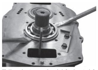
29. Use pry bars to remove the mainshaft and countershaft.
