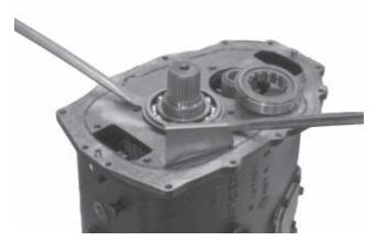
28. Use pry bars to remove the mainshaft and countershaft bearings.
