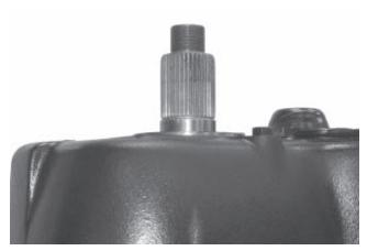
9. Next remove the speedometer signal gear.
