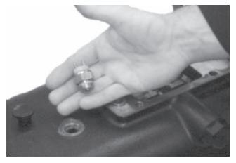
21. Install the backup light switch if it was removed earlier. Torque it to 25 - 41 ft. lbs.
