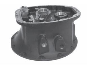
5. Place the clutch housing, drive gear face down, on the workbench.
