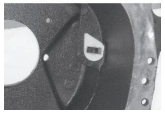
17. Notice that the 1st/reverse shift fork support bracket also stays in the housing. This bracket shoud not be removed unless it is broken and is going to be replaced.
