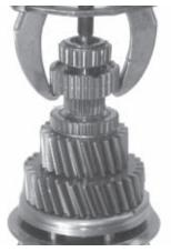
3. Attach a puller to the 6th/7th speed clutch gear. Remove the gear and the drive gear bearing together.
