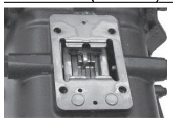
25. Install gasket and interlock retaining plate.
