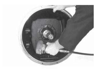
11. Next, tip the clutch housing up. Remove the four drive gear bearing cap capscrews.
