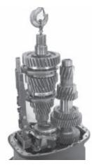
10. Oil the pocket bearing race, then slide the mainshaft assembly into place. It may be necessary to tip the countershaft away from the mainshaft to do this. Make sure the shift bars line up with the shift bar support in the case.
