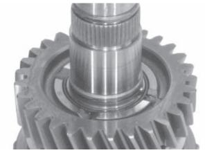
5. Note that the lock ball keeps the thrust washer form rotating on the shaft. **Wearing safety glasses**, Continue by installing the snap ring with the rounded side toward the thrust washer.
