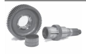
25. Remove 1st gear and the bearing from the shaft. The clutch gear is a part of the shaft.
