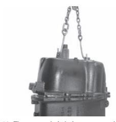
14. Then use a chain hoist to remove the rear housing.
