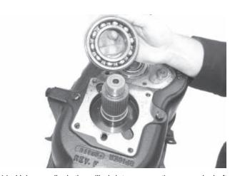
11. Using a puller in the milled slots, remove the rear mainshaft bearing.
