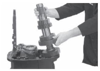
8. The countershaft is installed next. Tilting the countershaft toward the mainshaft is the easiest way to do this. Notice that there aren't any timing marks on the gears. There is no need to time the countershaft to the mainshaft.
