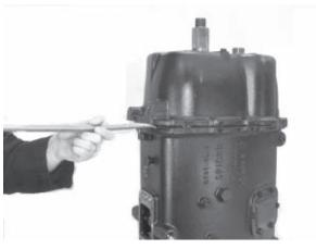
13. Next, place pry bars in the slots provided in the rear case. Break the seal.
