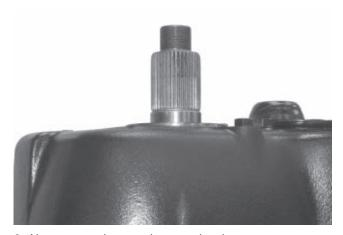
9. Next remove the speedometer signal gear.
