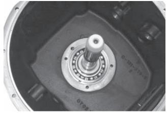
3. Place a protective sleeve over the shaft before installing the bearing cap. (See the warning on the inside front cover of this manual.) Also notice the position of the lubrication hole. The bearing cap lubrication hole must be aligned with this housing lubrication hole.
