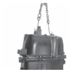
Then use a chain hoist to remove the rear housing.
