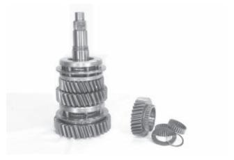
5. Remove the snap ring, thrust washer, and lock ball.
