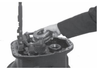
7. Next lubricate then install the 6th/7th speed synchronizer. Shift it down toward the drive gear. This will aid alignment.
