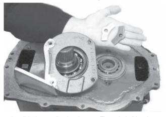
2. Install the intermediate bearing caps. The mainshaft bearing cap has a groove that lines up with the lubrication hole in the housing. Do not use gaskets or sealing compounds on either cap because it could prevent proper lubrication to the unit. Torque the cap capscrews to 25 - 41 ft. lbs.
