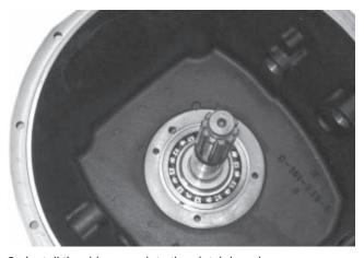
2. Install the drive gear into the clutch housing.
