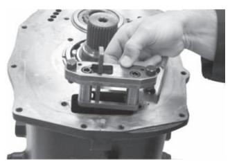
23. Remove retaining bolts and rear shift bar support.
