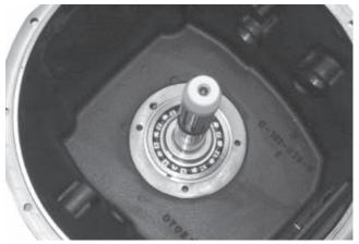
3. Place a protective sleeve over the shaft before installing the bearing cap. (See the warning on the inside of this manual.) Also notice the position of the lubrication hole. The bearing cap lubrication hole must be aligned with this housing lubrication hole.
