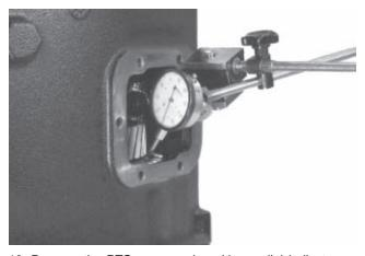
18. Remove the PTO cover and position a dial indicator as shown. Use a pry bar to lift up on a gear. End play should measure between .001"-.008". If end play is correct, replace the PTO cap and torque the cap screws to 25 - 41 ft. lbs. If end play is not correct, add or subtract shims under the rear countershaft bearing cap.
