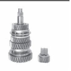
4. Next remove the overdrive gear in an overdrive unit, or 6th speed gear in a direct drive unit. There are two caged needle bearings in the gear.
