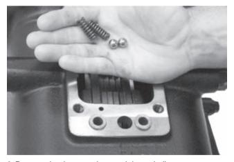
3. Remove the detent springs and detent balls.
