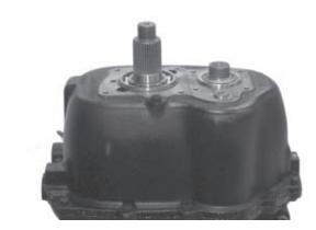
12. Next install the rear mainshaft bearing, using the proper driver to avoid bearing damage. Also install the countershaft and the countershaft bearing race.
