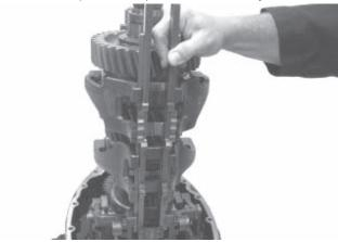
11. Install the rail channel from the top through the shift forks and down into the front bar support.
