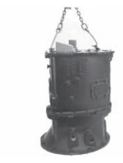
2. Begin main case disassembly by removing the housing.
