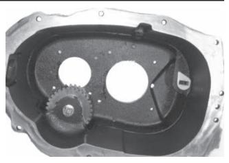
10. Assemble the bearings and gear onto the idler shaft and install the assembly. Make sure the bearings are packed with Moly #2 lubricant.
