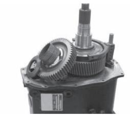
20. Continue by removing the thrust washer, reverse gear, and the caged needle bearings.
