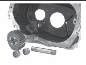
19. Remove the reverse idler gear and bearings.
