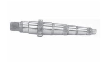
11. Disassembly of the mainshaft is complete.
