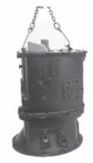
2. Begin main case disassembly by removing the housing.
