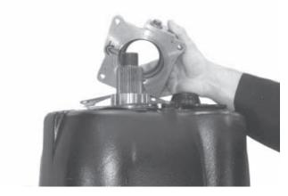
16. Install the signal gear and the mainshaft bearing cap and gasket. Make sure the bearing cap oil passage lines up with the oil passage in the transmission housing.
