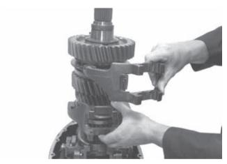
5. Remove 2nd/3rd shift fork, 4th/5th shift fork. (Overdrive models) remove shift fork assembly retaining bolts from clutch housing. (Direct models) remove 6th/7th shift fork.
