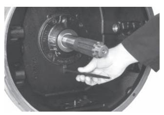
12. Use the milled slot to pry the bearing cap away fromt the housing.
