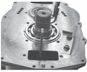
28. Lock the transmission into two gears. Remove the snap ring or mainshaft intermediate nut, depending on which component your unit contains. If your unit contains the mainshaft intermediate nut, the easiest way to remove it is to use the special socket pictured on the tool reference page.
