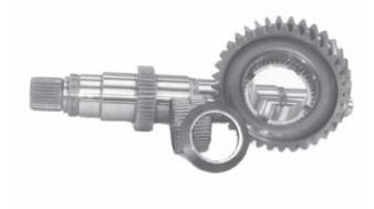
10. Then remove the thrust washer, 2nd speed gear, and the caged roller bearing.
