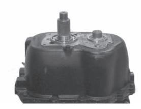
13. Next install the rear mainshaft bearing, using the proper driver to avoid bearing damage. Also install the countershaft and the countershaft bearing race.
