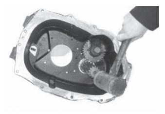
15. Using a plastic mallet, tap the rear countershaft out of the rear of the case.
