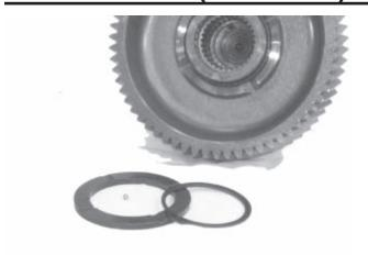
25. Remove the thrust washer and lock ball next.
