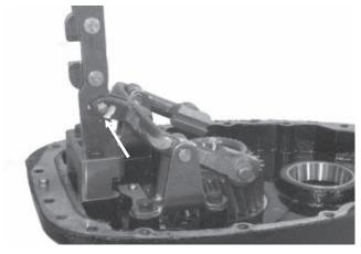
9. If the overdrive shift bar is worn, simply remove the snap ring and pin. Replace the bar, and secure it with the shift fork mounting pin and snap ring.
