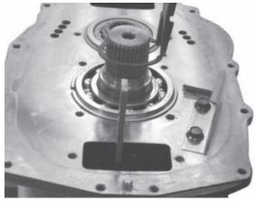
3. Install the snap rings on the intermediate bearings. Lock the transmission into two gears. If the unit is to be secured by a snap ring, lift up on 4th gear to expose the snap ring groove. Install the snap ring. If the unit is secured with a nut, install the nut on the mainshaft using the special socket listed in the tool reference. Torque the nut to 300 - 325 ft. lbs.
