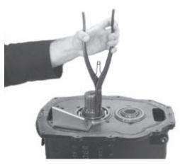
1. Install the snap rings on the intermediate bearings. Lock the transmission into two gears. If the unit is to be secured by a snap ring, lift up on 4th gear to expose the snap ring groove. Install the snap ring. If the unit is secured with a nut, install the nut on the mainshaft using the special socket listed in the tool reference. Torque the nut to 300 - 325 ft. lbs.
