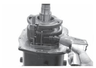
21. Remove retaining bolt from 1st/reverse shift fork. Remove 1st/reverse shift fork and collar from output shaft.
