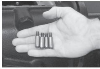
3. The four springs and plungers should be removed now. If the reason for the teardown was a shifting problem, closely examine the springs and plungers for wear or damage. Replace them if they are worn or damaged.
