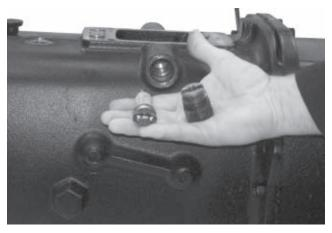
5. If the driver has experienced shifting problems, check the crossgate plunger and spring at this time. Replace them if they are worn or damaged. If no problems have occurred, it is not necessary to remove the plunger.
