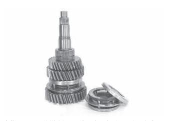
${\it 6. Remove\ the\ 4th/5th\ speed\ synchronizer\ from\ the\ shaft.}$
