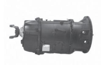
1. After removing the transmission from the vehicle, drain the oil. Let the unit cool down first. Otherwise, hot transmission fluid could cause burns.
