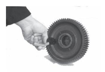
24. To remove 1st gear from the mainshaft, first remove the snap ring. Always wear safety glasses to protect your eyes when servicing transmissions.
