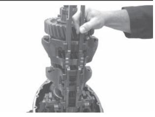
4. Remove rail channel from shift forks and front bar support.
