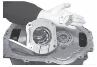
26. Continue by removing the two intermediate bearing caps. The large oil trough connected to the housing doesn't have to be removed.
