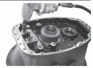
10. Remove retaining bolts and front shift bar support.
