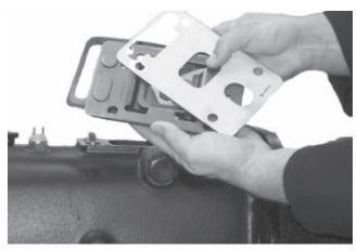
2. Remove the interlock retaining drive screws. Next remove the gaskets and interlock retainer plate.
