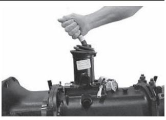
28. Temporarily install the shift tower and bench shift the unit to make sure all forks are shifting properly. Before removing shift tower assembly, shift the transmission into direct gear. This will aid in the installation of transmission into the vehicle.
