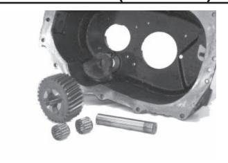
19. Remove the reverse idler gear and bearings.
