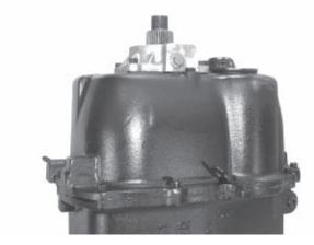
7. Remove the nut, washer, and end yoke or flange.
