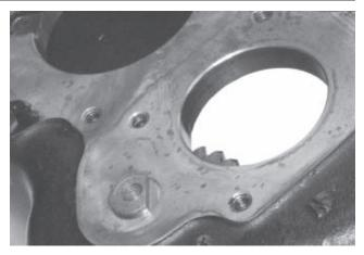
10. The straight edge on the end of the idler shaft must be positioned as shown here. Tap it into the case so the top portion of the shaft is flush with the case, or not more than .030" below the case surface. The lower portion of the idler shaft will extend about 1/4" above the case.
