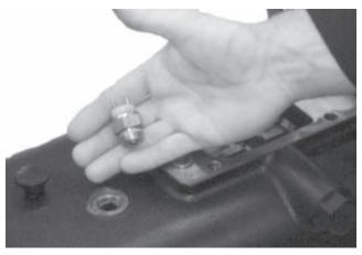
20. Install the backup light switch if it was removed earlier. Torque it to 25 - 41 ft. lbs.
