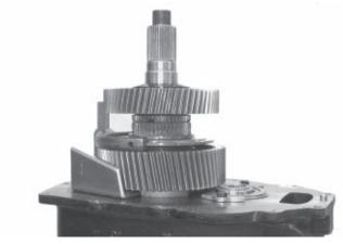
8. Next install the caged bearing and reverse gear. The gear hub should face the bearing. Also install the thrust washer, with the tapered side up.
