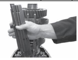
13. Slide the shift rails into the front bar support and in place between the rail channel. When properly installed in the rail-channel, the tabs on the bottom of the shift rails will line up with the appropriate shift fork. Also, there are indentations on rails 2/3, 4/5, and 6/7. If the rails are installed properly, the indentations will descend from left to right. After insuring proper installation, temporarily secure shift rails with a zip tie.
