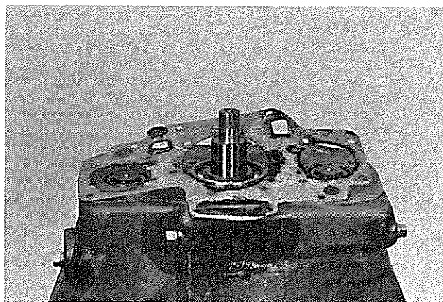
16. Remove gasket. This completes the disassembly of the rear section. Place the transmission on a bench for front section disassembly.
