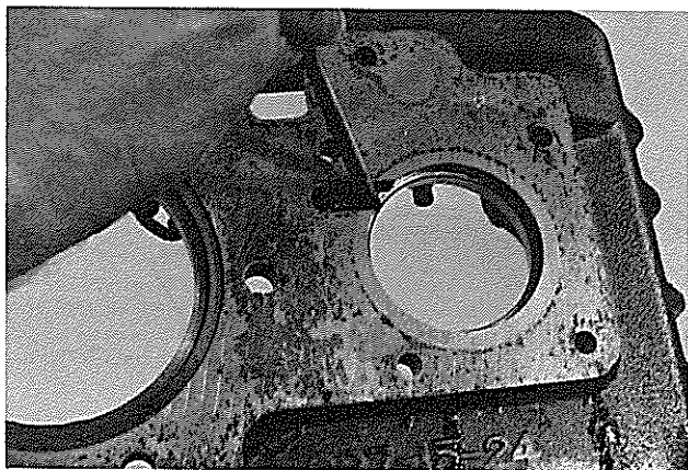
15. Tap bearing cups from rear case.
