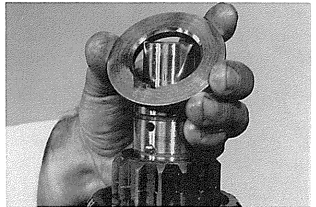
12. Assemble locking pin and lower bronze thrust washer with the flat side up.
