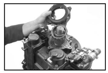
10.Remove the rear bearing retainer and speedometer gear
