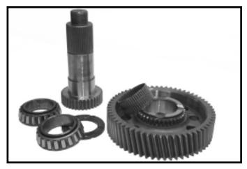
22.Using a press, remove inner output bearing and low range gear from output shaft
