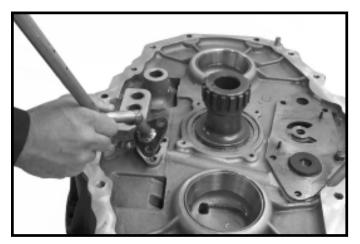
3.Install OPTI-LUBE spray distribution tube and torque bolts to 38-42 ft.lbs.
