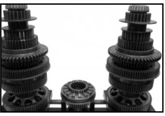
13.Remove  $5^{th}$  gear and  $4^{th}/5^{th}$  clutch collar and  $4^{th}$  gear
