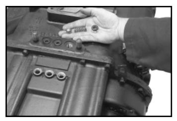
15.Install the detent balls, springs and torque plugs to  $25-41\,\mathrm{ft}$ . lbs.
