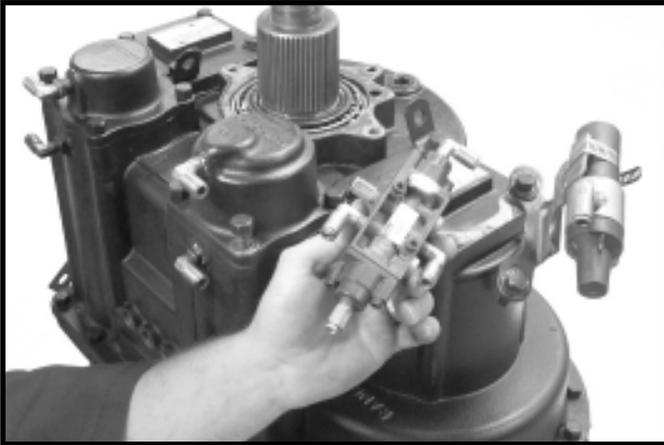
11. Remove air filter regulator, bracket, range and splitter valves
