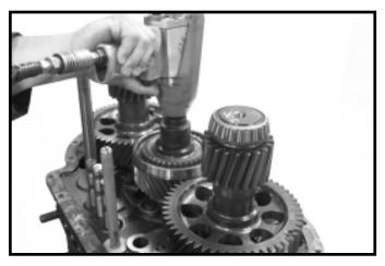
18.Use an 1 1/2" socket to remove the synchronizer ring
