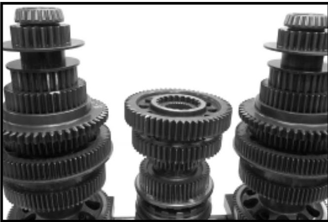
11.Remove 1<sup>st</sup> gear and 1<sup>st</sup>/ reverse clutch collar
