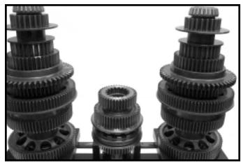
6.Install  $2^{nd}$  gear,  $2^{nd}$  /  $3^{rd}$  gear clutch collar and  $3^{rd}$  gear
