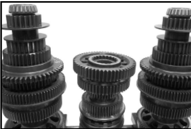
7. Install 1<sup>st</sup> gear and 1<sup>st</sup> / reverse clutch collar
