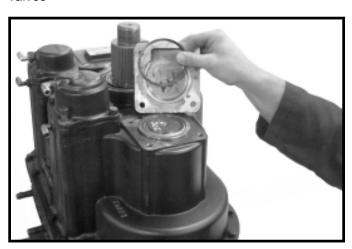
12. Remove the rear countershaft bearing retainer shims
