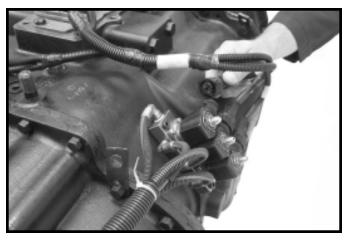
18.Install wiring harness and attach to shift solenoids
