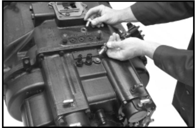
4.Remove three gear position switches and back-up light switch
