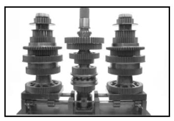
9.Install tapered bearing, thrust washer and reverse gear
