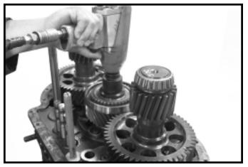
2.Install high range synchronizer race, clutch gear, washer and bolt. Torque bolt to 380 – 400 ft. lbs.
