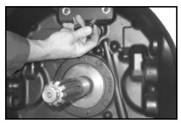
8.Remove two clutch housing bolts from the inside of the bell housing before placing the transmission on end
