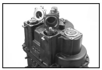
7.Install range and splitter piston housings and bolts torque to 29 – 45 ft.lbs.
