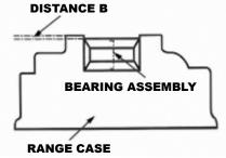
Next, measure from the face of the range case to the end of the pilot (B). Subtract the two figures and shim accordingly. You can be within four thousandths of an inch, so select the shims that will give you the amount closest to what is required
