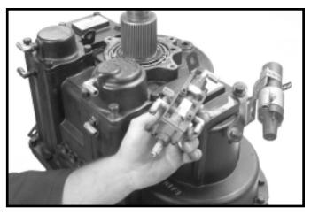
10.Install air filter regulator, bracket range and splitter valves
