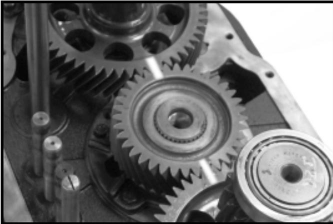
1. Install range countershafts and high range gear making sure to align the timing marks
