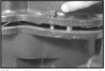
15.Remove all the range case bolts, then thread two of the case bolts into the threaded holes provide and draw tight to split the range case from the main case
