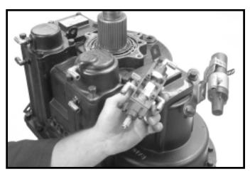
11.Remove air filter regulator, bracket, range and splitter valves
