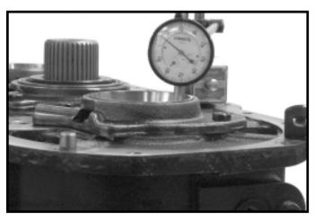
17.Measure front countershaft end play by prying the countershaft up and down with a large screwdriver thru the PTO opening. (End play should be .001 – .008) Adjust end play by adding, or subtracting shims under the rear countershaft
