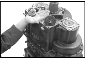
6.Install range and splitter pistons and retaining nuts and torque to 29 – 45 ft.lbs.
