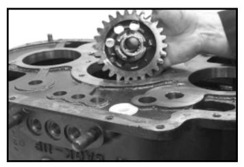
11.Install the reverse idler gear, caged needle bearing and spacer
