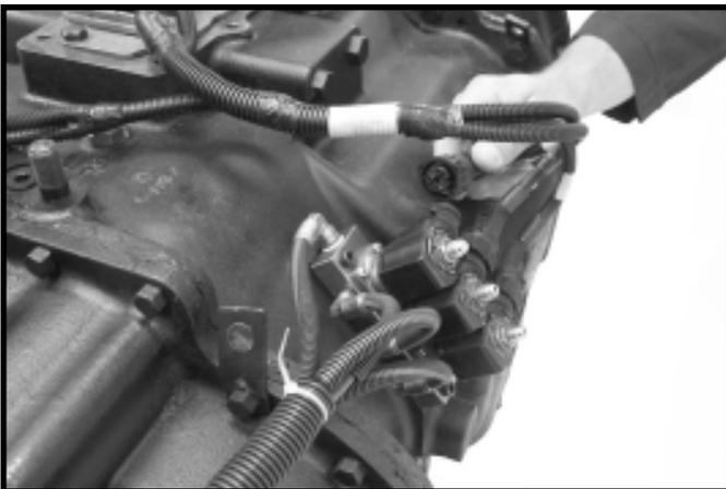
2.Remove wiring harness from shift solenoids
