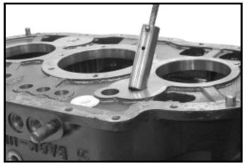
3.Use a slide hammer with a 3/8" 16 thread adapter to remove the reverse idler shaft
