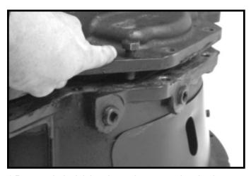
1.Remove bolts joining the main case to the clutch housing. After removing all the bolts, thread two of the case bolts into the threaded holes provided in the main case and draw tight to split the main case from the clutch housing
