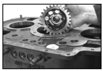
4.Remove the reverse idler gear, caged needle bearing and spacer
