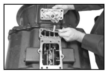
7. Remove the overdrive shift fork reversing mechanism
