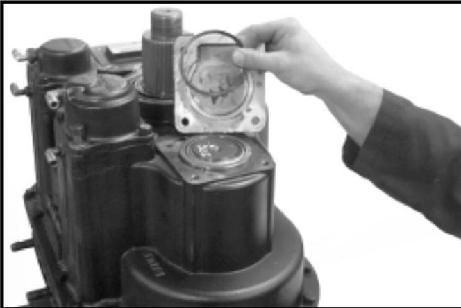
12. Remove the rear countershaft bearing retainer shims
