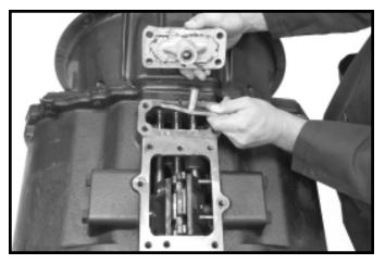
13.Install the overdrive shift fork reversing mechanism
