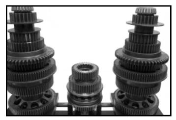
12.Remove  $2^{\text{nd}}$  gear,  $2^{\text{nd}}/3^{\text{rd}}$  gear clutch collar and  $3^{\text{rd}}$  gear
