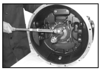
2.Apply Loctite 515 to front bearing retainer and install. Torque bolts to  $38-42\ \mathrm{ft}$ . Ibs.
