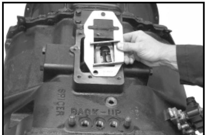
6.Remove interlock retaining bolts, plate and interlock
