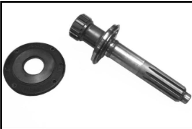
17.To remove the input shaft and bearing cap, remove the four cap retaining bolts. Pull the shaft from the housing. It may be helpful to place 2 bolts in the threaded bearing cap holes. Tightening the bolts will draw the bearing cap from the housing. Tap the input shaft out of the bearing cap. To disassemble the input shaft assembly, remove the snap ring, press the bearing off the shaft
