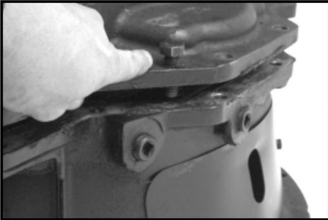
1. Remove bolts joining the main case to the clutch housing. After removing all the bolts, thread two of the case bolts into the threaded holes provided in the main case and draw tight to split the main case from the clutch housing
