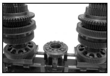
14. Remove splitter clutch gear and shift collar
