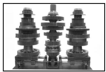
8.Remove the lifting tool and slide the countershafts apart
