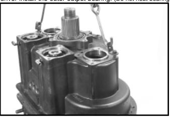
5. Using a chain hoist lift the range case and attach to main case with case bolts, torque to 38-42 ft. lbs.
