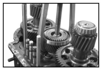
19. Using a puller, remove the high-range gear and synchronizer
