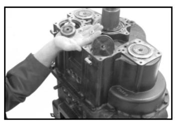
14.Remove the range and splitter piston retaining nuts and pistons
