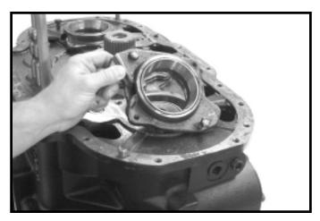
23. Remove rear countershaft bearing retainers
