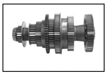
1. This view of the countershaft shows the direction of the gears. The gears are secured with three keys, with the exception of reverse. This gear is part of the shaft, All gears can be pressed off one at a time towards the front of the countershaft
