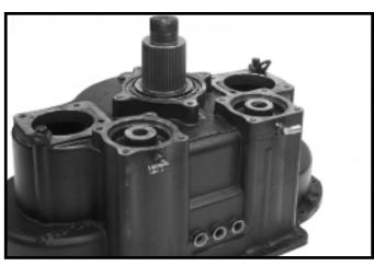
4.Install output shaft assembly into range case assembly. Install inner output bearing spacer and using the proper driver install the outer output bearing. (Do not heat bearing)
