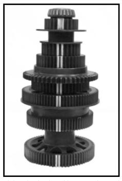
2.If a straight edge is placed between the teeth (painted here to show the timing marks) every gear on the countershaft will be in line
