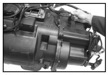
19. Attach wiring harness to gear position switches
