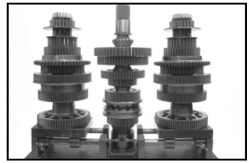
9.Remove tapered bearing, thrust washer and reverse gear
