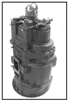
11.Install the speedometer gear and end yoke, or flange. Torque to 550 – 600 ft. lbs.
