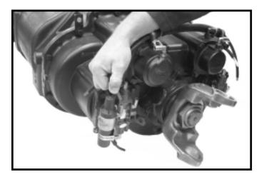
3.Remove all air lines and necessary fittings (note: it is not necessary to mark lines for reassembly since a schematic is provided on page 7)
