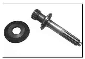
17.To remove the input shaft and bearing cap, remove the four cap retaining bolts. Pull the shaft from the housing. It may be helpful to place 2 bolts in the threaded bearing cap holes. Tightening the bolts will draw the bearing cap from the housing. Tap the input shaft out of the bearing cap. To disassemble the input shaft assembly, remove the snap ring, press the bearing off the shaft
