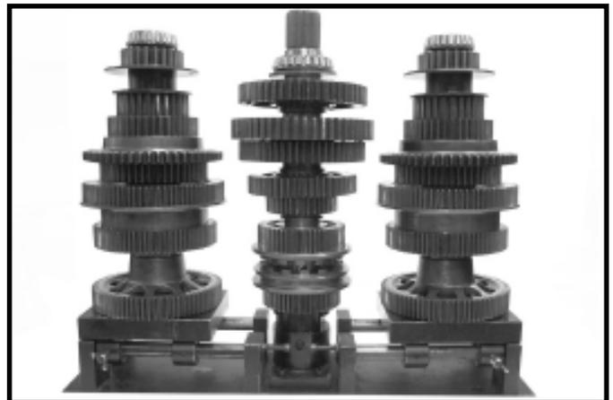
8. Remove the lifting tool and slide the countershafts apart
