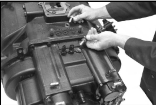
16. Install the three gear position switches and back-up light switch. Torque to 25 – 41 ft. lbs.
