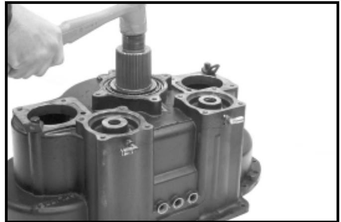
21.Using a plastic mallet, remove output shaft from range case assembly **REPLACE HAMMER**
