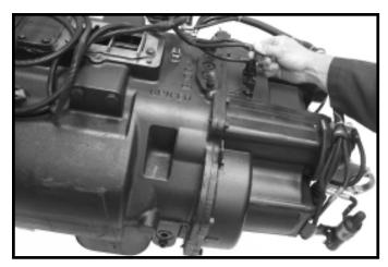
1.Remove wiring harness from gear position switches
