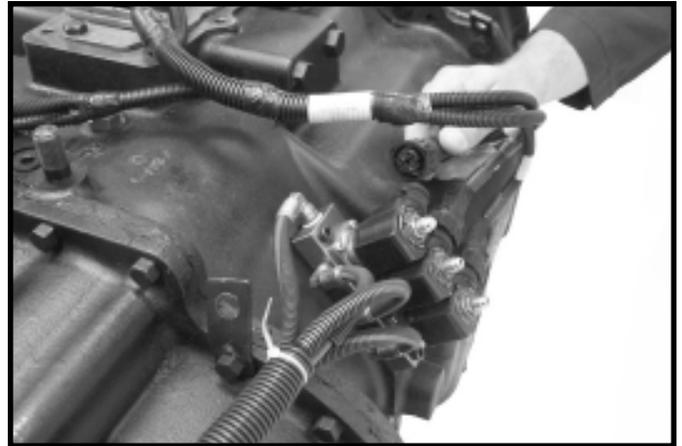
18. Install wiring harness and attach to shift solenoids
