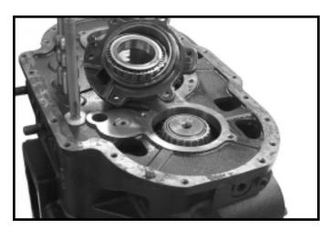
24.Remove rear main shaft bearing retainers
