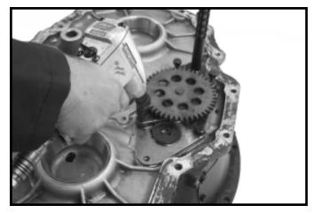
4.Install OPTI-LUBE pump with 3 bolts and torque to 38 – 42 ft.lbs.
