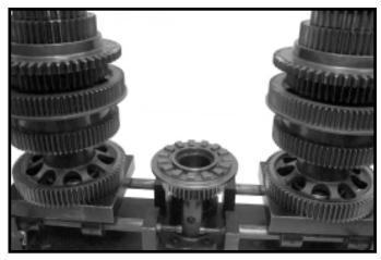
5.Install countershafts, splitter clutch gear and shift collar into "countershaft / mainshaft" assembly fixture. Continue building mainshaft assembly by placing  $5^{\text{th}}$  gear and  $4^{\text{th}}$  /  $5^{\text{th}}$  clutch collar and  $4^{\text{th}}$  gear into fixture
