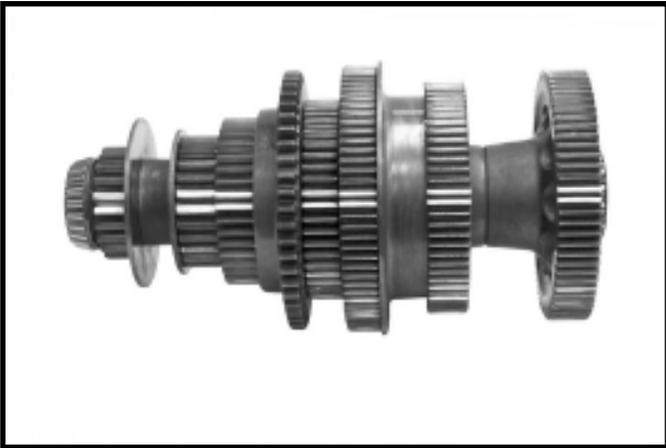
1. This view of the countershaft shows the direction of the gears. The gears are secured with three keys, with the exception of reverse. This gear is part of the shaft, All gears can be pressed off one at a time towards the front of the countershaft
