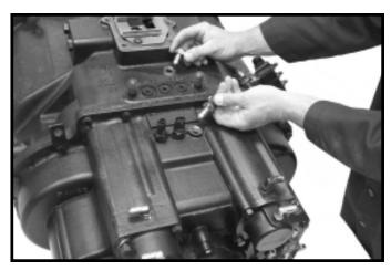
4.Remove three gear position switches and back-up light switch
