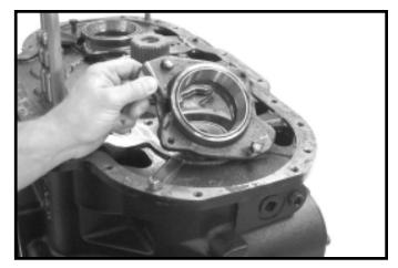
16.Install rear countershaft bearing retainers and torque bolts to  $38-42 \, \text{ft.lbs}$ .
