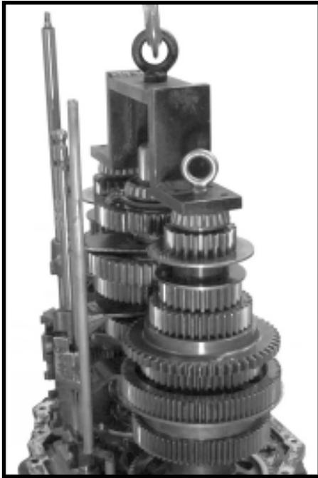
! 5. Install an "A-frame lifting fixture" and use a chain hoist to remove the shaft assembly
