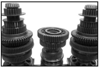
7.Install 1st gear and 1st / reverse clutch collar
