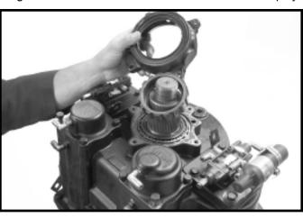
9.Install rear bearing retainer and shims (refer to diagram). Install speedometer gear
