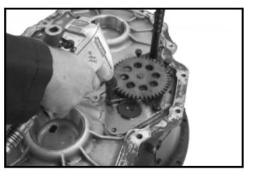
15.Remove 3 retaining bolts from OPTI-LUBE pump
