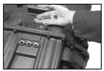
5. Remove detent balls and springs
