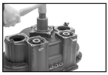
21.Using a plastic mallet, remove output shaft from range case assembly REPLACE HAMMER
