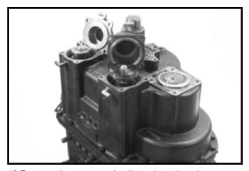
13. Remove the range and splitter piston housings
