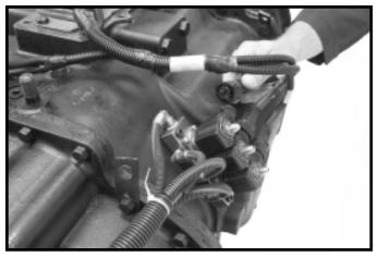
2. Remove wiring harness from shift solenoids
