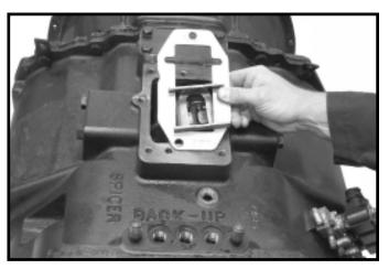
6.Remove interlock retaining bolts, plate and interlock
