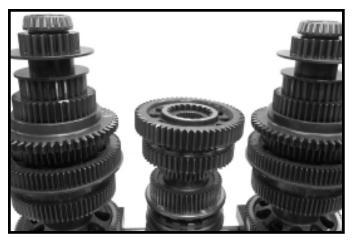
11.Remove 1st gear and 1st/ reverse clutch collar
