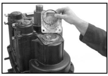
8.Install range countershaft rear bearing retainers and shims range countershafts must have a .003 – .007 of endplay
