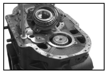
15.Install rear mainshaft bearing retainer and torque bolts to 38 - 42 ft.lbs.
