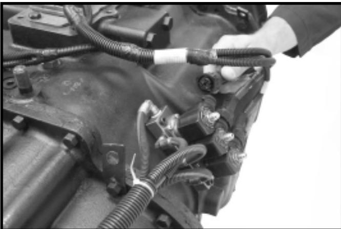
2.Remove wiring harness from shift solenoids
