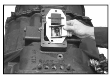
14.Install the interlock, plate and retaining bolts. Torque to 52 - 92 ft. lbs.
