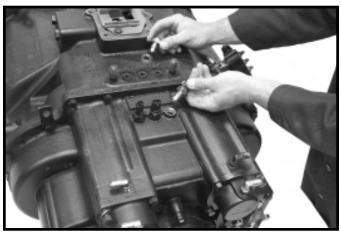
16.Install the three gear position switches and back-up light switch. Torque to 25 – 41 ft. lbs.
