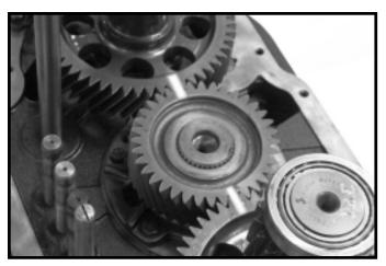
1.Install range countershafts and high range gear making sure to align the timing marks
