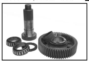
3.Install cage needle bearing, low range gear, and thrust washer. Install inner output bearing to the output shaft. (Do not heat bearing)
