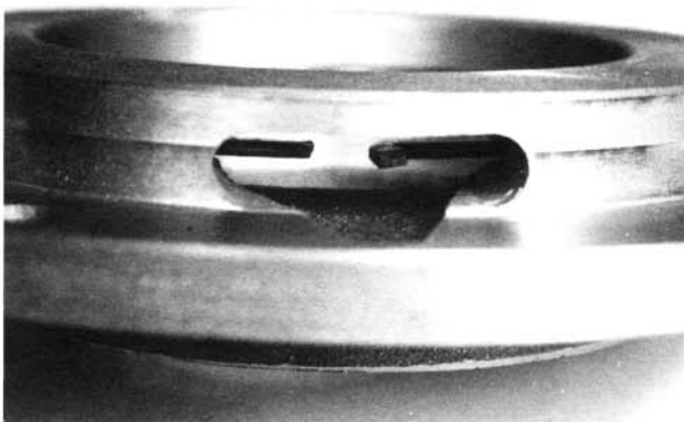
3. When reassembling, first install the snap ring into the input bearing cap.
