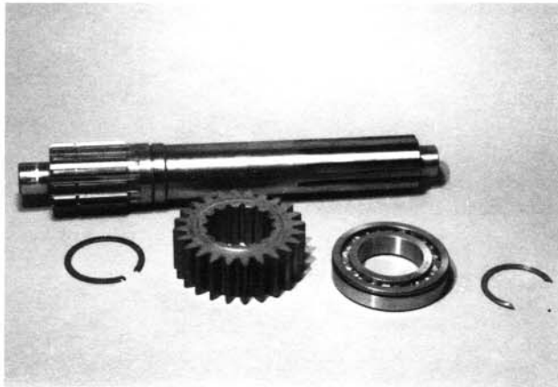
2. This view shows the input subassembly when disassembled.
