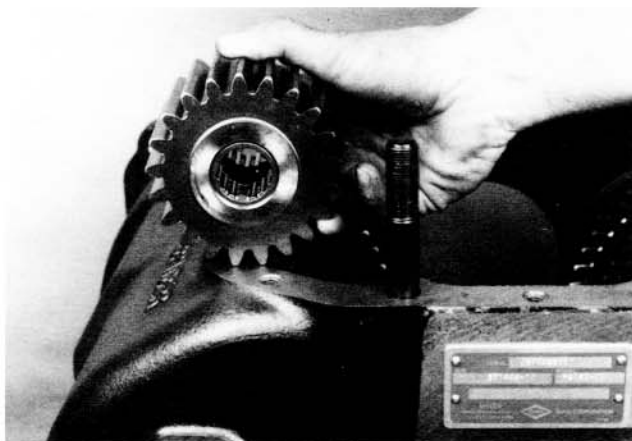
23. Remove the upper reverse idler gear.
