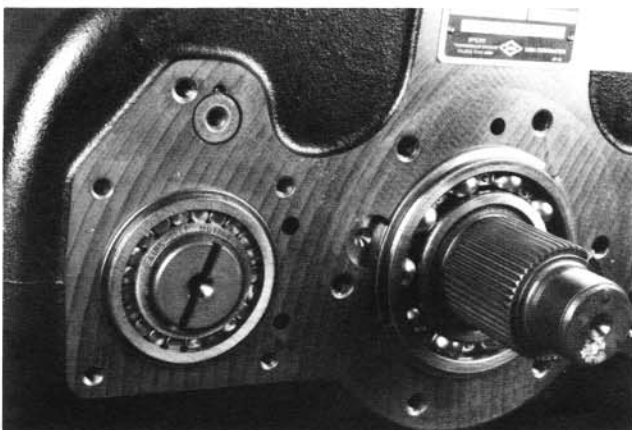
21. Install the upper reverse idler shaft. Note: It is difficult to align the gear with the case hole unless the input shaft is in the unit. It is also necessary to lift up on the mainshaft reverse gear to obtain proper alignment.
