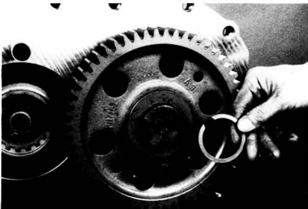
9. Remove the snap rings from the countershafts. Always wear safety glasses to protect your eyes when removing or installing snap rings or bearings.
