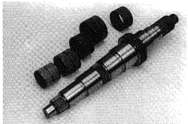
10. The mainshaft uses caged needle bearings under all gears.
