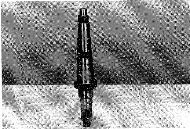
13. Begin reassembly by placing the mainshaft in an upright position. Also, coat all bearings with Moly #2 lubricant at this time.
