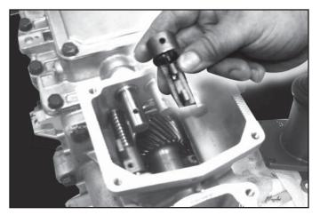
10. Install the new 3/4 shift lug supplied in the kit. Make sure that the opening on shifting lug is up.
