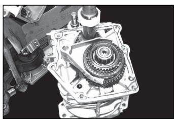
Clean all mating surfaces thoroughly. Check condition of all six O-rings on shift rails prior to attaching the rear extension. Replace if cut or missing. Apply anaerobic sealer to mating surface of the main case and attach the rear extension assembly. Torque the six bolts to 42-50 ft-lb.
