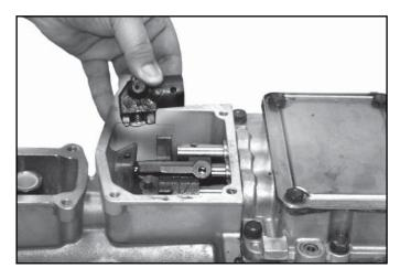
Using a punch, remove the roll pins from the three forward shift lugs. Slide the two (2) outside shift lugs towards the rear and remove from unit. DO NOT CLEAN the factory applied grease from the lugs.
