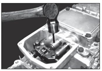
11. Install the two (2) outside shift lugs with the openings to the center. Secure all three (3) shift lugs with roll pins.
