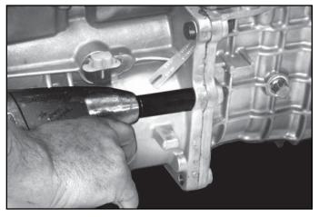
4. Remove the six (6) rear extension assembly to main case bolts.
