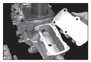
13. Apply RTV sealant to rear shift cover opening. Install rear cover plate supplied in kit. Re-use the original shifter bolts to secure plate. Torque to 18-22 lb./ft.
