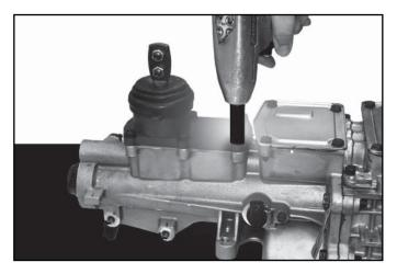
Shift unit into neutral position. Remove six (6) shift tower housing bolts from rear of extension housing. NOTE: Do not discard bolts as they will be needed during reassembly. Remove shifter housing and discard.
