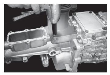
12. Clean mating surfaces thoroughly. Apply RTV sealant to mating surface of the shift tower assembly and rear extension. Install new shift tower assembly. Torque the four (4) new bolts included in kit to 18-22 ft-lb. Install shift boot.
