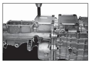
Remove the four (4) bolts and star washers from the middle inspection cover. Remove inspection cover. NOTE: The old bolts are not required for re-assembly. Four new longer bolts are supplied in kit.
