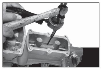
6. Make sure the rear shift rail is in neutral position. Using a punch, remove the roll pin in the double shift lever socket. The roll pin will fall through the drain hole and will need to be removed after the extension housing is separated from the main case.
